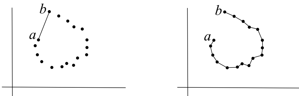
Figure 1.12: Illustration of how MDS and Isomap would calculate the distance between points a and b . Figure on the left shows MDS as taking the Euclidean distance between points. Isomap on the right takes the geodesic distance between points.
