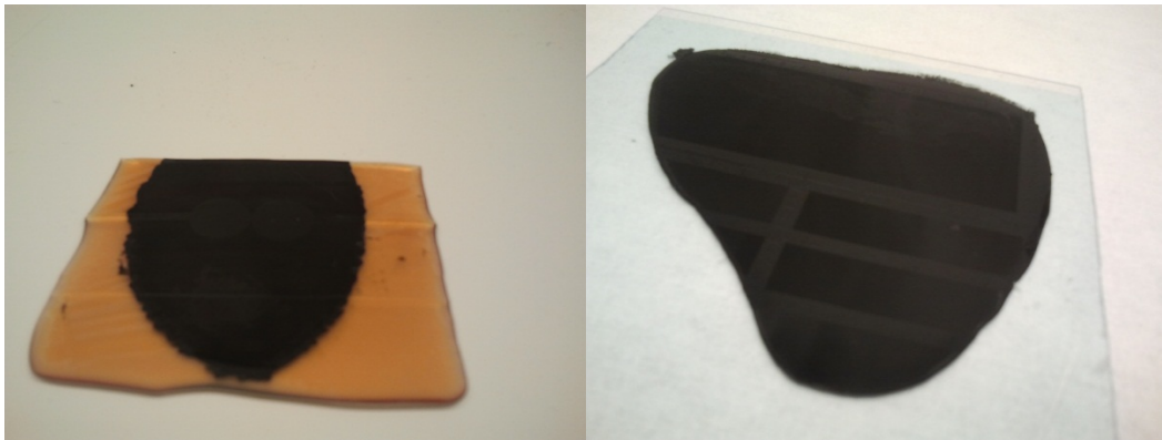
Figure 3.9: Adhesives made out of composite materials. Picture on the left has the composite adhesive portion embedded in plain polyurethane. Picture on the right shows a composite adhesive sample attached to a rigid backing of acrylic.
