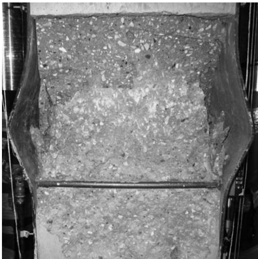
Figure 6-12 Crushed Concrete and NW and SW Flange Buckles in Zone 3 on the West Face of H5 (after test)
