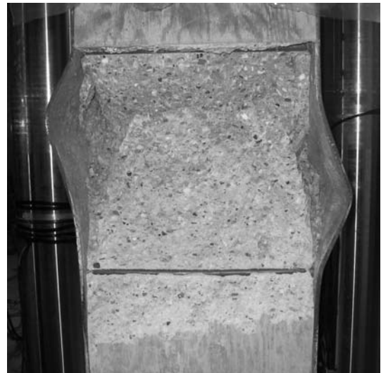
Figure 6-5 Crushed Concrete and NE and SE Flange Buckles in Zone 3 on the East Face of H2 (after test)
