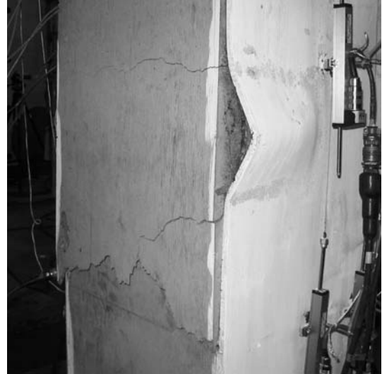
Figure 6-11 Crushed Concrete and NE Flange Buckle in Zone 2 on the East Face of H4 (after test) – SE Flange Buckle in Zone 2 not shown
