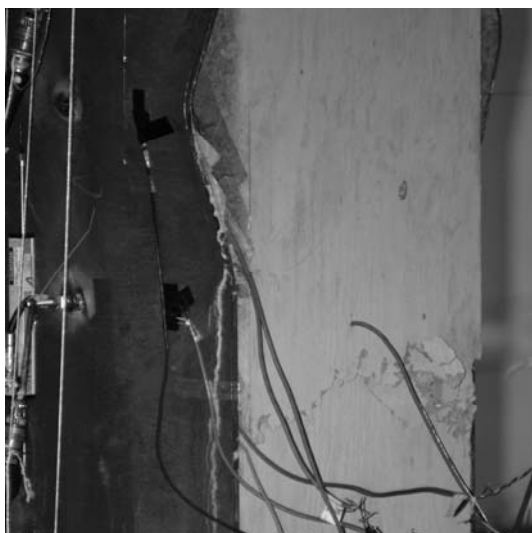
Figure 6-16 Crushed Concrete and NW and SW Flange Buckles in Zone 2 on the West Face of H7 (after test)
