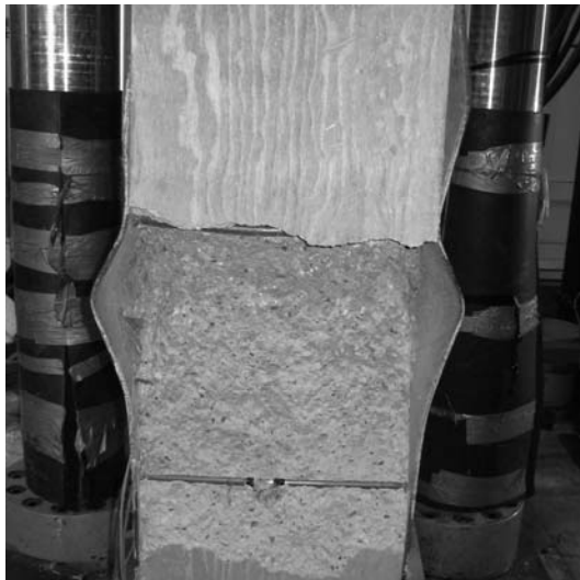
Figure 6-4 Crushed Concrete and NW and SW Flange Buckles in Zone 2 and a Second Buckle of the SW Flange in Zone 3 on the West Face of H2 (after test)
