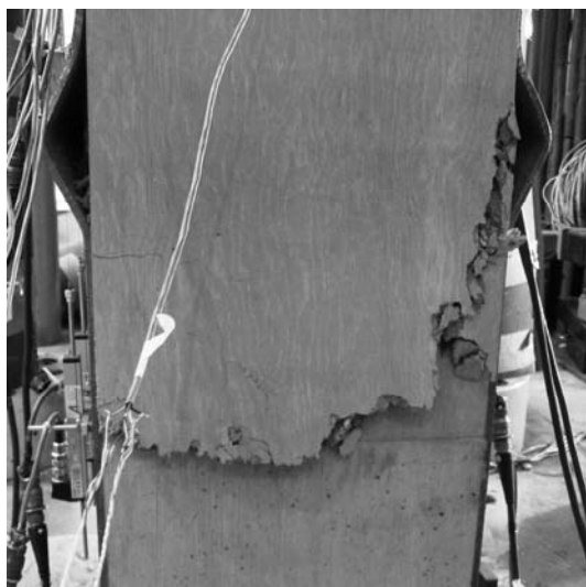
Figure 6-14 Crushed Concrete and NW and SW Flange Buckles in Zone 2 on the West Face of H6 (after test)
