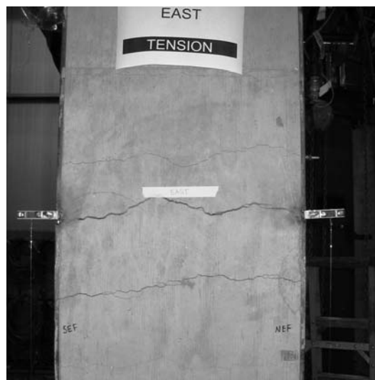
Figure 7-7 Tension Crack Pattern on the East Face of H10 (after test)
