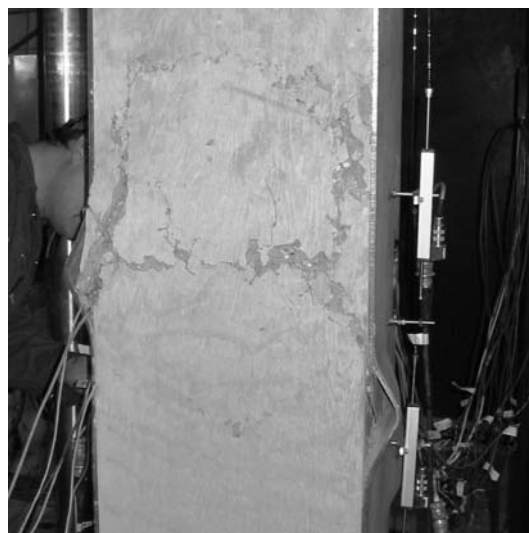
Figure 6-15 Crushed Concrete and SE Flange Buckle in Zone 4 and NE Flange Buckle in Zone 3 on the East Face of H6 (after test)
