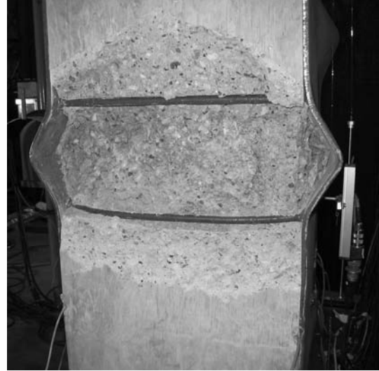
Figure 6-3 Crushed Concrete and NE and SE Flange Buckles in Zone 5 on the East Face of H1 (after test)
