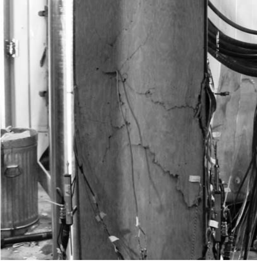
Figure 7-2 Crushed Concrete and SW Flange Buckle in Zone 3 on the West Face of H8 (after test)
