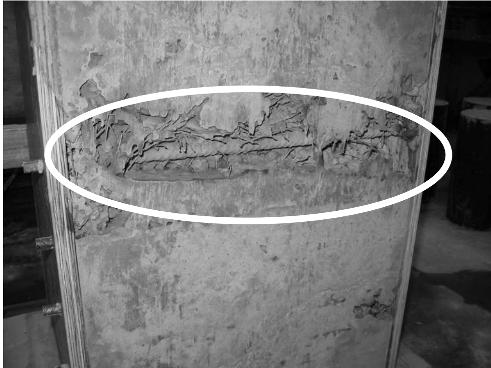
Figure 3-3 Void in Concrete (within ellipse) at Link Created by Bridging of 60 mm Steel Fibres (École Polytechnique)
