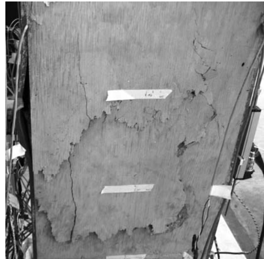
Figure 7-5 Crushed Concrete and SE Flange Buckle in Zone 2 on the East Face of H9 (after test)
