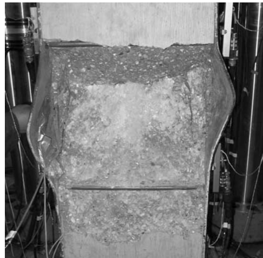
Figure 6-13 Crushed Concrete and NE and SE Flange Buckles in Zone 2 on the East Face of H5 (after test)
