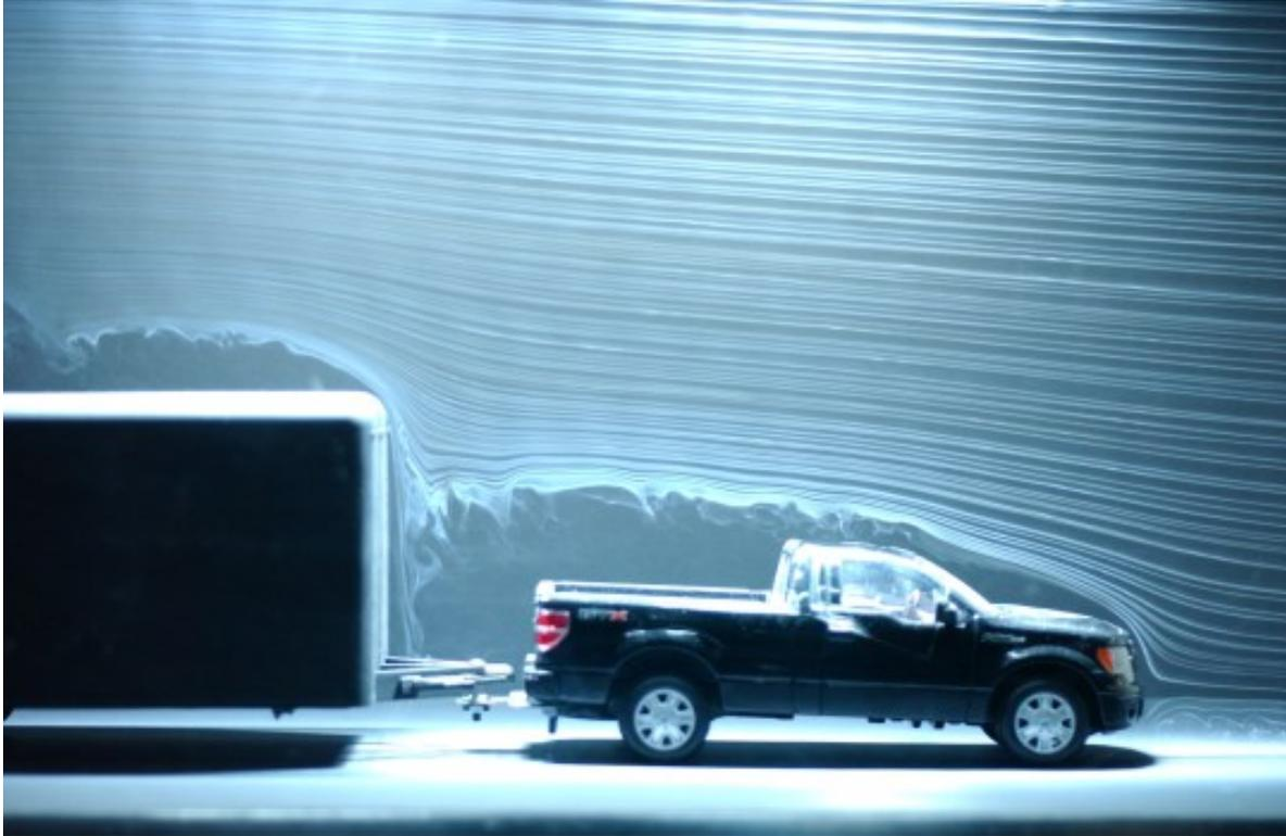
**Figure 34: Hood separation,  $Re = 15,800$ . Flow in right to left direction, contrary to convention.**
