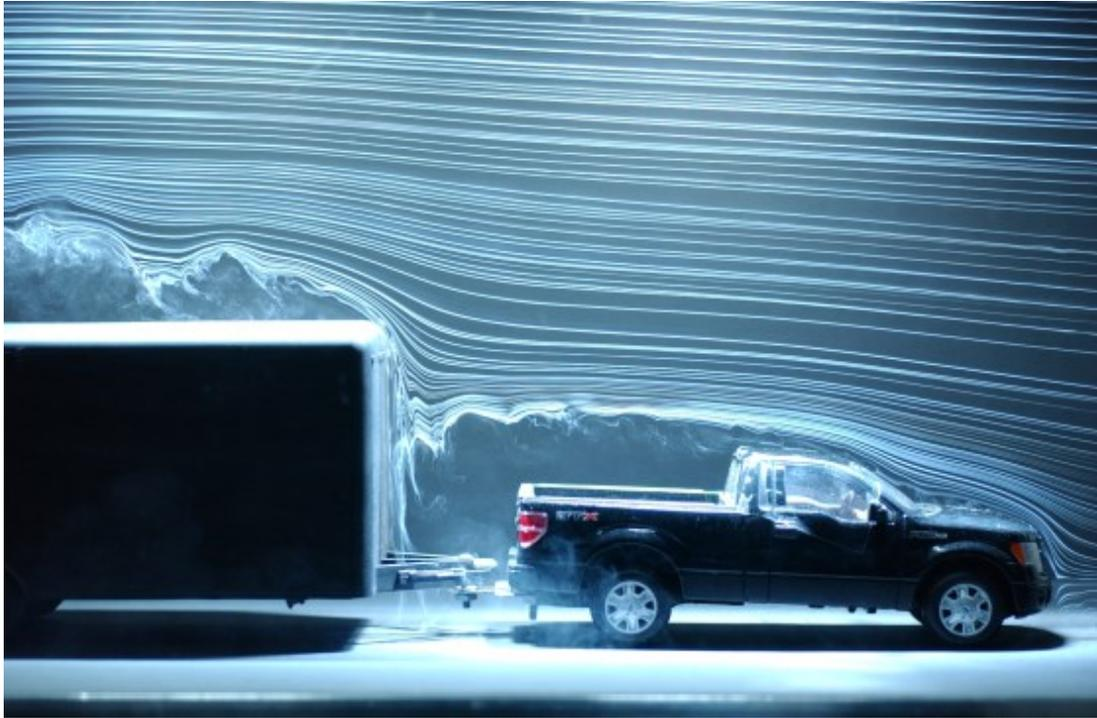
**Figure 35: Hood separation reduced,  $Re = 44,400$ .**
