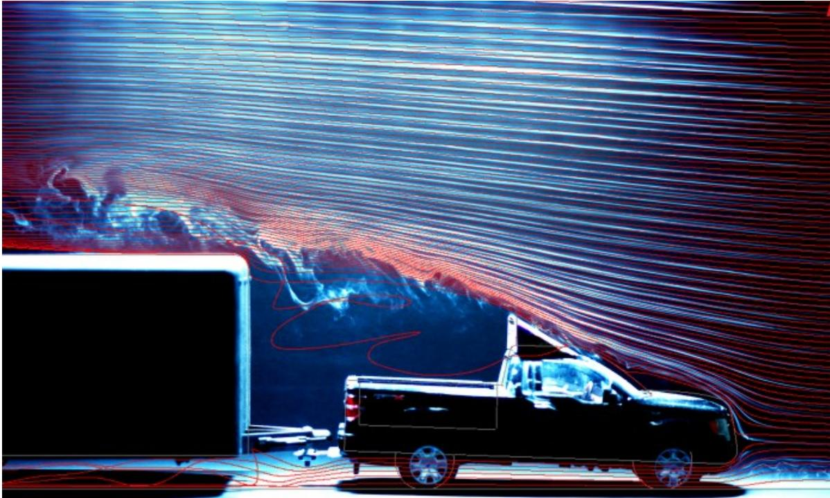
Figure 42: Streamline, streakline overlay with deflector. Flow in right to left direction. Re = 14,900.
