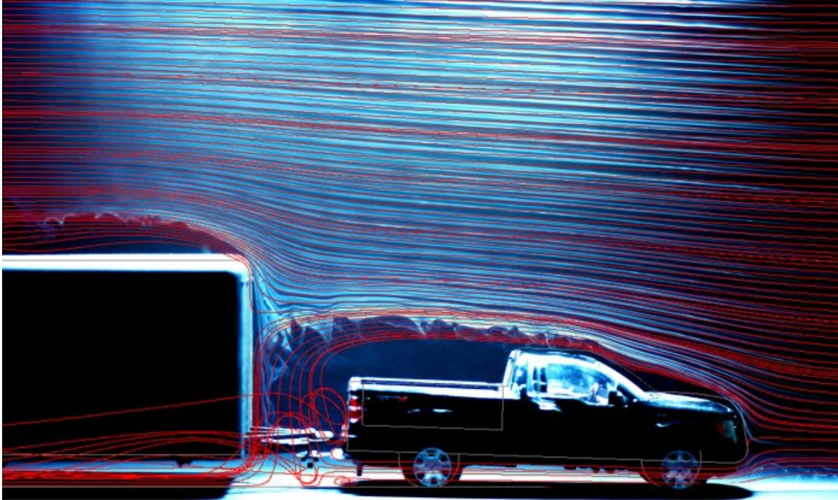
Figure 41: Streamline, streakline overlay with no deflector. Flow in right to left direction.
