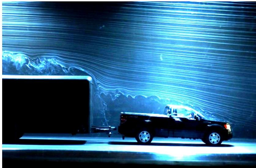
**Figure 10: Ford F-150 and cargo trailer with deflector.  $Re = 13,700$**
