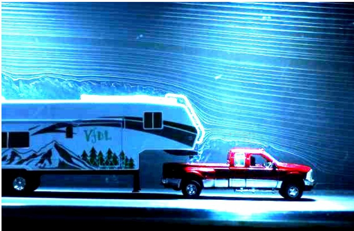
**Figure 5: Ford F-350 and fifth wheel trailer,  $Re = 13,700$ , flow is from right to left.**
