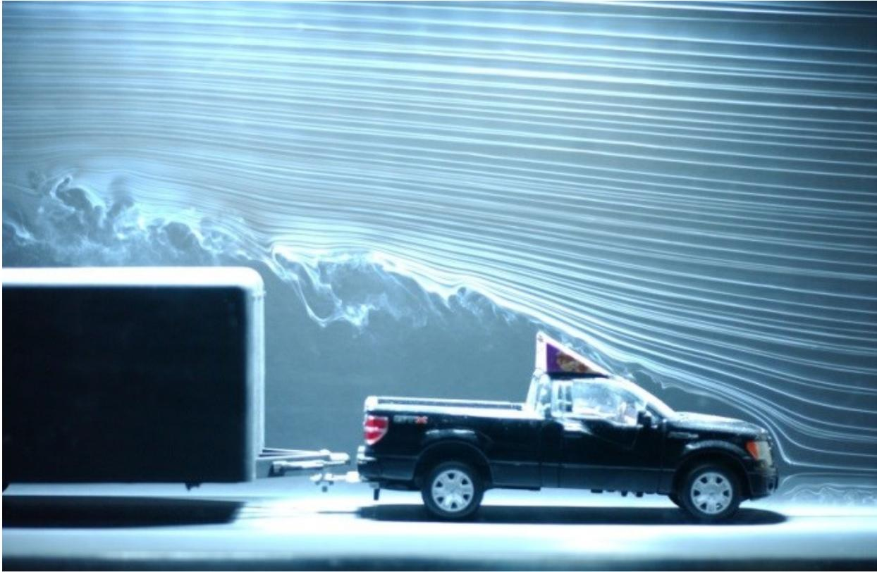
**Figure 40: Experimental streaklines of mean stream flow over model with deflector.**
