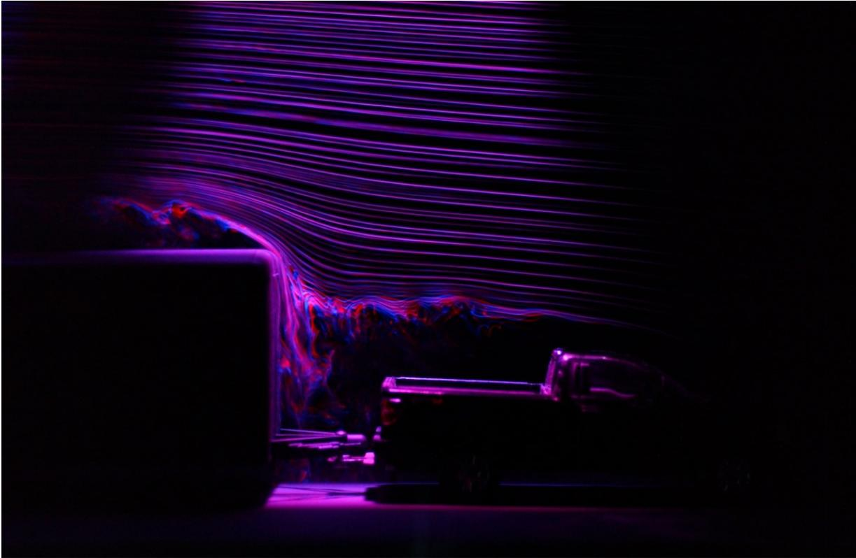
**Figure 18: ICV Photograph showing red and then delayed blue strobe exposures of smoke streaklines.**
