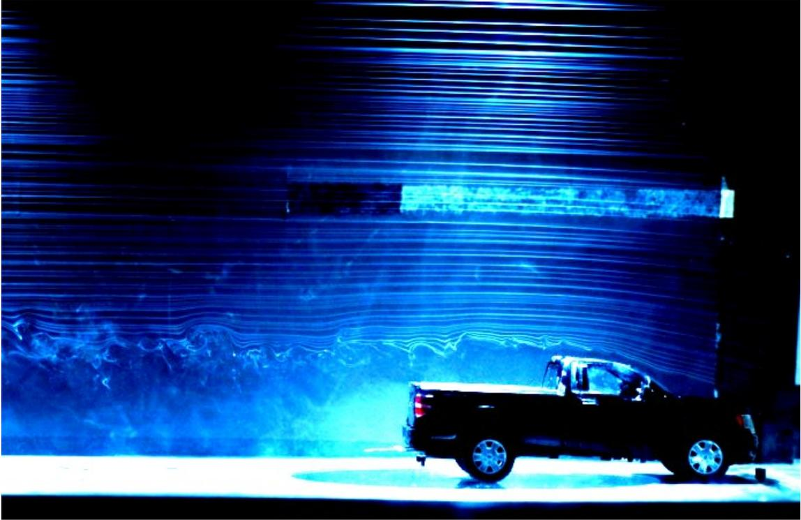
**Figure 13: Only truck model present in wind-tunnel.**
