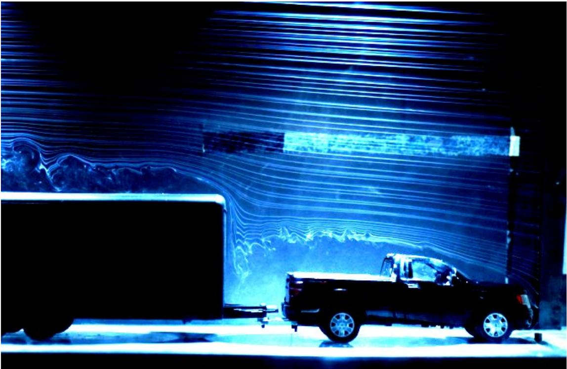
**Figure 14: Truck and trailer present in wind-tunnel.**
