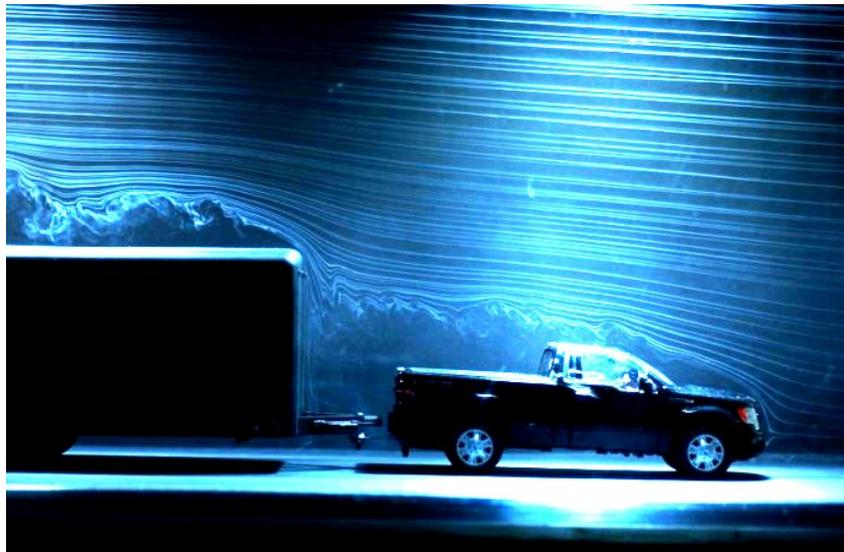
**Figure 9: Ford F-150 and cargo trailer without deflector.  $Re = 13,700$ .**
