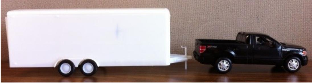
**Figure 2: Wind-tunnel model of Light-Vehicle Trailer System studied here.**
