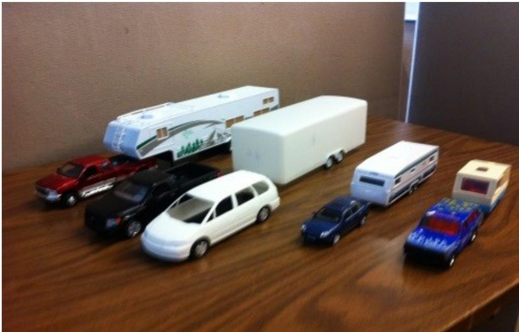
**Figure 1: Modern Light Vehicle-Trailer Systems. From left to right: a Fifth-Wheel, a truck or van with a Cargo Trailer, an SUV with Travel Trailer, a Jeep type vehicle with Classic Travel Trailer. Photo courtesy of Bradley Myers.**
