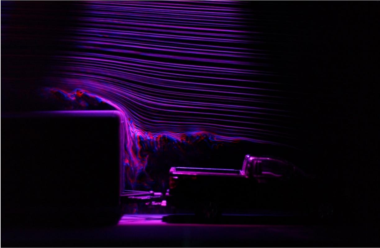
**Figure 18: ICV Photograph showing red and then delayed blue strobe exposures of smoke streaklines.**
