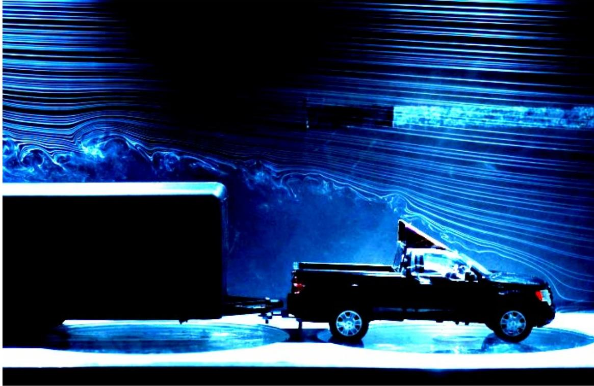
**Figure 15: F-150 and cargo trailer with deflector.**
