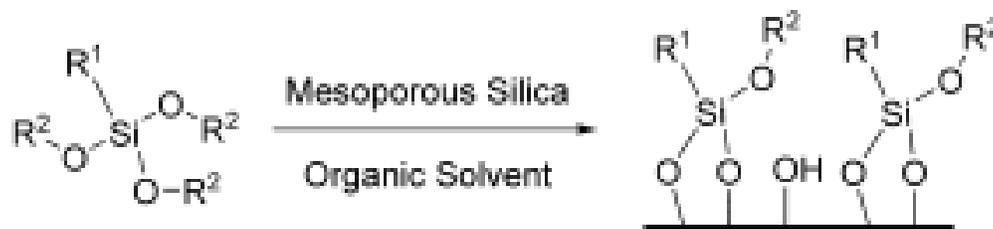
Figure 2-1. Scheme for reaction of silane with silica
