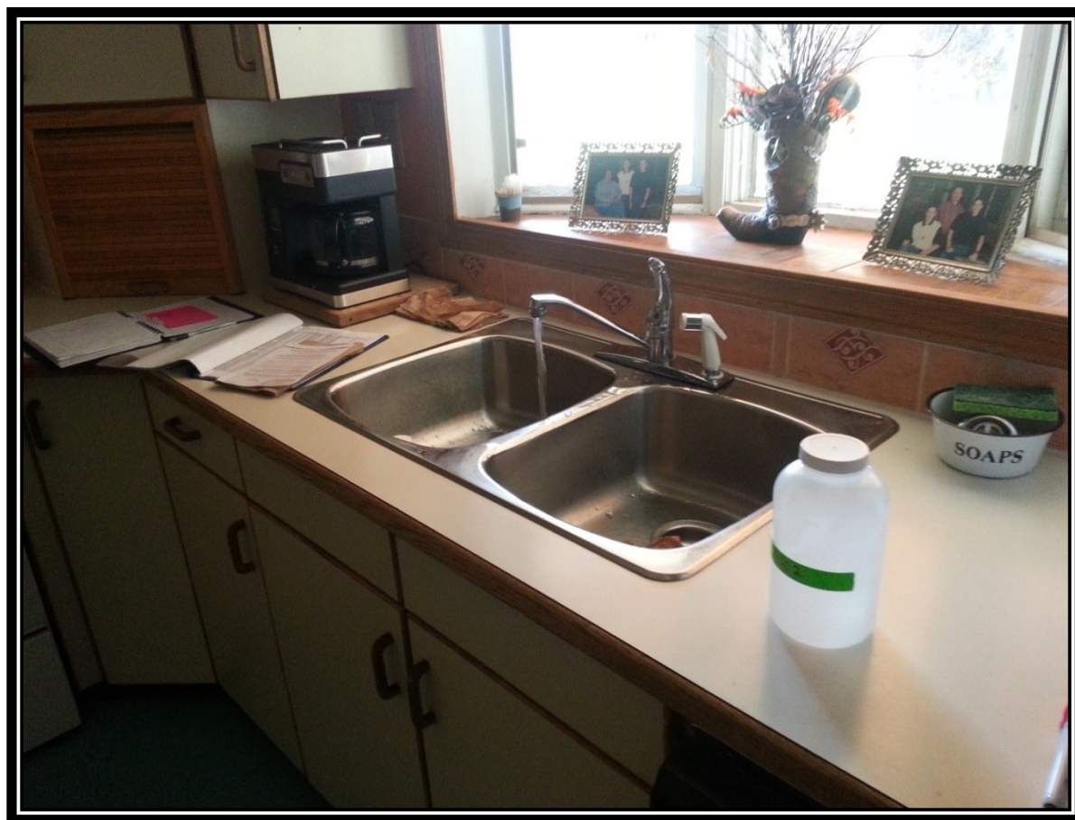
FIGURE 4-1: WATER SAMPLES WERE COLLECTED IN CLEAN PLASTIC BOTTLES FROM KITCHEN TAPS AFTER DISINFECTION WITH CHLORINE SOLUTION AND RUNNING THE WATER FOR THREE MINUTES.
