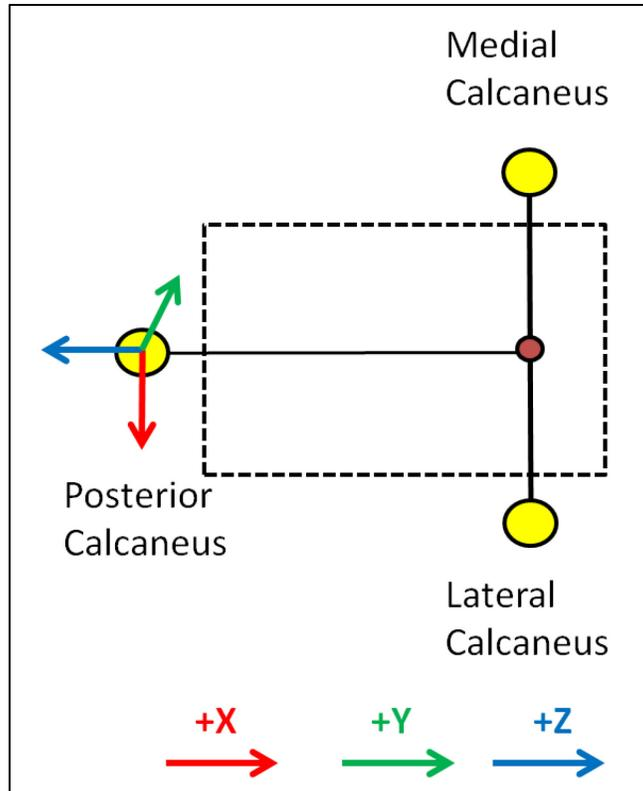
**Figure 2-3: Diagram showing method for modeling the calcaneus from motion analysis data. Yellow circles identify retro-reflective markers, red circles identify center points. This is a top down view of the calcaneus.**
