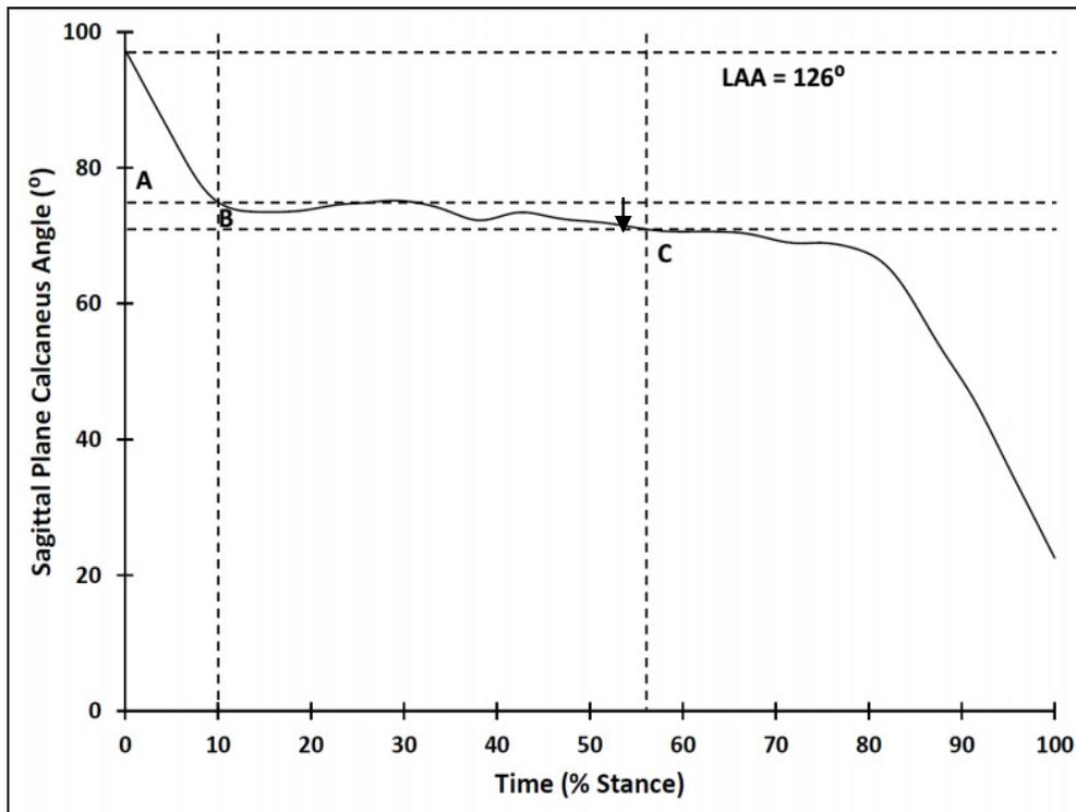
Figure 2-10: Calcaneal plantar flexion during stance for the foot with the lowest LAA (126°). Time point A is heel strike, B is footflat, and C is heel off; midstance is between B and C.
