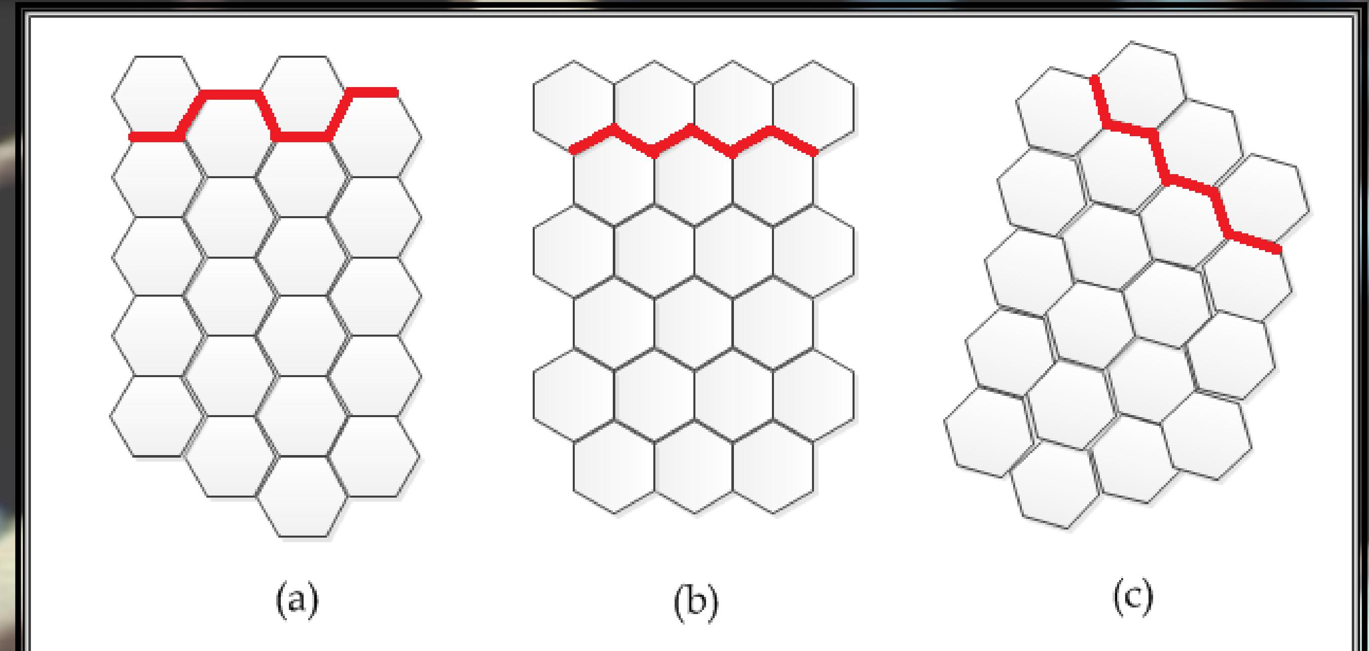
Figure 1) The different structural conformations of single-walled carbon nanotubes walls. The three structures are armchair (a), zigzag (b), and chiral (c). The red lines show the different orientations of the carbon bonds.
