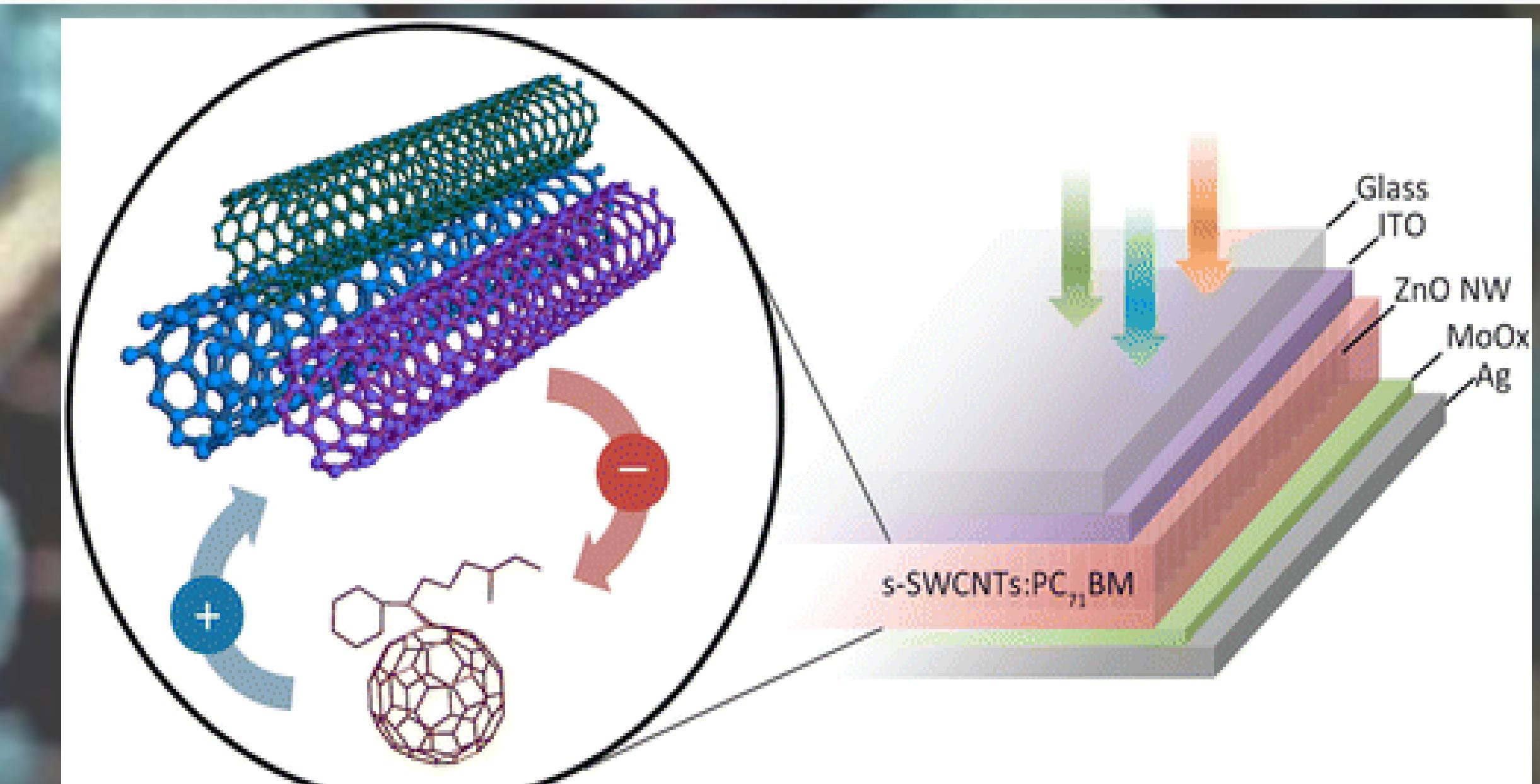
Figure 2) The composition of a photovoltaic cell using multiple forms of carbon nanotubes. The usage of multiple layers allows for greater absorption of energy. Modified from: Gong et al. (2014)
