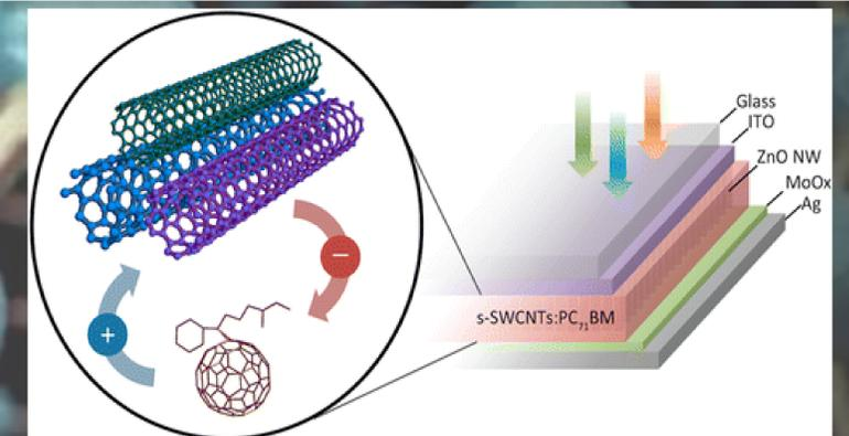
Figure 2) The composition of a photovoltaic cell using multiple forms of carbon nanotubes. The usage of multiple layers allows for greater absorption of energy.
