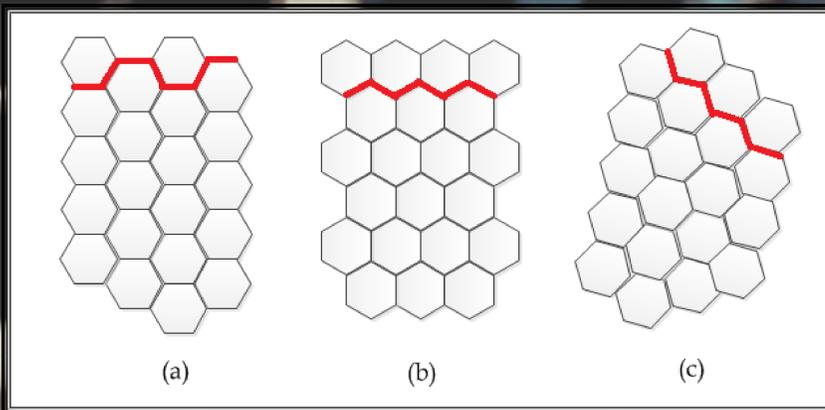
Figure 1) The different structural conformations of single-walled carbon nanotubes walls. The three structures are armchair (a), zigzag (b), and chiral (c). The red lines show the different orientates of the carbon bonds.
