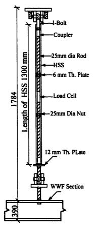
Figure 3.13 Detail of Vertical Link
