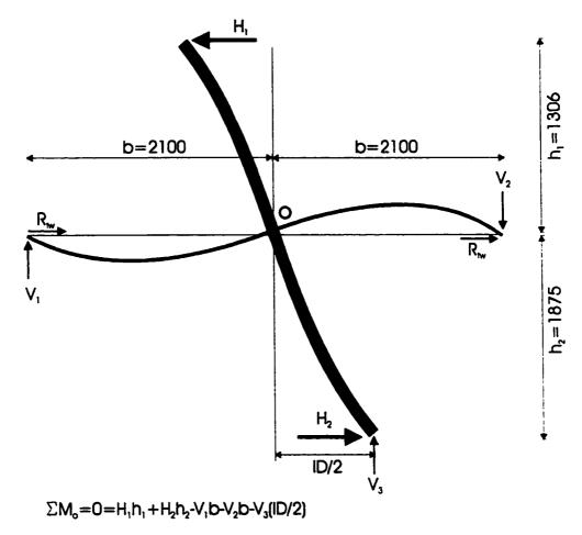
$R_{\mbox{\tiny hw}} = \mbox{Resistance}$  due to friction in Twisting Restraints
