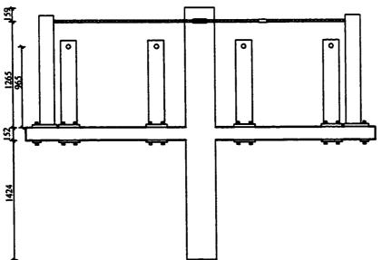
Figure 3.15 Slab Edge Restraining System
