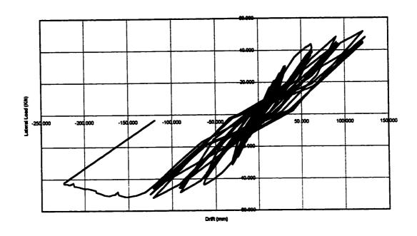
Figure 4.10 Horizontal Load vs. Lateral Drift Steel Fibre Specimen
