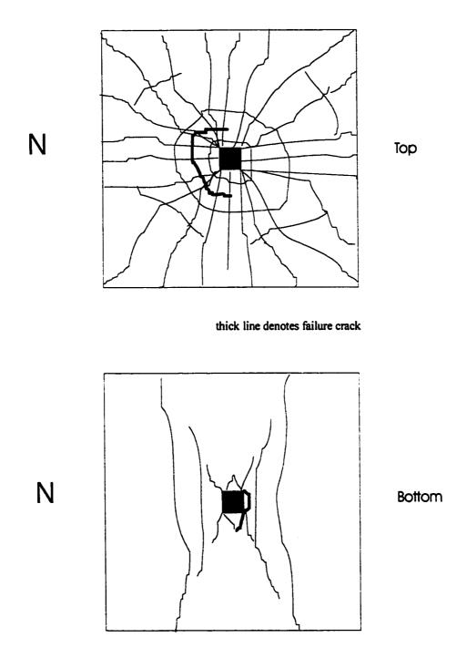
Figure 4.2 Final Crack Pattern of Control Specimen
