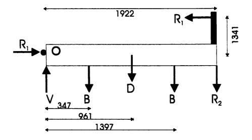
Figure 5.2 Free Body Diagram of Slab Cantilever
