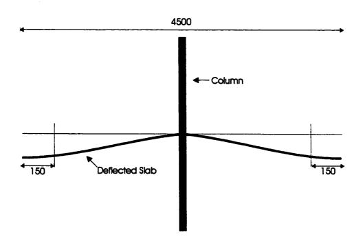
Figure 3.2 Slab Deflection under Gravity Loads
