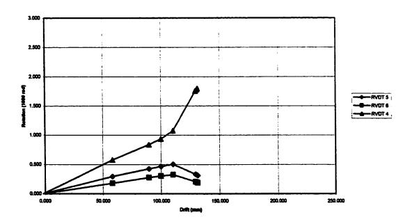
Figure 4.19 Slab Rotation vs. Lateral Drift RVDT 4, 5 & 6 Control Specimen – Failure
