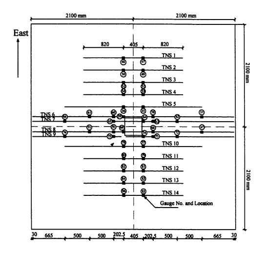
Figure 3.18 Top Mat Strain Gauge Locations (N-S Direction)
