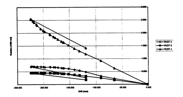
Figure 4.18 Slab Rotation vs. Lateral Drift RVDT 4, 5 & 6 Steel Fibre Specimen – Pushover
