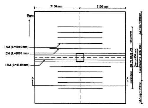
Figure 3.7 Slab Reinforcement - Top Mat (N-S Direction)
