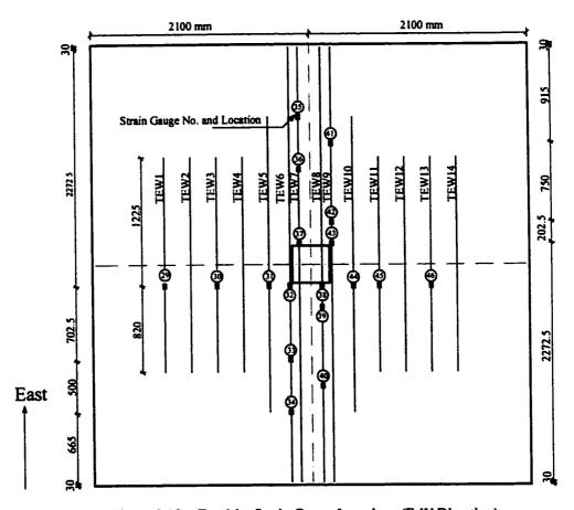
Figure 3.19 Top Mat Strain Gauge Locations (E-W Direction)
