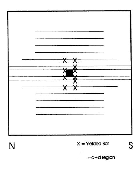
Figure 4.20 Yielded Bar Locations at Failure in Top Mat Steel Fibre Specimen
