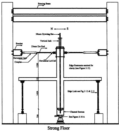
Figure 3.10 Lateral Load Test Frame
