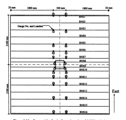
Figure 3.20 Bottom Mat Strain Gauge Locations (N-S Direction)
