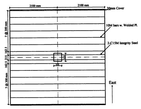
Figure 3.5 Slab Reinforcement - Bottom Mat (N-S Direction)
