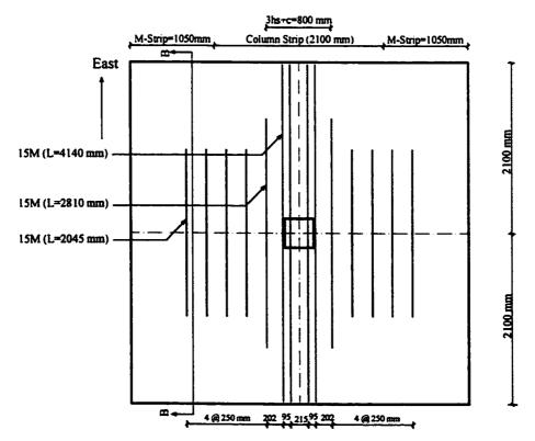
Figure 3.8 Slab Reinforcement - Top Mat (E-W Direction)
