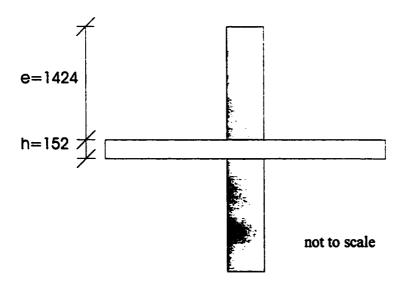
Figure 3.3 Geometry of Specimen (mm)
