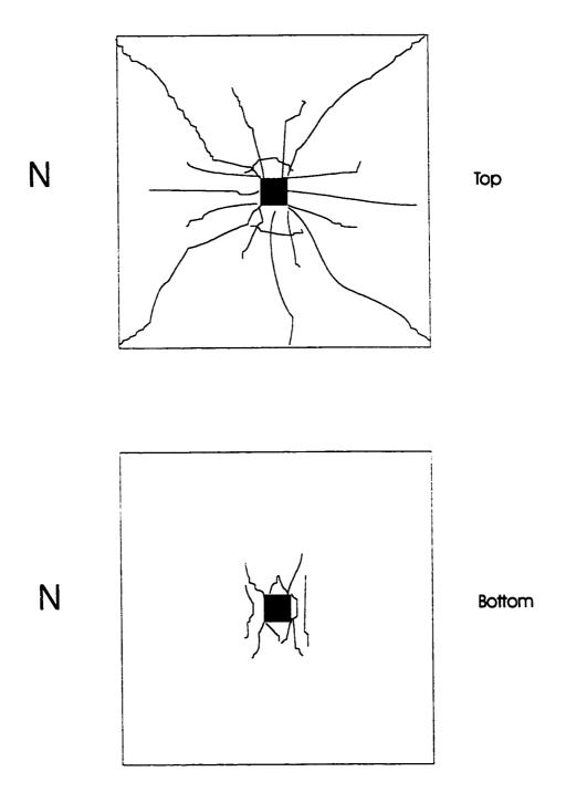
Figure 4.1 Final Crack Pattern of Steel Fibre Specimen
