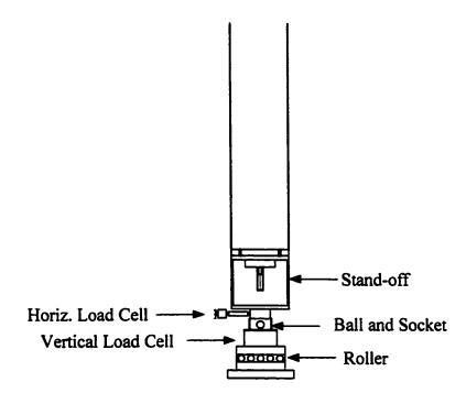
Figure 3.10 A Detail of Column Support
