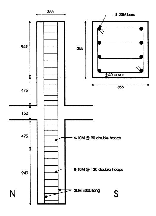
Figure 3.4 Column Reinforcement Layout
