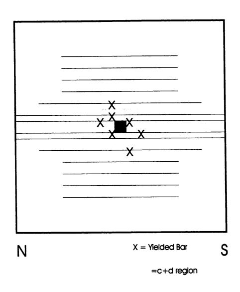
Figure 4.21 Yielded Bar Locations at Failure in Top Mat Control Specimen
