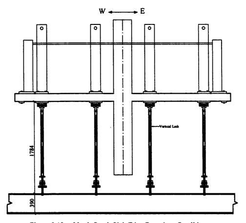
Figure 3.12 North-South Slab Edge Boundary Condition
