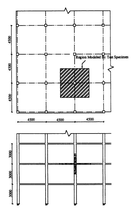
Figure 3.1 Prototype Flat Plate Structure
