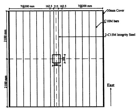
Figure 3.6 Slab Reinforcement - Bottom Mat (E-W Direction)
