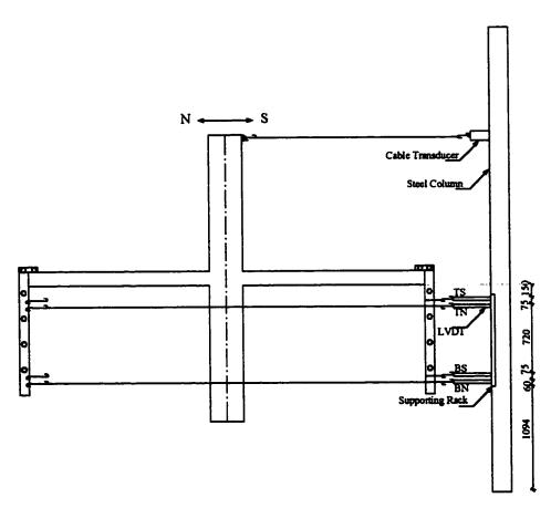
Figure 3.23 Position of Cable Transducers
