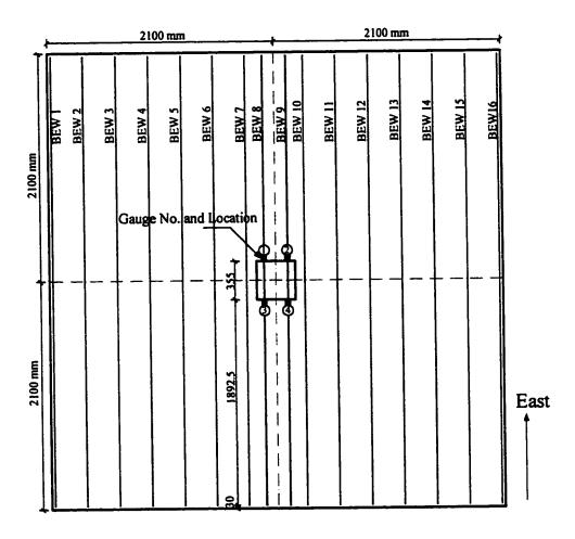
Figure 3.21 Bottom Mat Strain Gauge Locations (E-W Direction)
