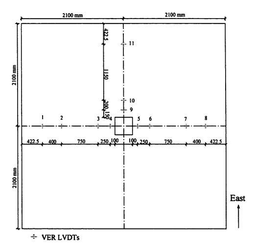
Figure 3.22 Position of Vertical LVDT's (Underside of Slab)
