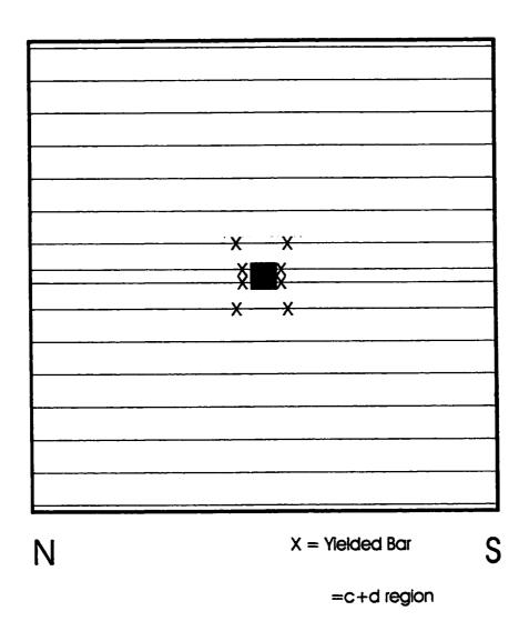
Figure 4.22 Yielded Bar Locations at Failure in Bottom Mat Steel Fibre Specimen
