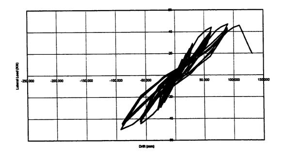
Figure 4.11 Horizontal Load vs. Lateral Drift Control Specimen
