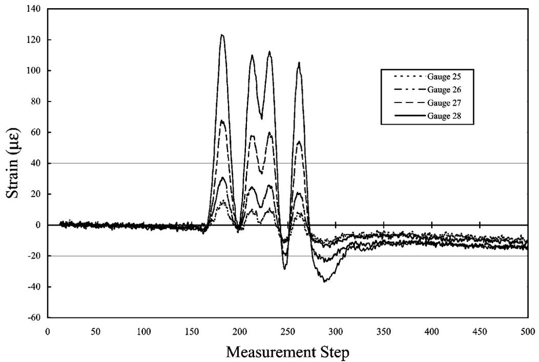
**Figure 4–24** Measured Dynamic Strain vs. Time Step – Gauges 25 Through 28, Girder 4 North
