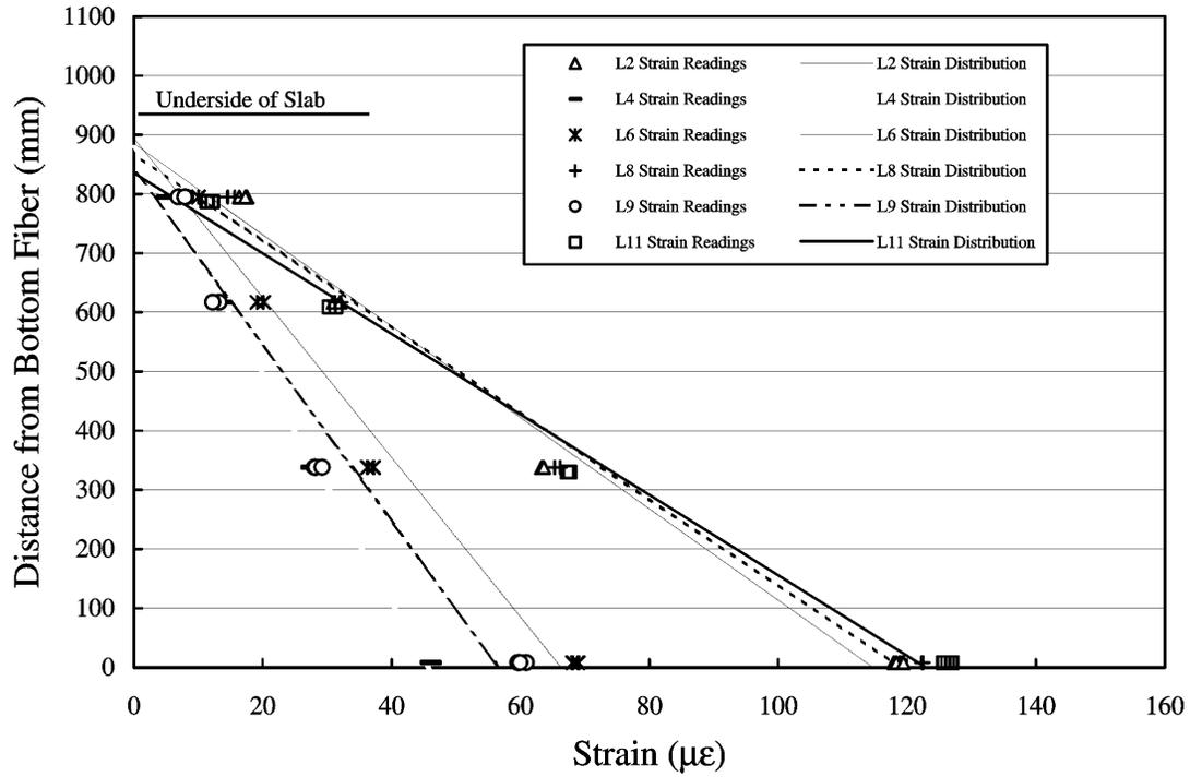
Figure 4-37 Static Strain Distributions, Locomotives Advancing Westward, Girder 3 North
