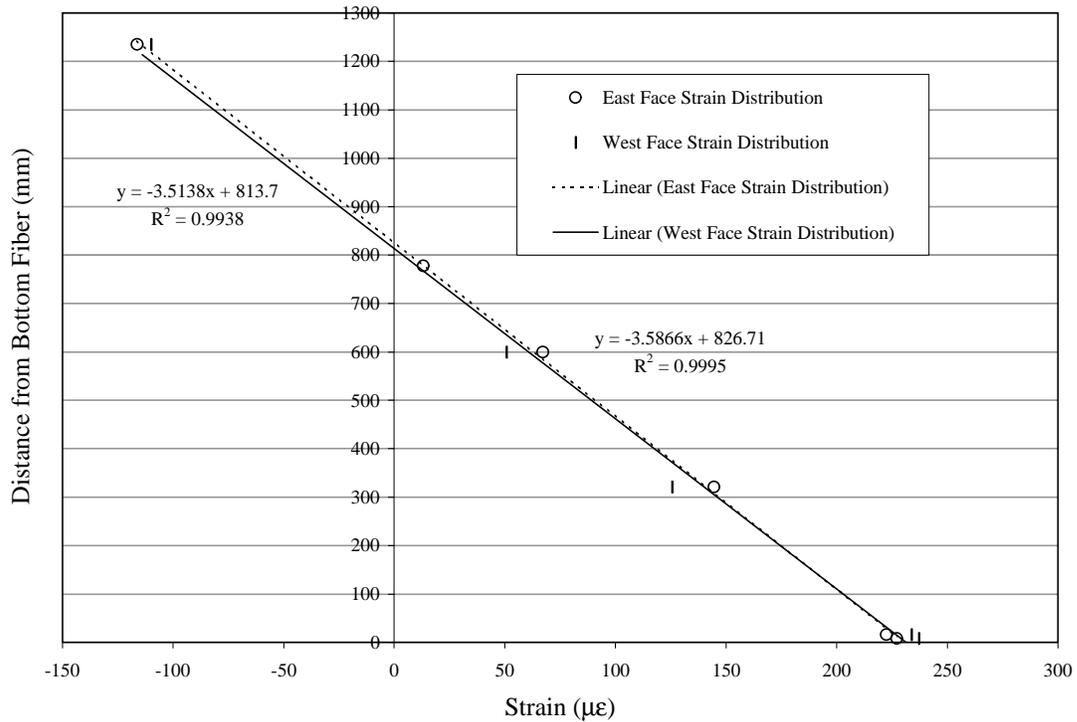
**Figure 6-4** Strain Distributions at Midspan of Test Specimen 1 ( $P_{static}=150$  kN/actuator)
