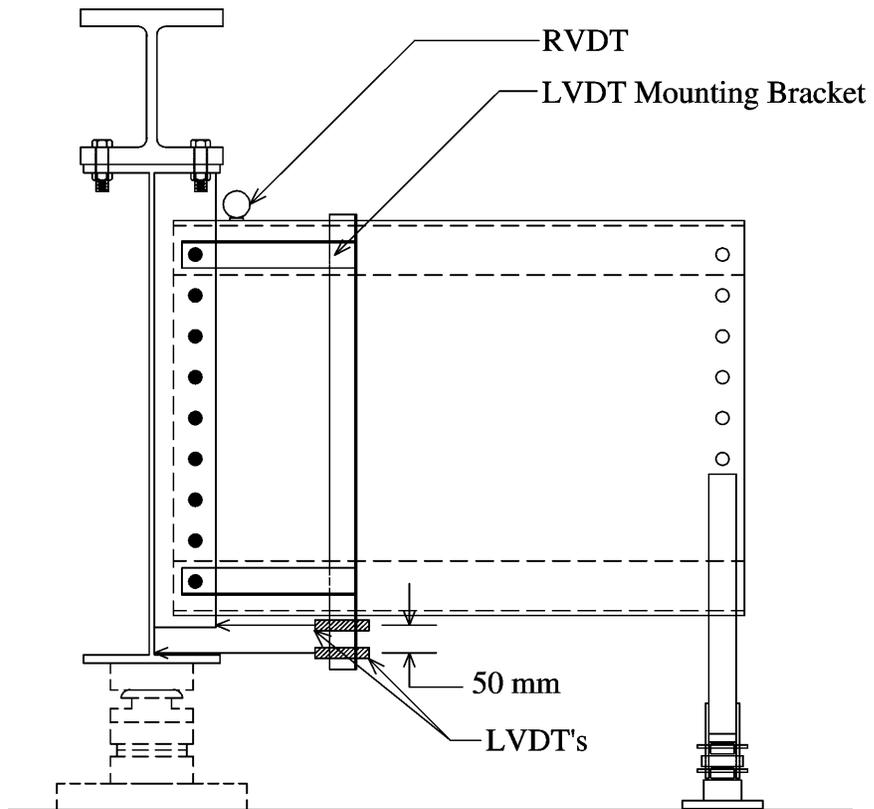
**Figure 5–12** Instruments Used to Measure Out-of-Plane Web Distortion
