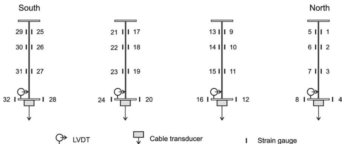
**Figure 3-1** Instrumentation of Girders Under Test Span
