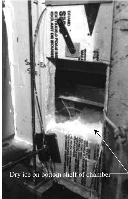
**Figure 5-8** View Inside Chamber Surrounding Joint 13 During Freeze Test
