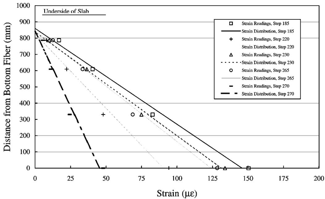
Figure 4-42 Dynamic Strain Distributions, Girder 3 North
