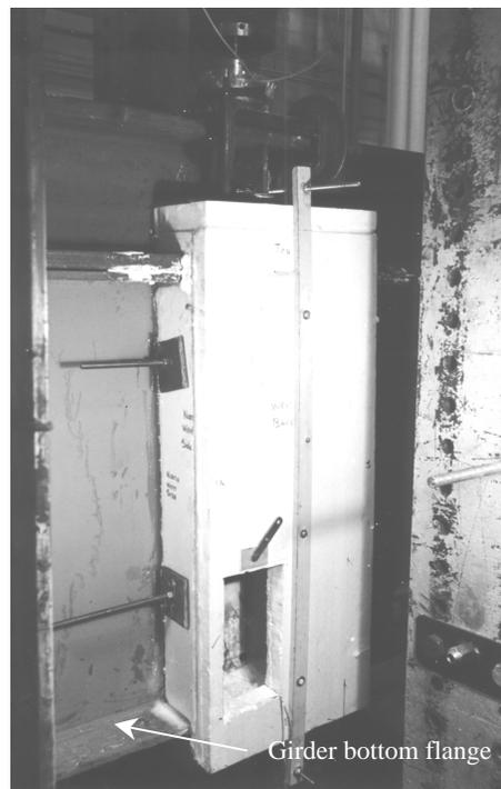
**Figure 5-7** West Side of Insulated Chamber Surrounding Joint 13, Test Specimen 2
