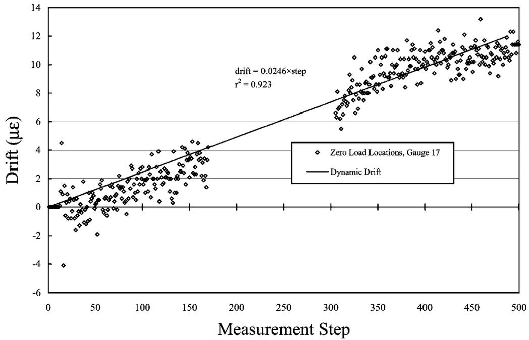
**Figure 4-26** Drift vs. Step, Gauge 17
