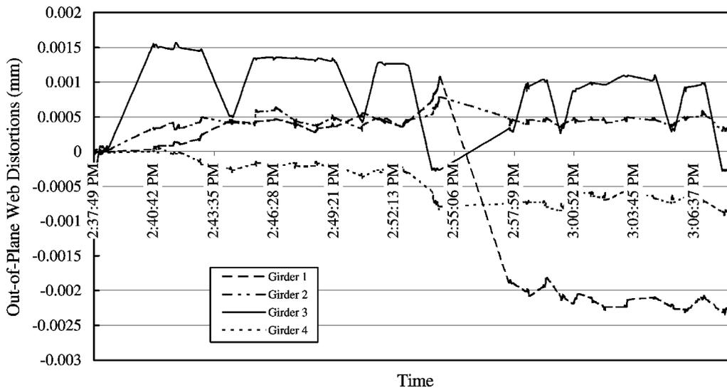
**Figure 4-47** Out-of-Plane Web Distortions Measured During Static Field Testing
