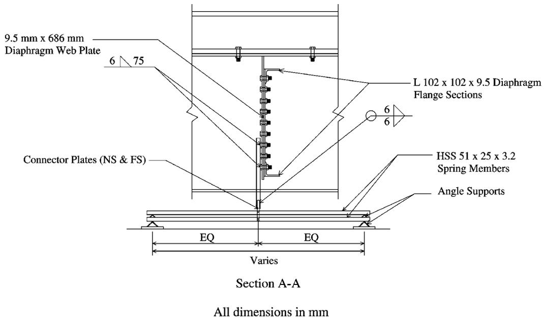
**Figure 5-3** Typical Cross-Section and Spring Support Details
