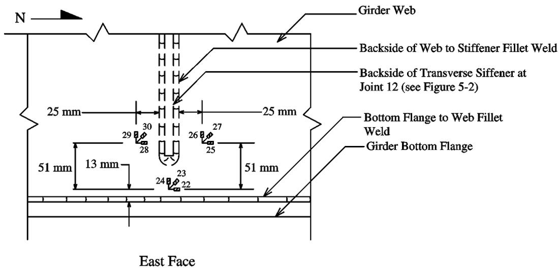
Figure 5-10 Location of Strain Rosettes at Joint 12
