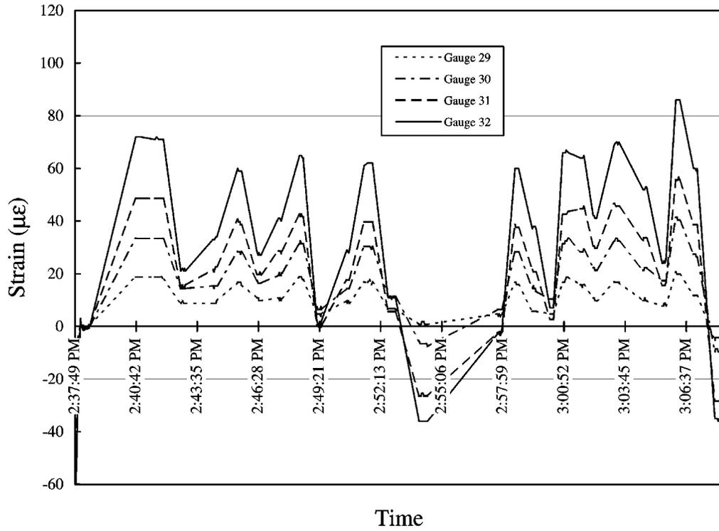
Figure 4-7 Measured Static Strain vs. Time Step – Gauges 29 Through 32, Girder 4 South
