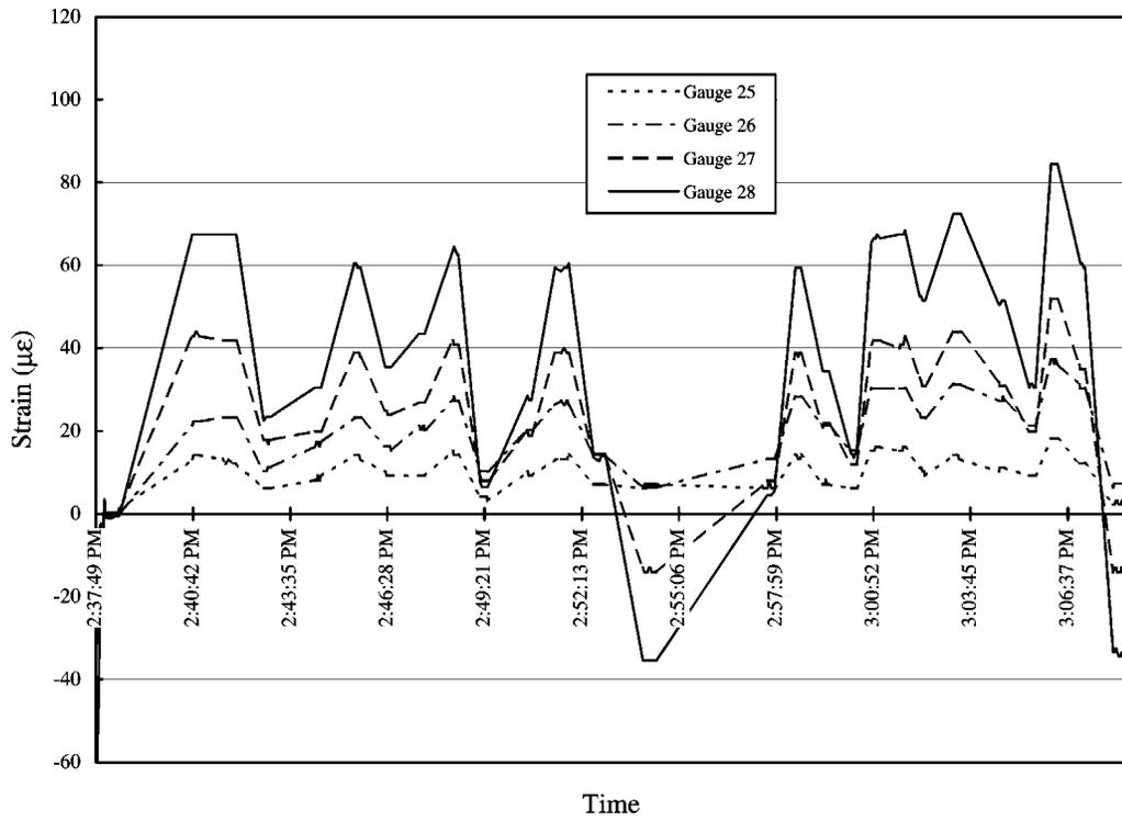
**Figure 4-46** Out-of-Plane Web Distortions Measured During Dynamic Field Testing
