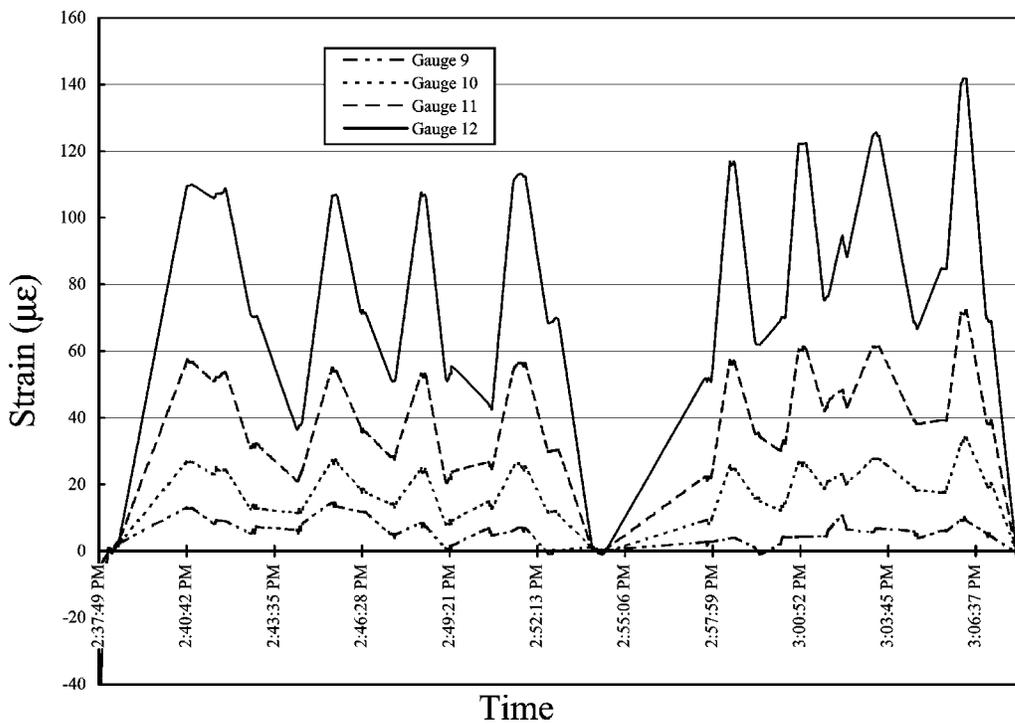
**Figure 4-14** Revised Static Measurements, Gauges 9 Through 12, Girder 2 North
