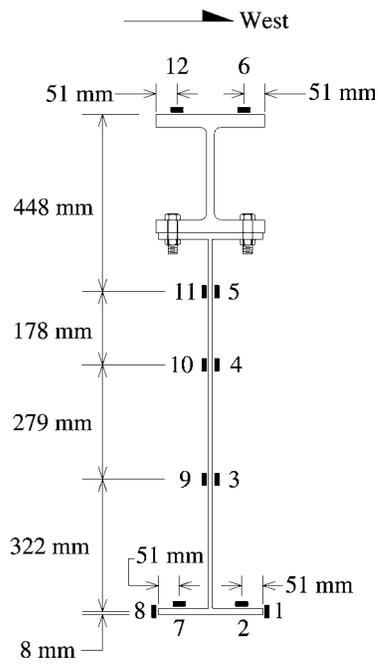
**Figure 5-9** Location of Strain Gauges Mounted at Midspan of Test Specimen
