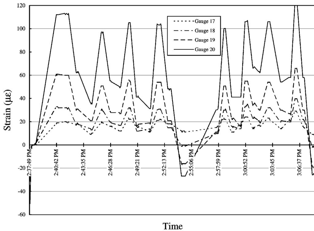
**Figure 4-5** Measured Static Strain vs. Time Step – Gauges 17 Through 20, Girder 3 North
