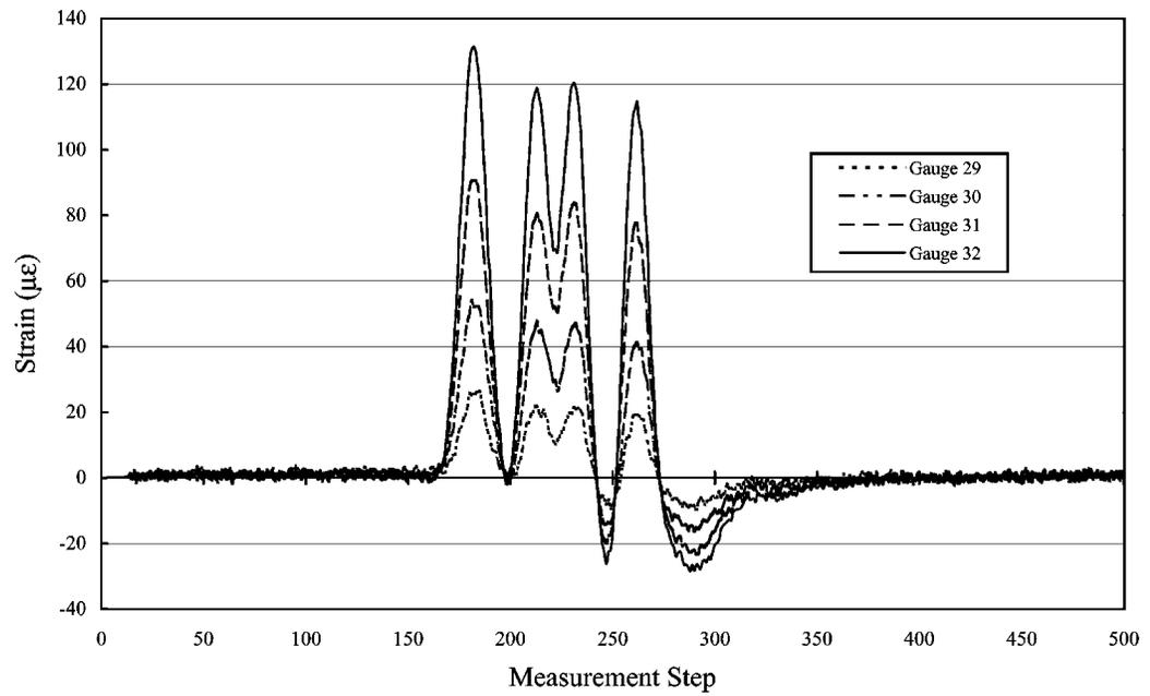
**Figure 4-36** Revised Dynamic Measurements, Gauges 29 Through 32, Girder 4 South
