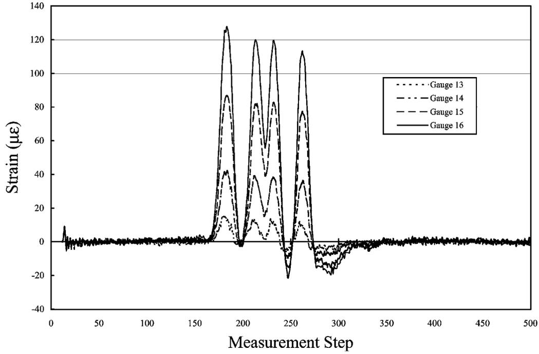
**Figure 4-33** Revised Dynamic Measurements, Gauges 13 Through 16, Girder 2 South
