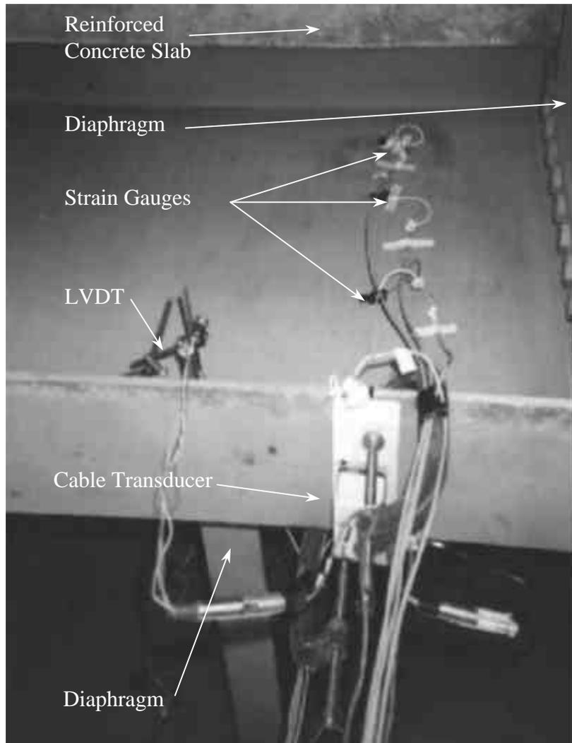
**Figure 3–3** Typical Field Instrumentation at Midspan of Test Girders
