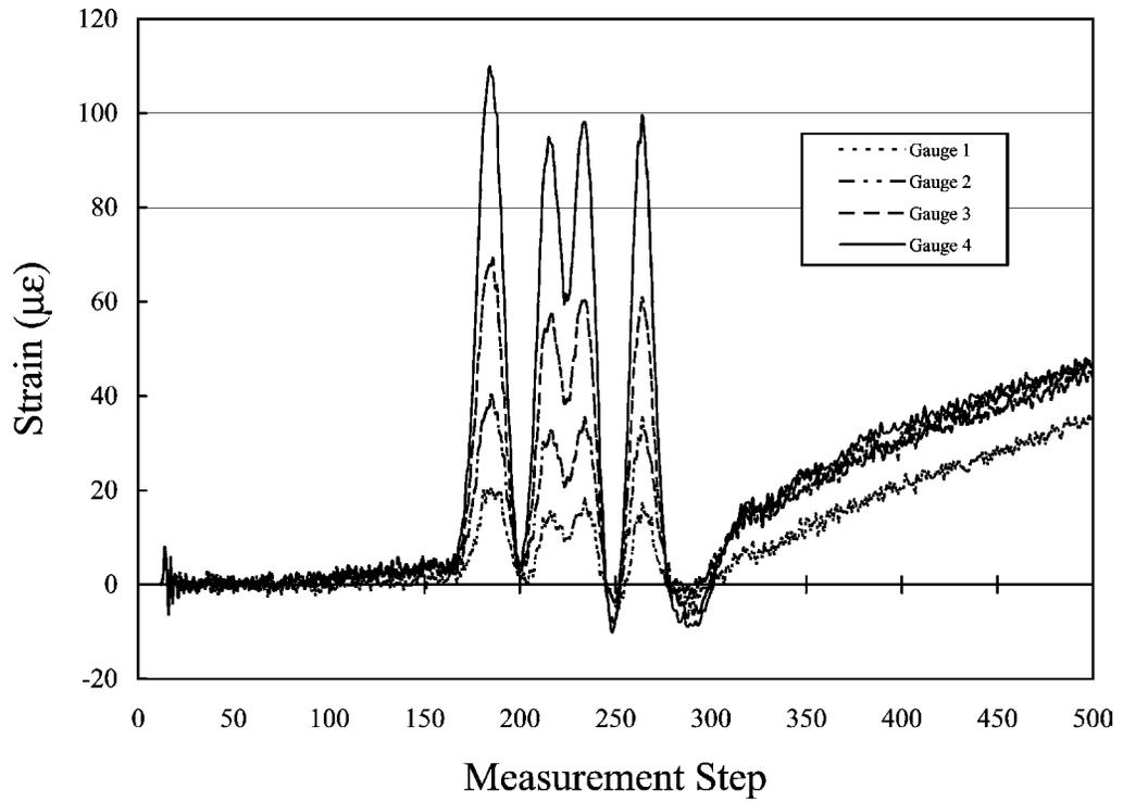
**Figure 4–19** Measured Dynamic Strain vs. Time Step – Gauges 1 Through 4, Girder 1 North
