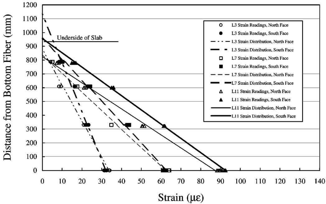
Figure 4-41 Strain Distribution on the North and South Face of Girder 4
