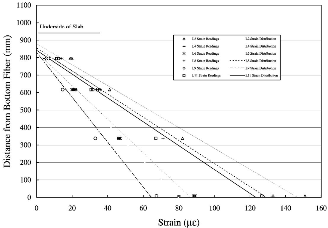
Figure 4-38 Static Strain Distributions, Locomotives Advancing Eastward, Girder 3 North
