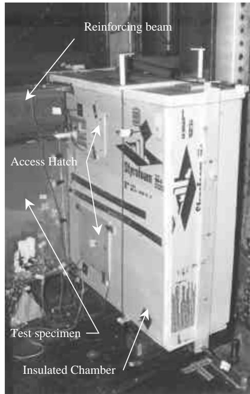
**Figure 5-6** East Side of Insulated Chamber Surrounding Joint 11, Test Specimen 2
