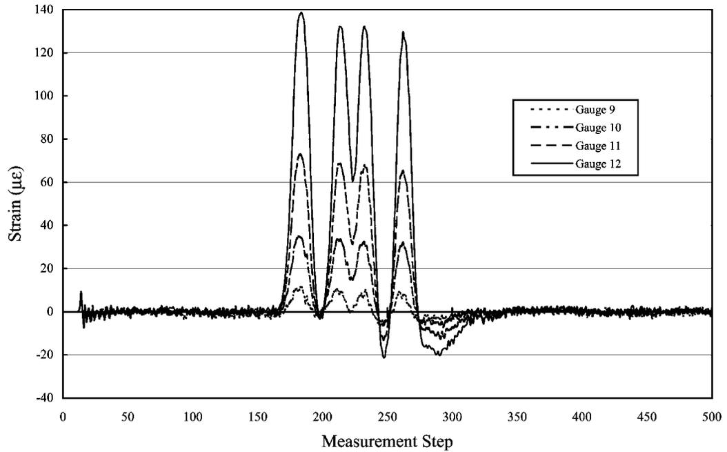
**Figure 4-32** Revised Dynamic Measurements, Gauges 9 Through 12, Girder 2 North
