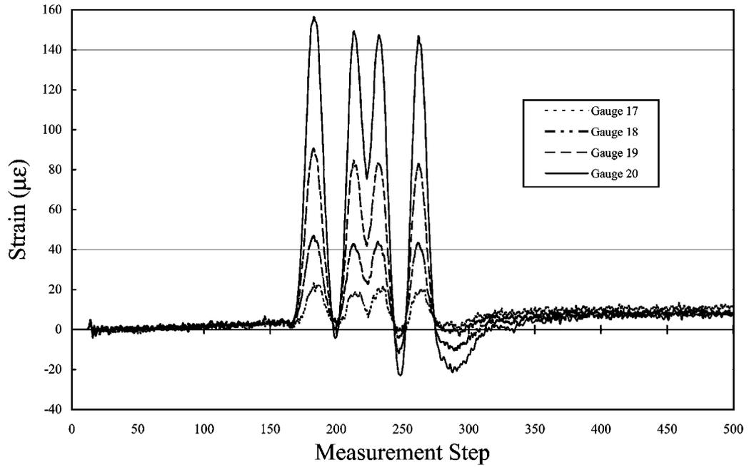
**Figure 4–23** Measured Dynamic Strain vs. Time Step – Gauges 17 Through 20, Girder 3 North
