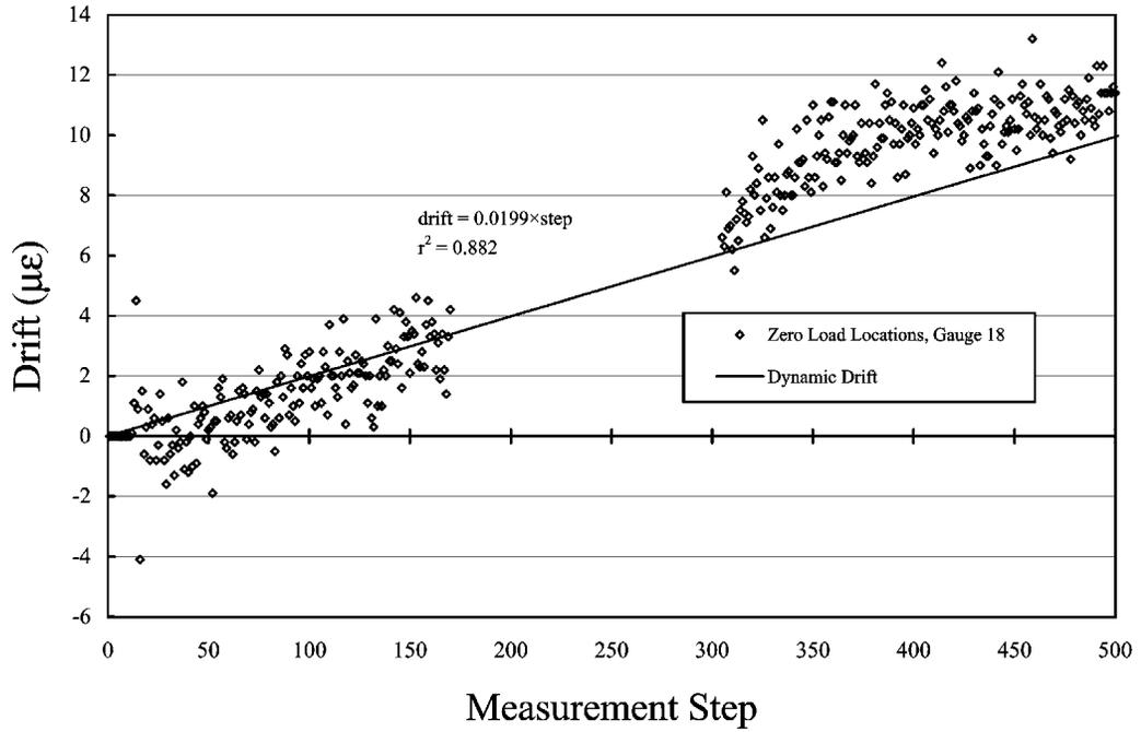
Figure 4–27 Drift vs. Step, Gauge 18
