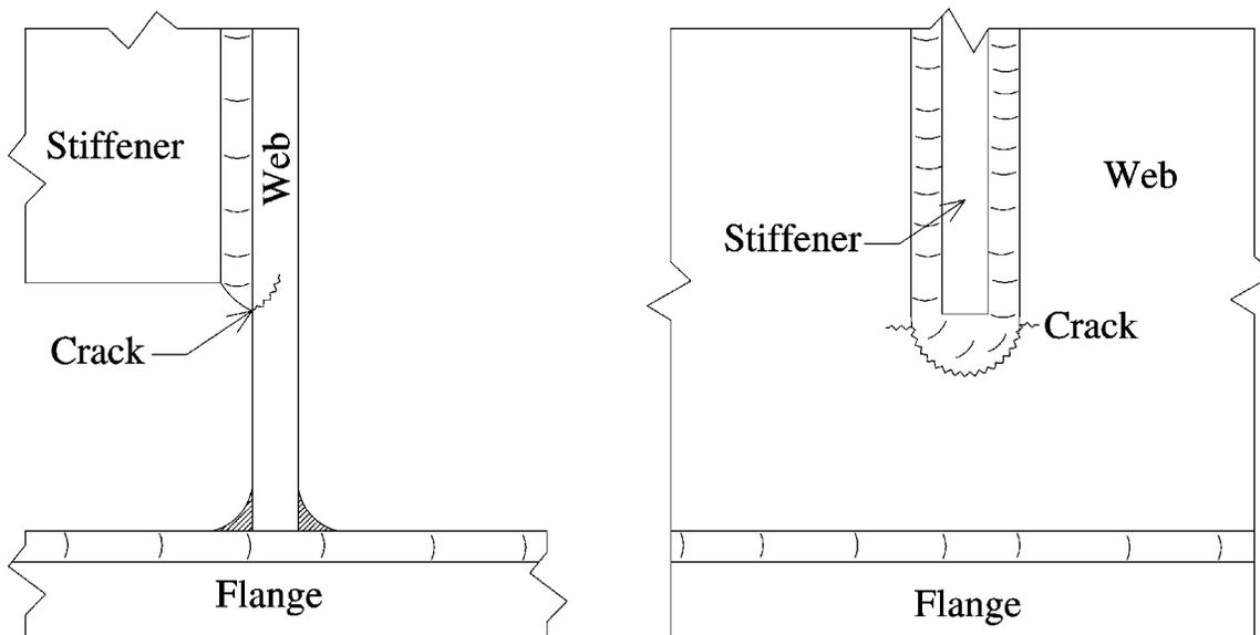
**Figure 2-2** Schematic of Web Crack at End of Transverse Stiffener (Fisher, 1978)
