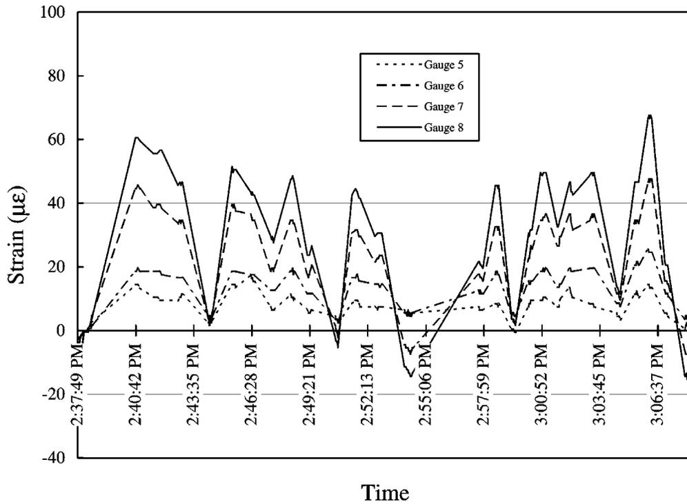
**Figure 4-2** Measured Static Strain vs. Time Step – Gauges 5 Through 8, Girder 1 South
