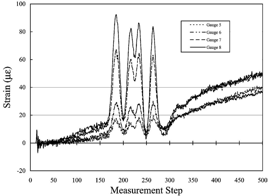
**Figure 4–20** Measured Dynamic Strain vs. Time Step – Gauges 5 Through 8, Girder 1 South
