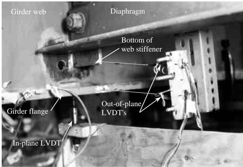
**Figure 5–11** Typical Orientation of LVDT's Mounted Beneath Diaphragm Locations
