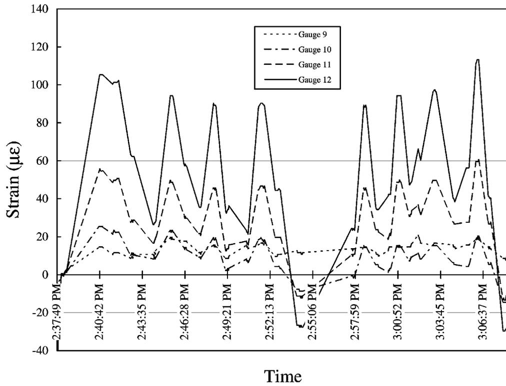
**Figure 4-3** Measured Static Strain vs. Time Step – Gauges 9 Through 12, Girder 2 North
