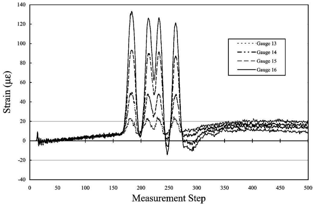
**Figure 4–22** Measured Dynamic Strain vs. Time Step – Gauges 13 Through 16, Girder 2 South
