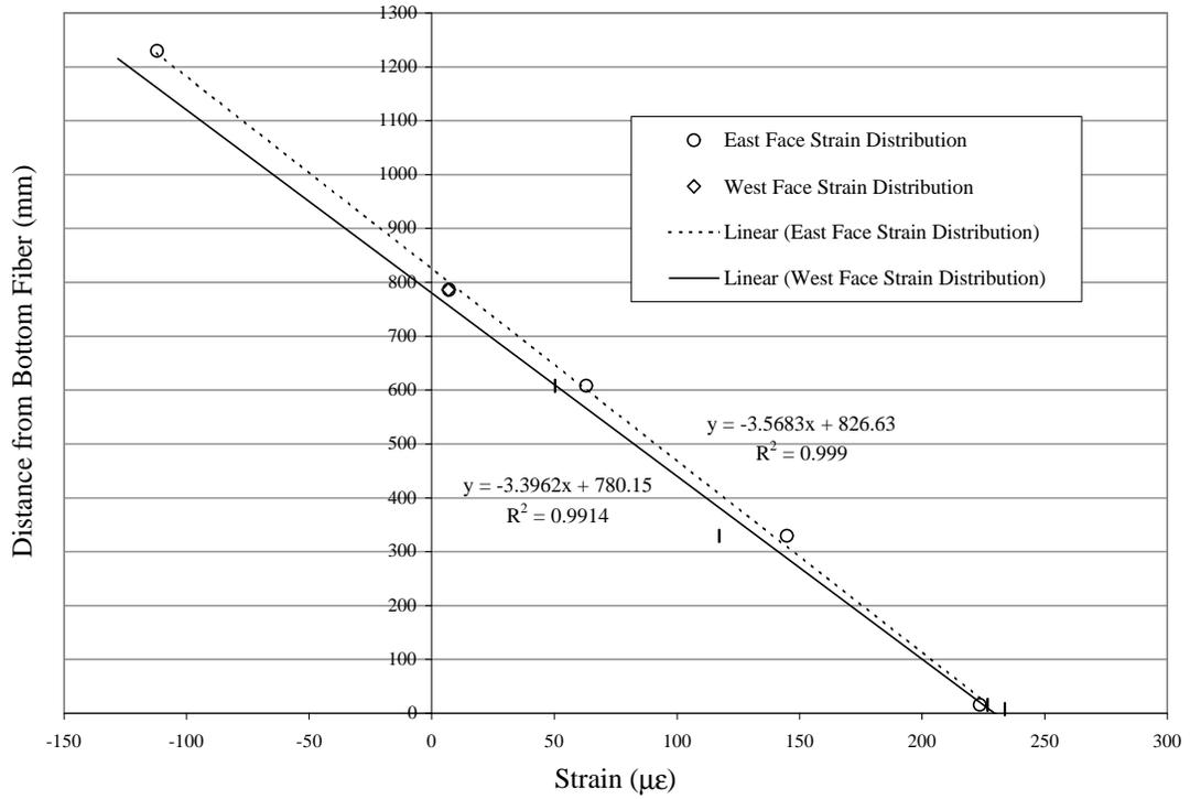
**Figure 6-5** Strain Distributions at Midspan of Test Specimen 2 ( $P_{\text{static}}=152$  kN/actuator)
