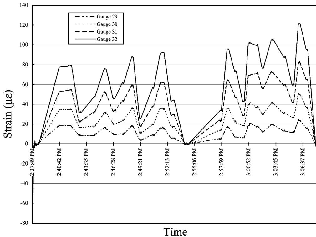
**Figure 4-18** Revised Static Measurements, Gauges 29 Through 32, Girder 4 South
