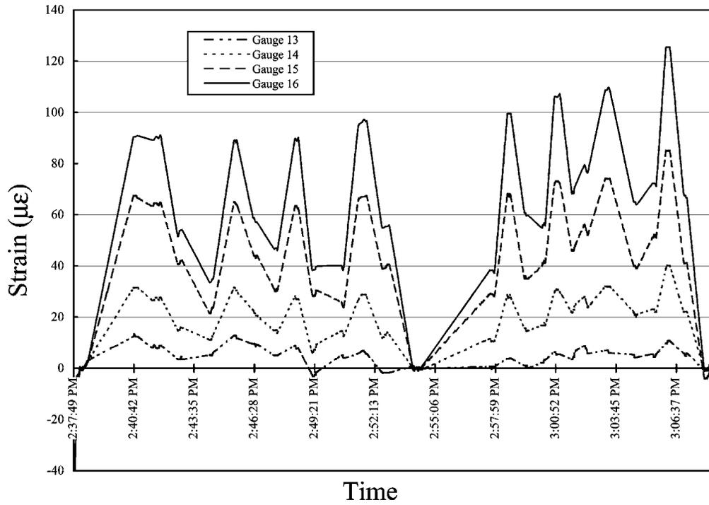
**Figure 4-15** Revised Static Measurements, Gauges 13 Through 16, Girder 2 South
