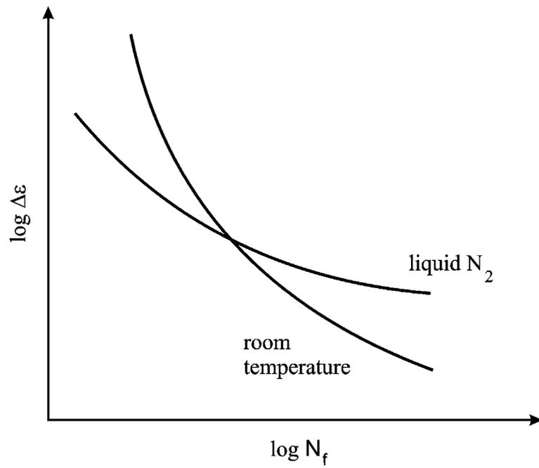
**Figure 2-4** Effect of Low Temperatures on Stress-Based Total Fatigue Life
