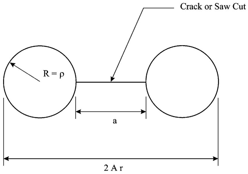
**Figure 2-3** Hole Drilling Rehabilitation (Lai, 1997)
