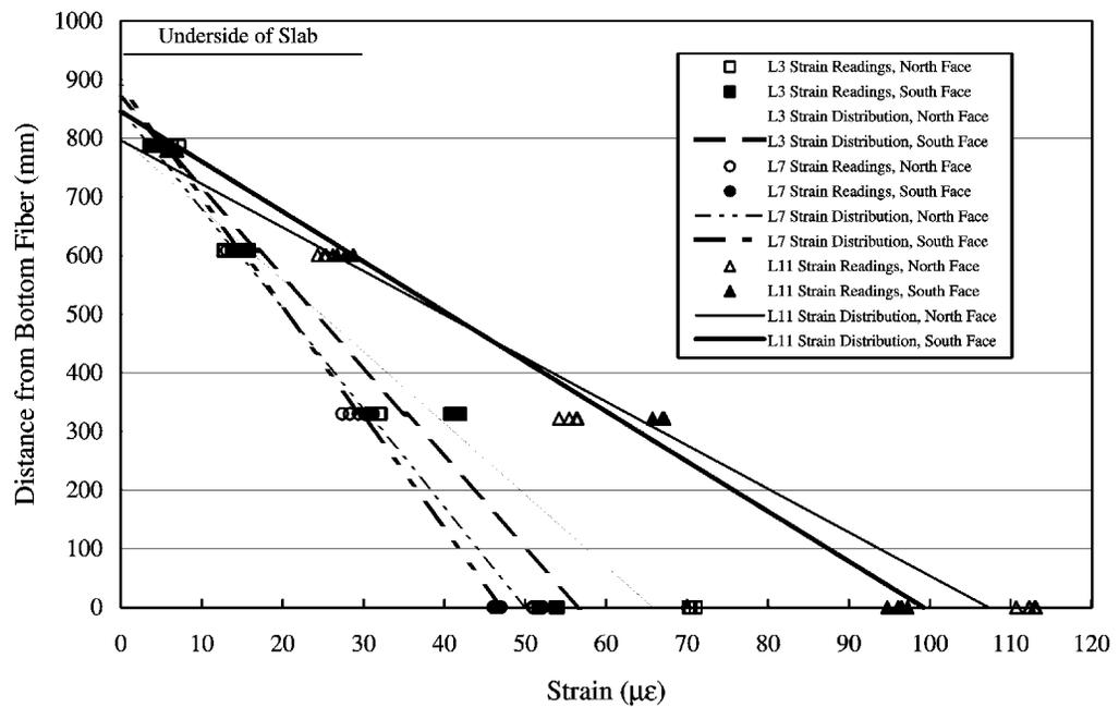
Figure 4-40 Strain Distribution on the North and South Face of Girder 2
