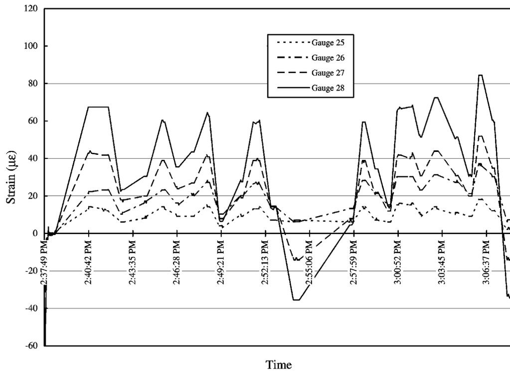
**Figure 4-6** Measured Static Strain vs. Time Step – Gauges 25 Through 28, Girder 4 North
