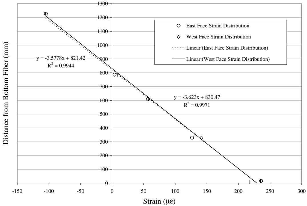
**Figure 6-6** Strain Distributions at Midspan of Test Specimen 3 ( $P_{\text{static}}=150$  kN/actuator)
