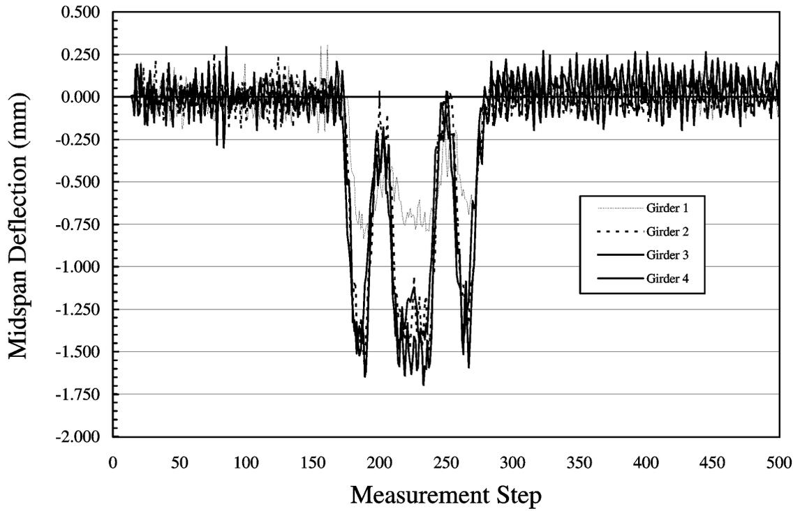
**Figure 4-43** Dynamic Vertical Displacement at Midspan of Girders
