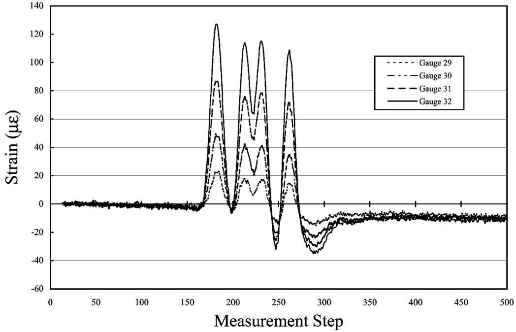
**Figure 4-25** Measured Dynamic Strain vs. Time Step – Gauges 29 Through 32, Girder 4 South
