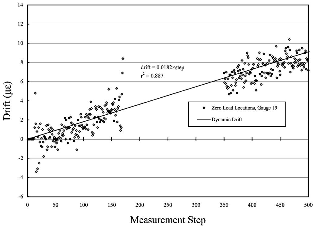
Figure 4–28 Drift vs. Step, Gauge 19
