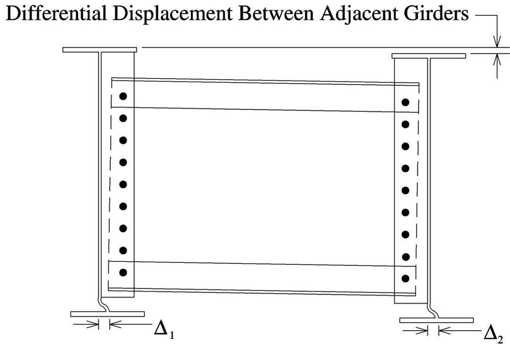
**Figure 2-1** Typical Out-of-Plane Web Distortion Mode Concentrated in Web Gap
