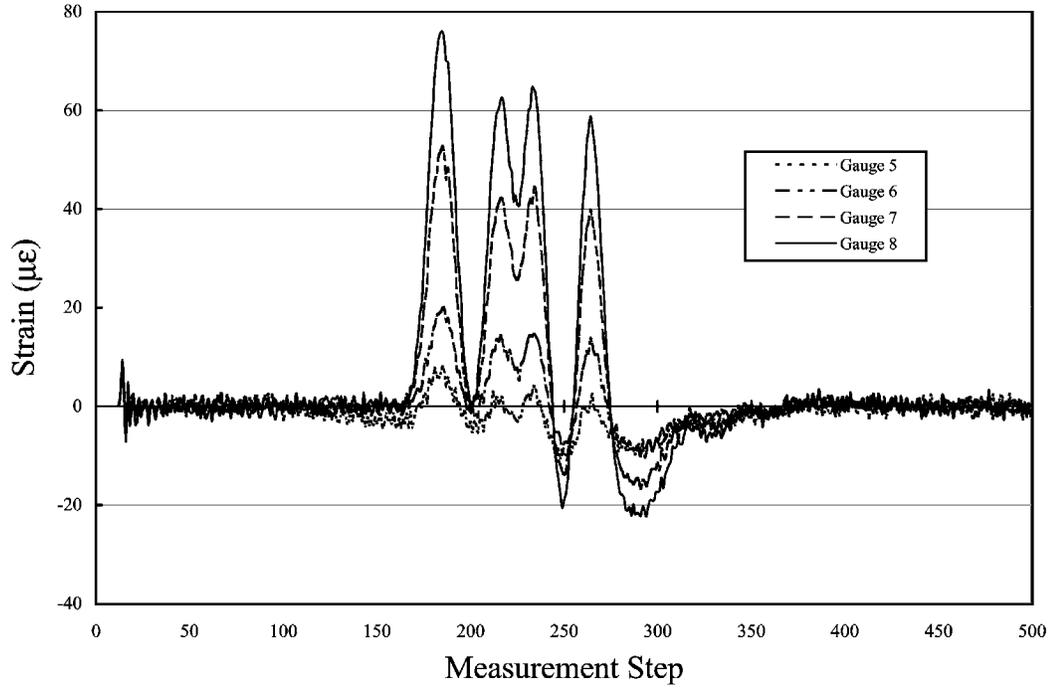
**Figure 4-31** Revised Dynamic Measurements, Gauges 5 Through 8, Girder 1 South
