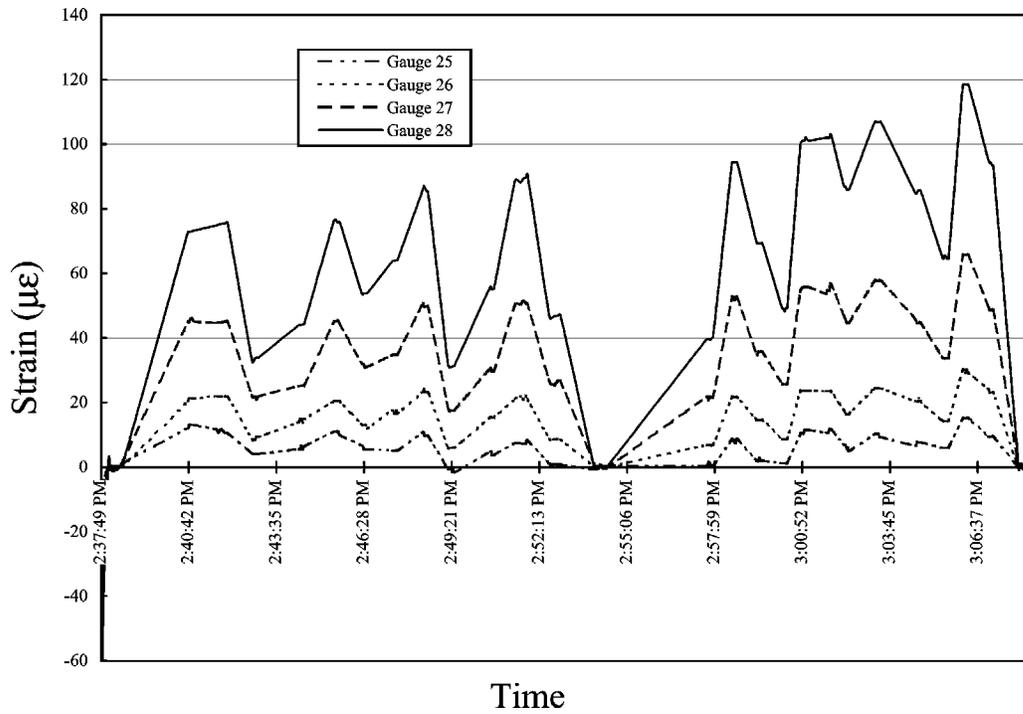
**Figure 4-17** Revised Static Measurements, Gauges 25 Through 28, Girder 4 North
