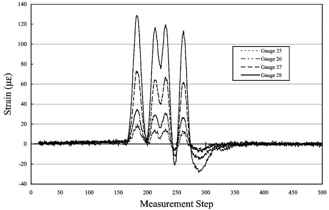
**Figure 4-35** Revised Dynamic Measurements, Gauges 25 Through 28, Girder 4 North
