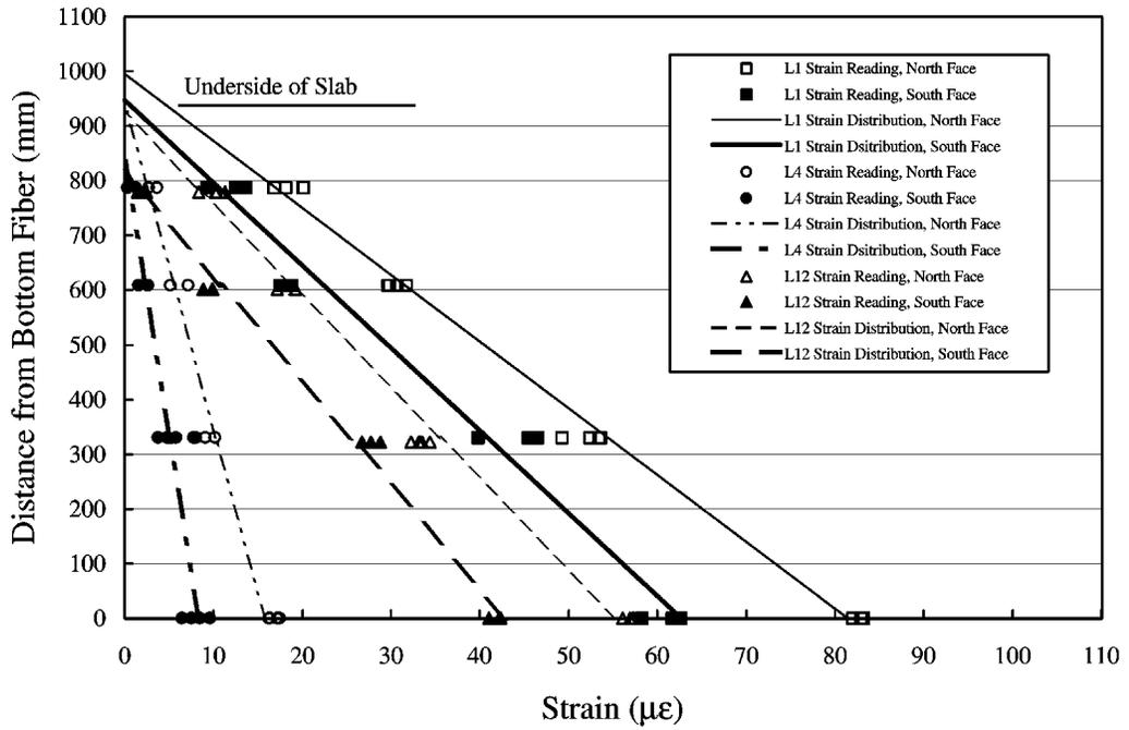
Figure 4-39 Strain Distribution on the North and South Face of Girder 1
