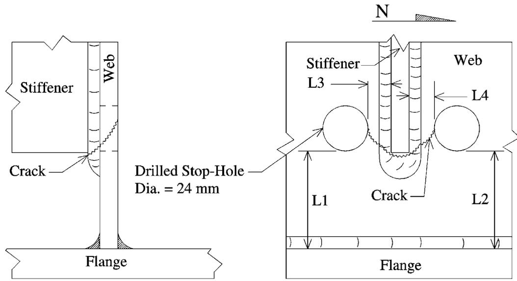
**Figure 6-1** Typical Orientation of Stop Holes and Cracks in Test Girder Sections
