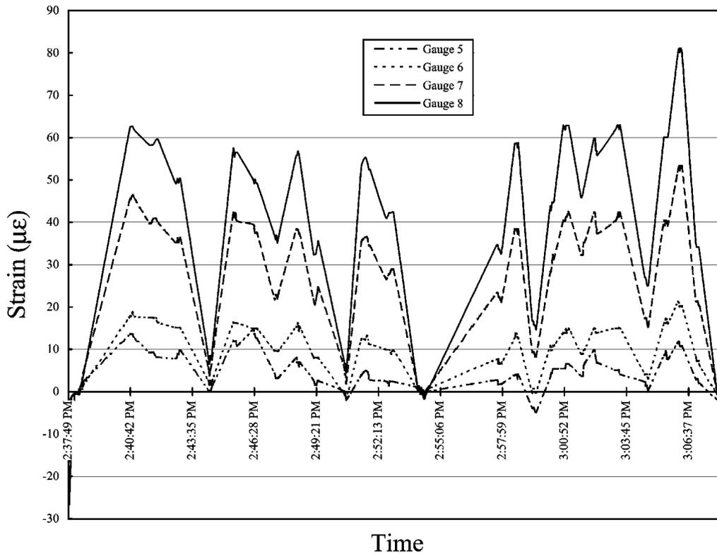
**Figure 4-13** Revised Static Measurements, Gauges 5 Through 8, Girder 1 South
