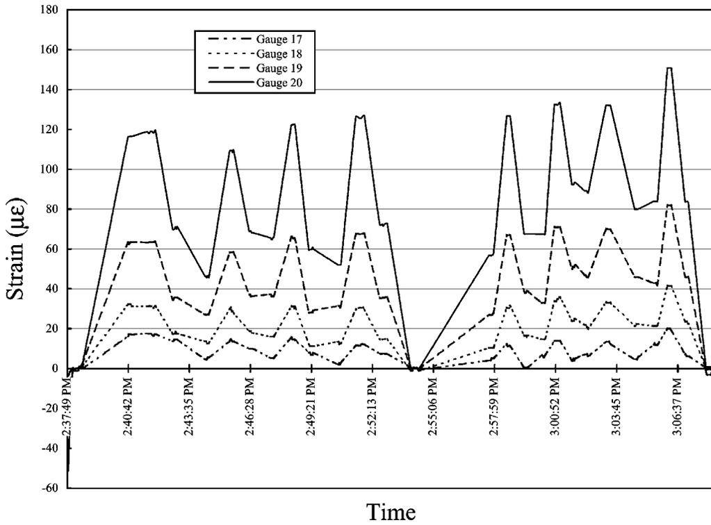
**Figure 4-16** Revised Static Measurements, Gauges 17 Through 20, Girder 3 North
