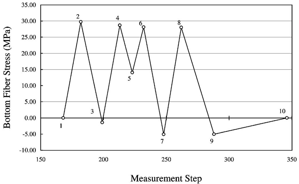
**Figure 4-44** Bottom Fiber Stress vs. Dynamic Measurement Step, Girder 3
