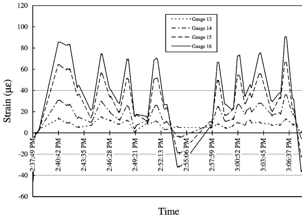
**Figure 4-4** Measured Static Strain vs. Time Step – Gauges 13 Through 16, Girder 2 South
