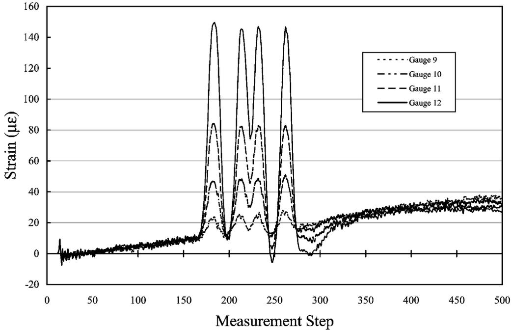
**Figure 4–21** Measured Dynamic Strain vs. Time Step – Gauges 9 Through 12, Girder 2 North
