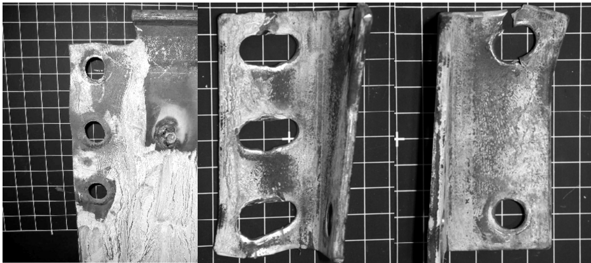
Angle leg connected to the column
