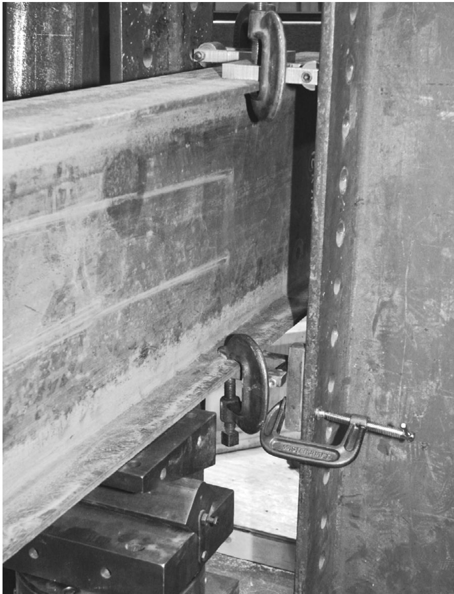
Figure 3-13 Lateral Bracing at Reaction Frame
