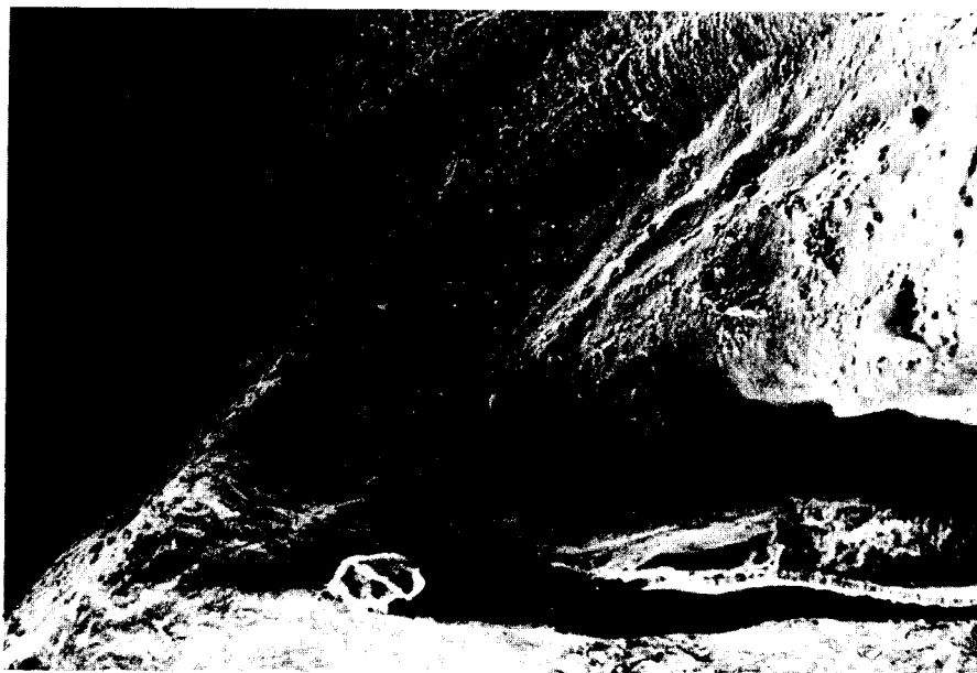
FIGURE 4.11(c) FATIGUE CRACK (X200)
