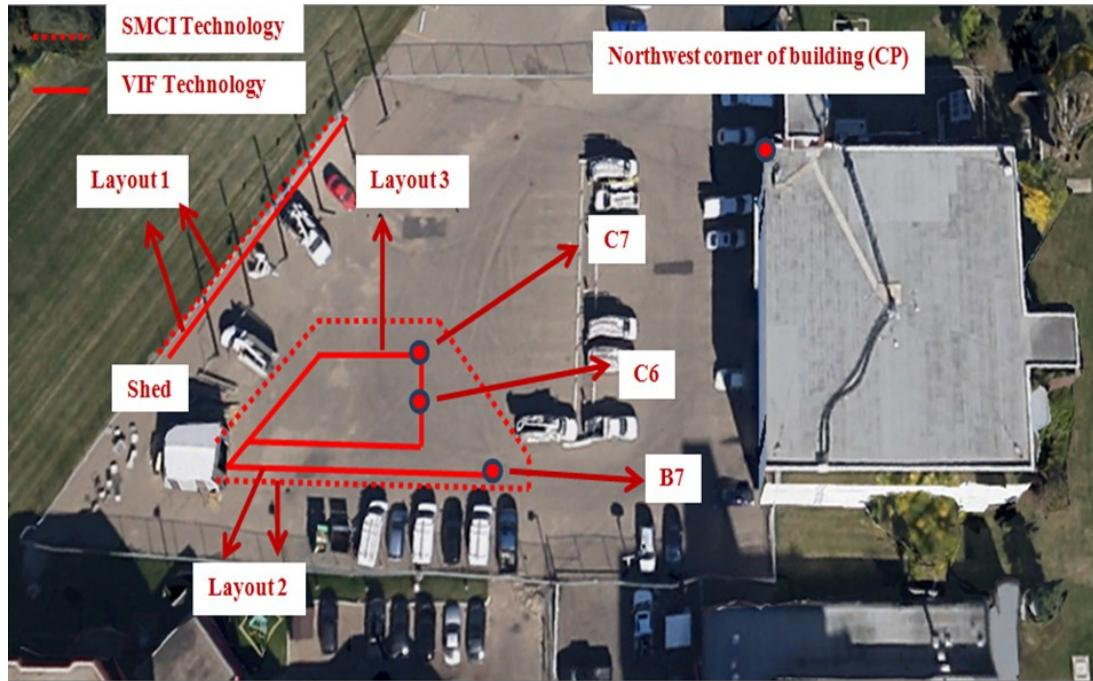
Figure 3-1: Installation layouts, Control Point (CP), shallowest points (C7, C6 & B7)
