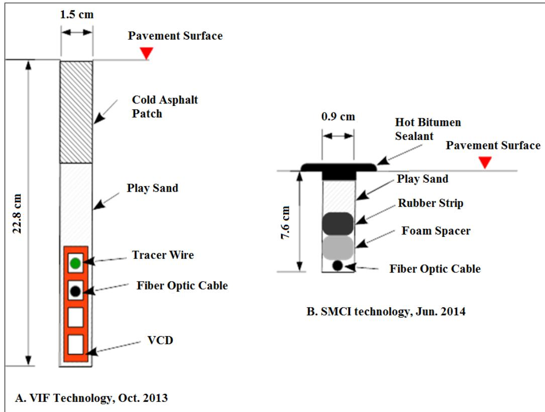
Figure 3-3: Cross section of VIF and SMCI installations
