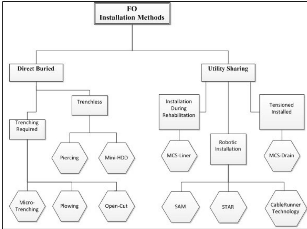
Figure 2-1: Fiber Optic Deployment Methods' Classification Diagram
