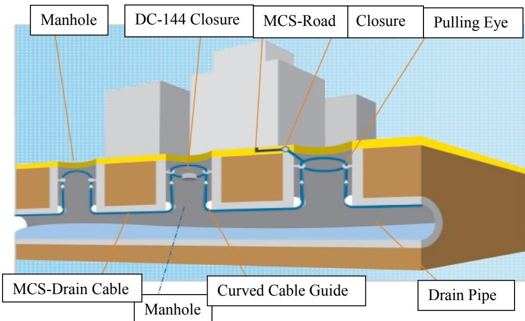
**Figure 2-6: MCS-Drain Installation Diagram (Reprinted from Corning Cable System 2001, with permission)**
