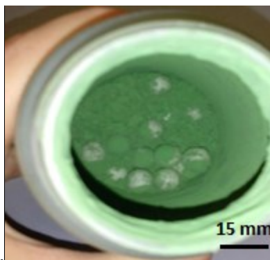
Figure 7. Mixed and dried \text{Cr}_2\text{O}_3 -Co powder
