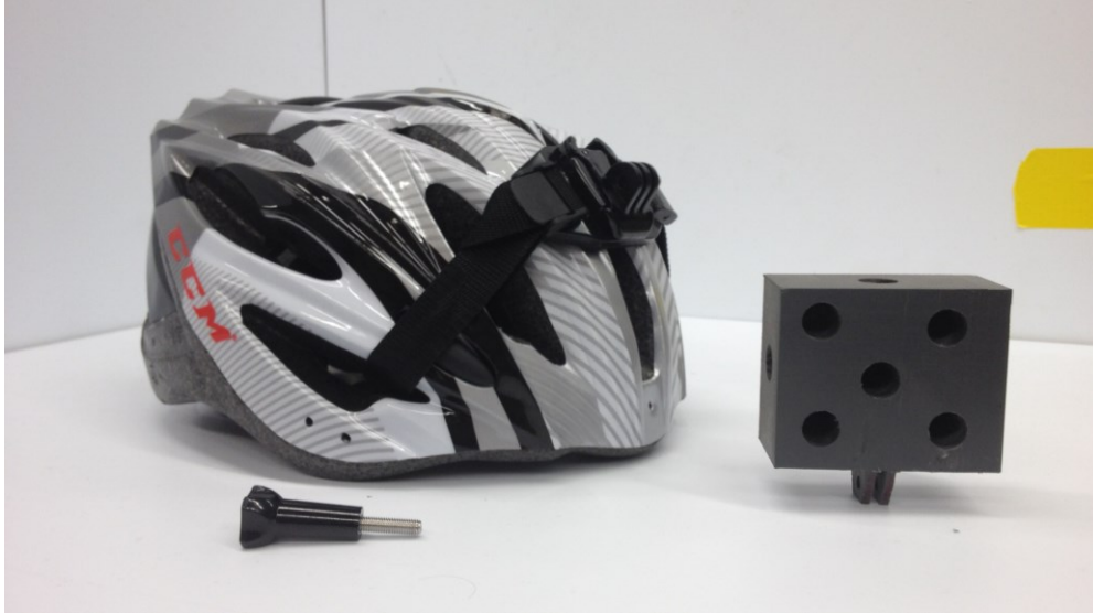
Figure 6.2: Photo of CCM Nexus size medium helmet (mass: 283 \pm 3 grams). 12 bicycle helmets were left unmodified and 12 were equipped with a GoPro vented helmet strap camera mount. A surrogate camera model made of impact resistant polyvinyl chloride (mass: 150 grams, dimensions: 70 mm x 60 mm x 30 mm).
