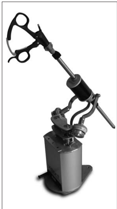
Example of a Computer-Based Simulator with Tactile (Haptic) Feedback: Xitact ITP — Instrument Tracking Port™ www.xitact.com
