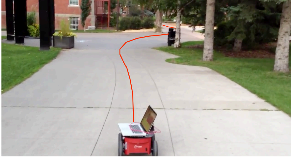
Figure 4.11: The robot replaying the outdoor path using Gabor-gist homing.
