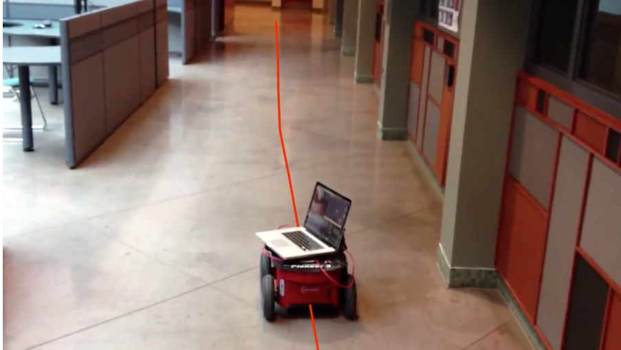
Figure 4.6: Indoor experiment, testing the methods ability to perform proper localization down a hallway. This experiment tests the ability to travel a straight line and also to properly localize the robot in an environment with many repeating patterns. This path is approximately 12 m. The robot completed the path successfully.
