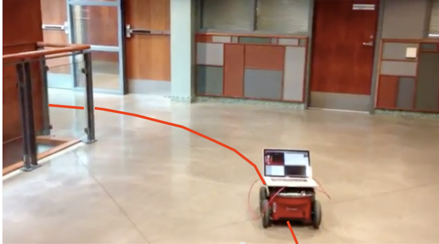
Figure 4.7: Indoor experiment, testing the methods ability to perform the types of turns required for indoor navigation. The path is approximately 10m. The robot completed the path successfully.
