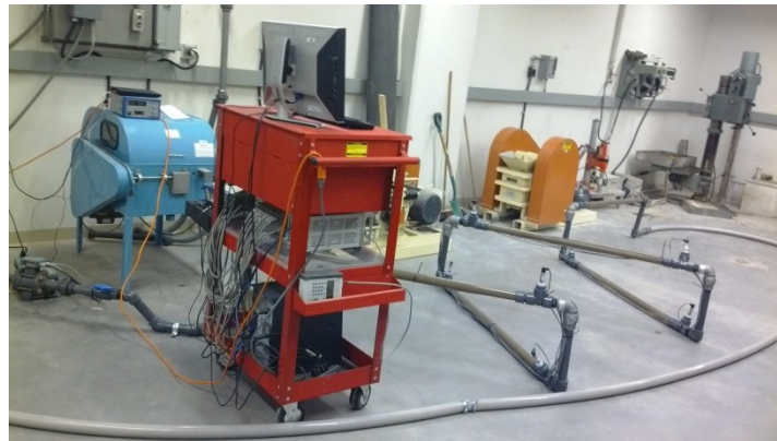
Figure 4-6 Pipe loop with alignment angle 80^\circ
