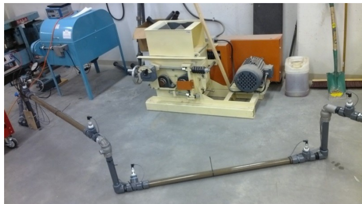
Figure 4-4 Pipe loop with alignment angle 30^\circ
