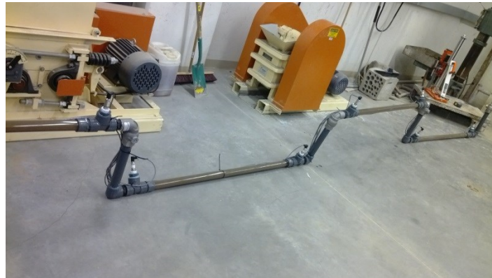
Figure 4-3 Pipe loop with alignment angle 0^\circ
