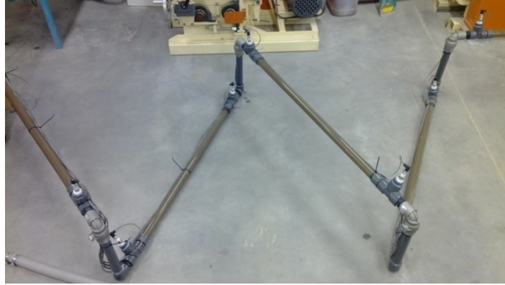
Figure 4-5 Pipe loop with alignment angle 60^\circ
