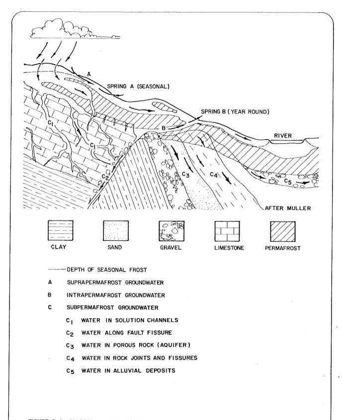
FIGURE 2.1 DIAGRAM SHOWING OCCURRENCE OF GROUNDWATER IN PERMAFROST REGIONS .
