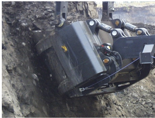
Figure 2.4 Rope shovel free-falling pendulum doors dipper with a curved shape front lip (The picture was kindly provided by Dr. Tim Grain Joseph, University of Alberta)
