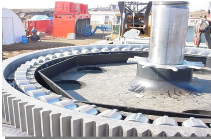
Figure 2.7 Rope shovel rotating circle and cylindrical rollers (The picture was kindly provided by Dr. Tim Grain Joseph, University of Alberta)
