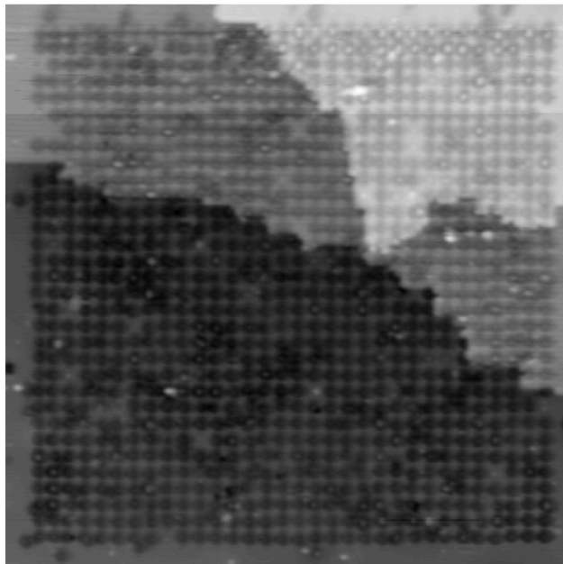
Figure 6.9: Grid of DBs at a 2nm pitch. Pulse bias was +2.4V and \Delta z_{\text{pulse}} was -150pm. Pulse width was 2 ms.
