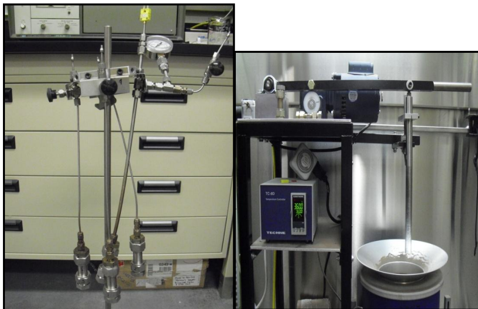
Figure 3.5. Left: Holder and micro-reactors. Right: Sand bath, motor and rod.
