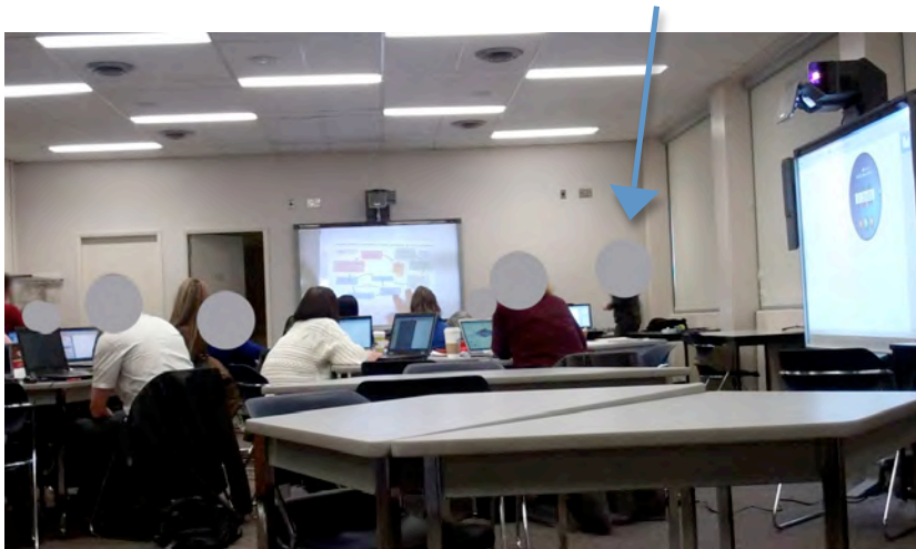
Figure 9 – Document camera (far right, behind trainer) is integrated into SMART Notebook software and its image is displayed on the IWB
