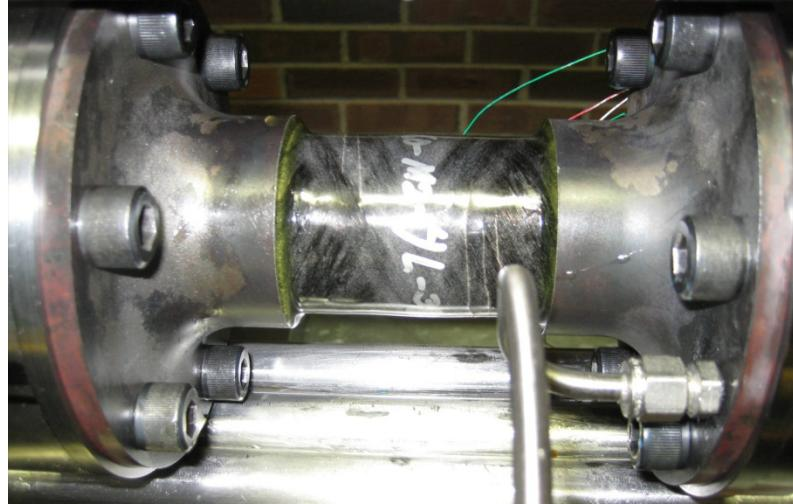
Figure 3-3: A four layer dual-wall specimen, subjected to pure tensile loading, showing surface cracks in the hoop direction
