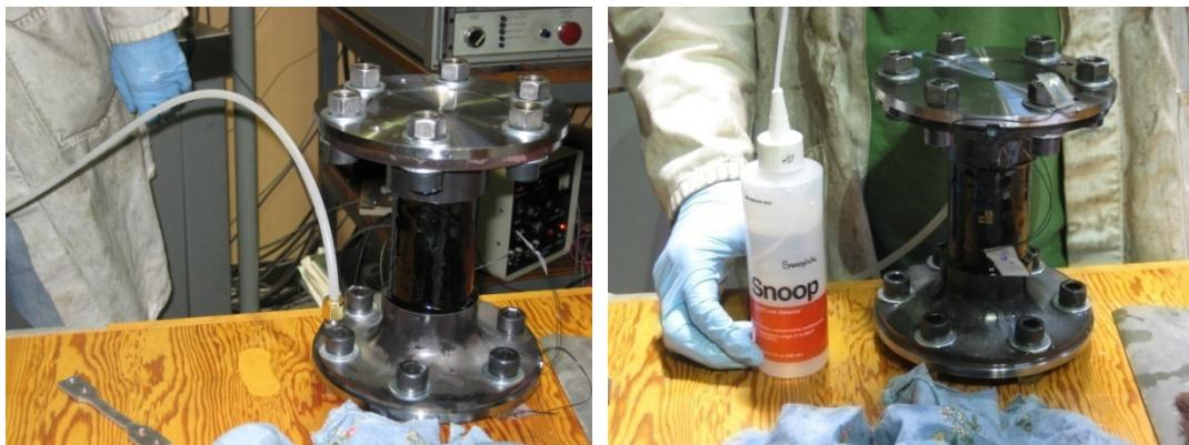
Figure 2-17: The specimen is pressurized with air to 207 kPa.
