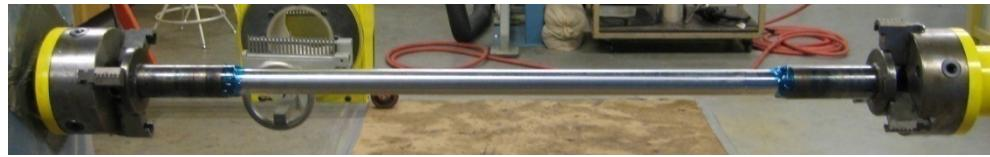
Figure 2-28: An installed 1.5 inch mandrel
