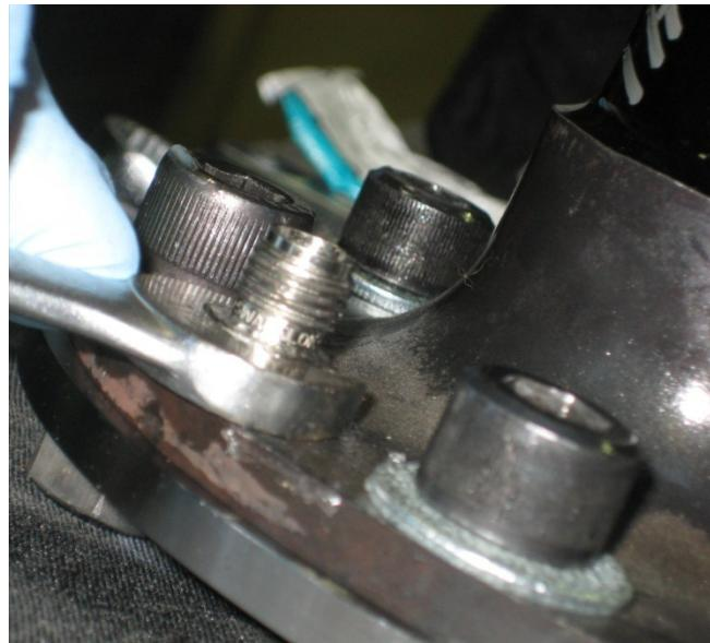
Figure 2-16: Attaching the 10-32 adapter to the supply flange
