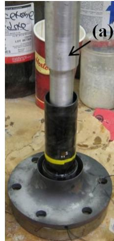
Figure 2-4: A 38.1 mm specimen employing (a) the alignment jig
