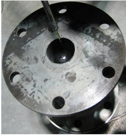
Figure 2-13: NUTO H 46 hydraulic fluid filling the inner tubular specimen
