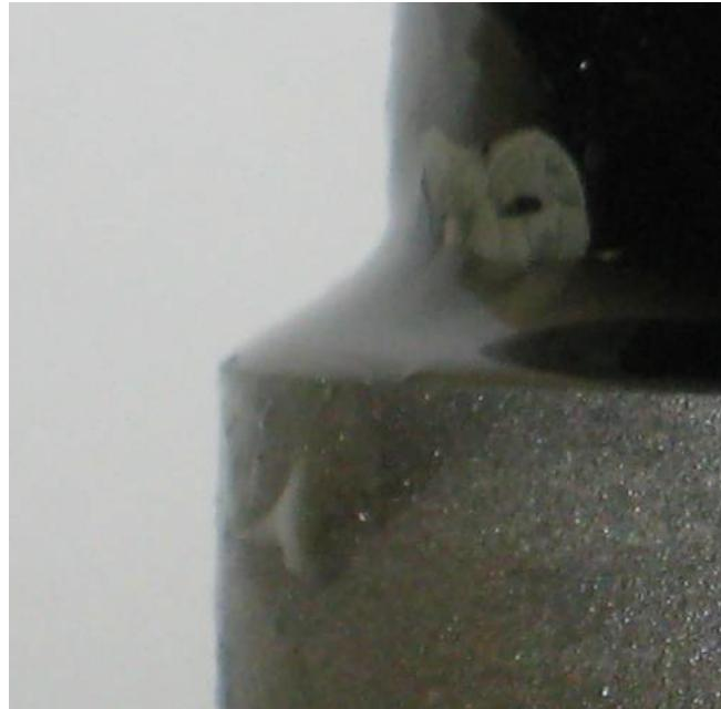
Figure 2-30: Cold-cure epoxy profile used for potting specimens
