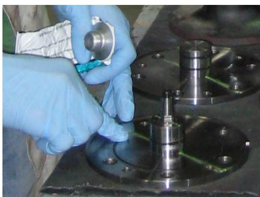
Figure 2-11: Vacuum grease is applied to the o-rings
