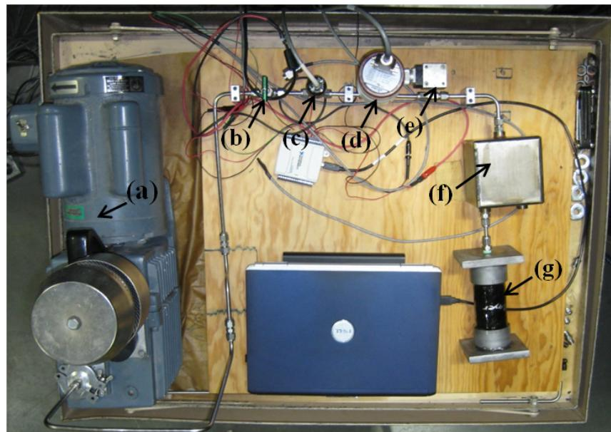
Figure 2-22: Top view of the components of the equipment cart, including the (a) mechanical vacuum pump, (b) valve, (c) thermocouple gauge, (d) capacitance manometer, (e) differential pressure transducer, (f) steel block, and (g) test specimen, in the benchtop testing configuration
