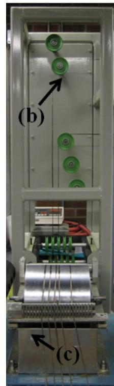
Figure 2-26: The (b) routing system and (c) epoxy bath
