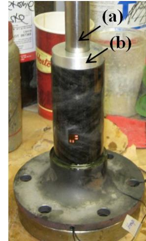
Figure 2-5: The (b) alignment cylinder aligning the 50.8 mm specimen
