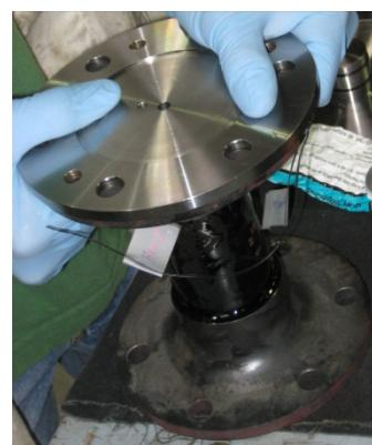
Figure 2-12: The gusset plate is pressed into the supply flange
