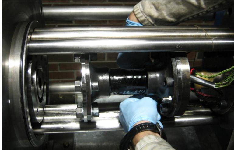
Figure 2-19: The supply side attached to the testing machine.
