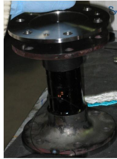
Figure 2-14: The gusset plate is pressed into the passive flange
