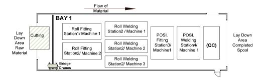
Figure 4.1 A schematic layout drawing of a bay in a pipe spool fabrication shop
