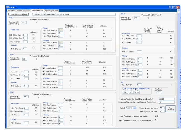
Figure 4.8 User interface for simulation model: revising the layout and shop configurations (inputs to simulation model)
