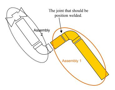
Figure 2.2 Assembly parts of a spool
