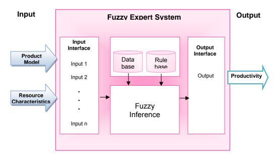
Figure 2.14 The structure of fuzzy expert system
