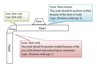
Figure 2.10 Examples of different types of position welds
