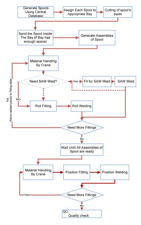
Figure 4.2 Structure of simulation model for case study
