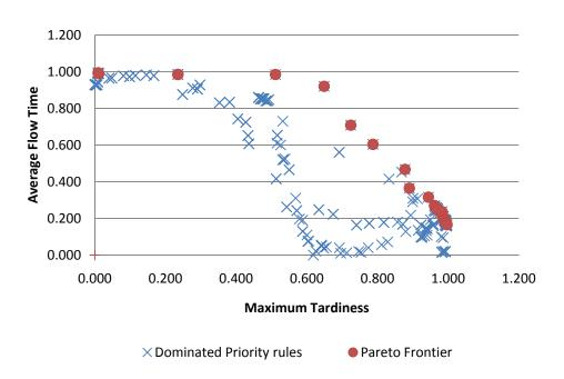
Figure 3.13 Pareto optimal set for a sample scenario
