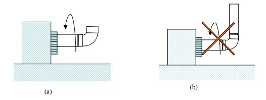
Figure 2.3 Example of roll welding constraint: (a) Roll welding is feasible; (b) Roll welding is not feasible (adopted from Sadeghi and Fayek (2008))
