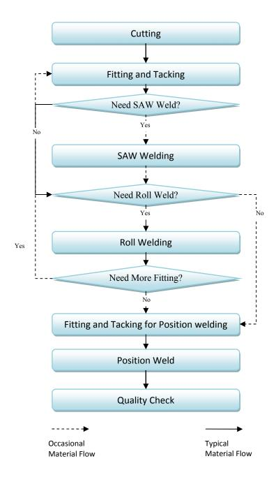
Figure 2.4 Flowchart of pipe spool fabrication process
