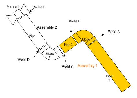
Figure 2.8 Components and assemblies of a spool
