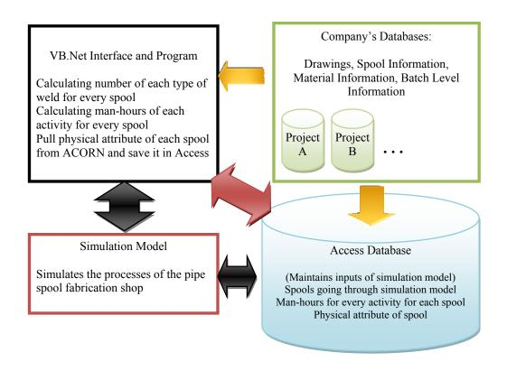
Figure 4.5 Relationships between company's databases and simulation model via VB.net and Access
