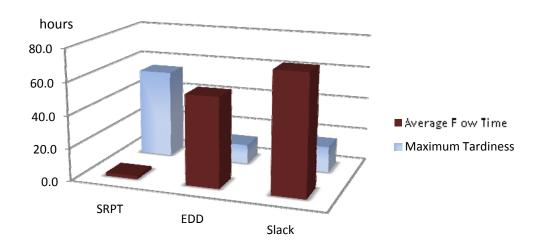
Figure 3.5 Simulation results of applying three simple dispatching rules on a spool fabrication shop (maximum tardiness vs. average flow time)
