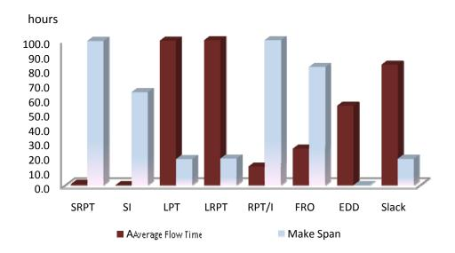
Figure 3.6 Simulation results of applying eight simple dispatching rules on a spool fabrication shop (make-span vs. average flow time)
