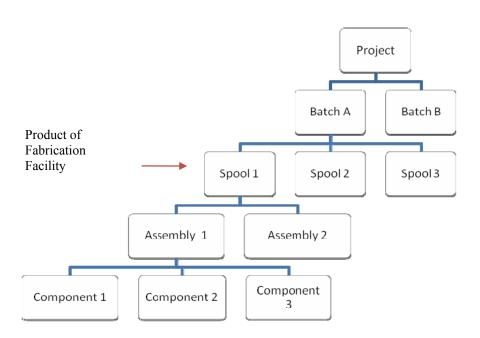
Figure 2.7 Typical work breakdown structure for spool fabrication
