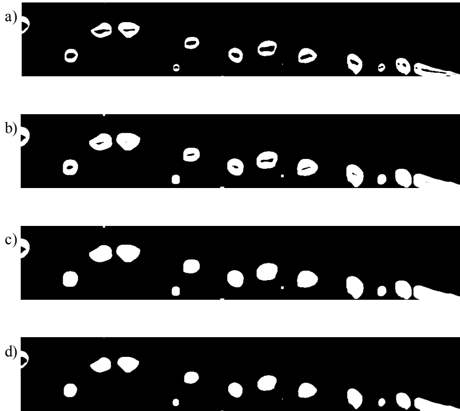
Figure A.3. Description of the steps followed during the filtering process of the image: a) contrast adjusted image, b) dilated image, c) Filling of the black areas within the objects, d) eroded image
