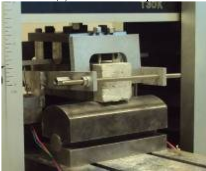
(c) Prism test setup
