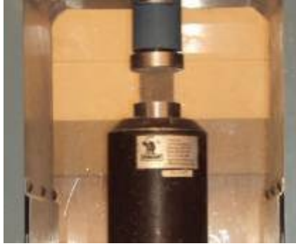
(a) Cube test setup
