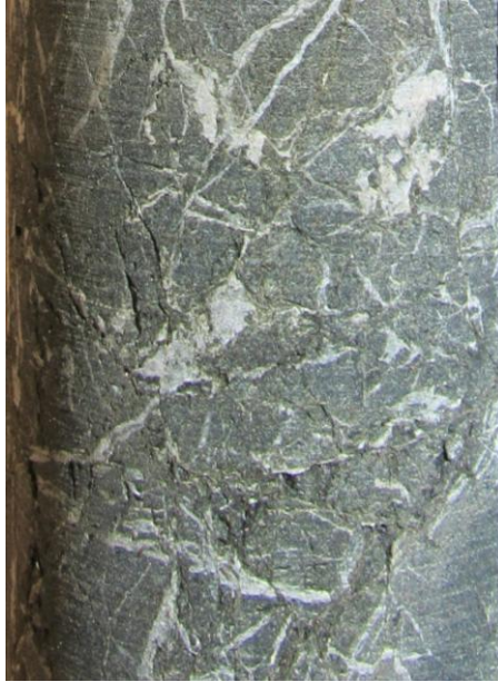
Figure 5-9: Example of the randomly distributed flaws in a 76-mm-diameter drill core.
