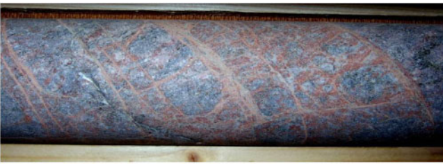
Figure 10. Example of micro-defects in 51 mm core diameter.
