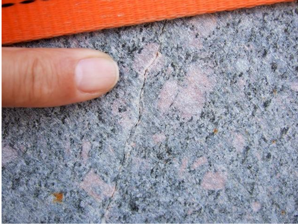
Figure 6-17: Example of the irregular interlocking geometry of a natural fracture.
