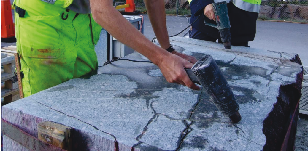
Figure 6-14: Example of the initial stage in detailed mapping process used to identify the fractures.
