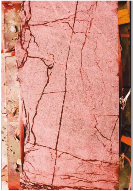
Figure 6-15: Photos of block fracture pattern and the resulting digital mapping.
