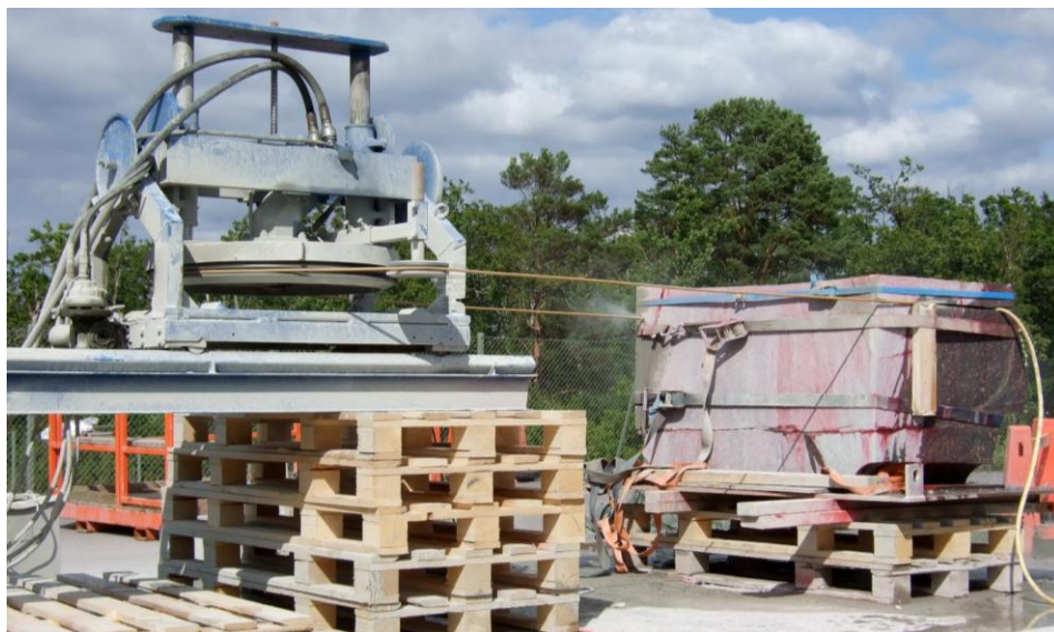
Figure 6-13: Wire sawing of the blocks into 100-mm-thick slabs.
