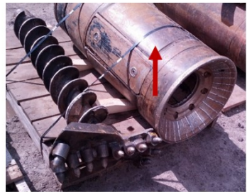
The steering shoe located on the top of the Eliminator
