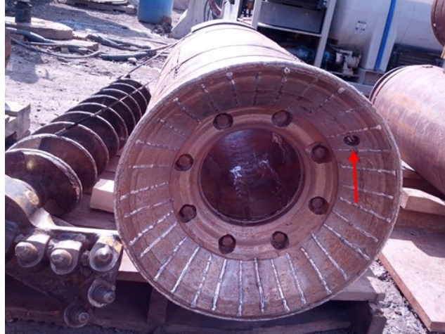
Figure 2.14. Jetting nozzle at the face of the Eliminator
