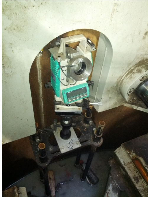
Figure 2.12. Camera mounted on a theodolite in the launch shaft
