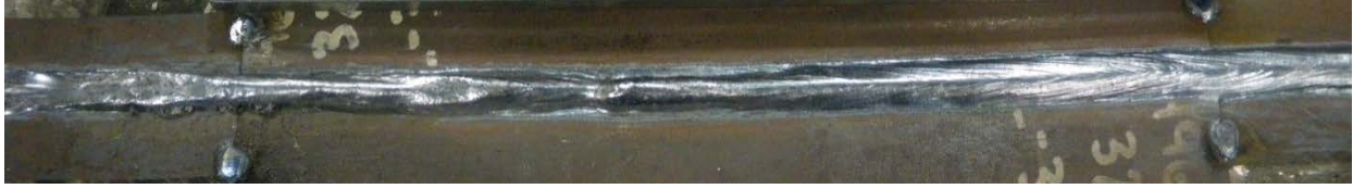
Figure 4.11: Instrumented weld produced with only 6 type K thermocouples embedded.
