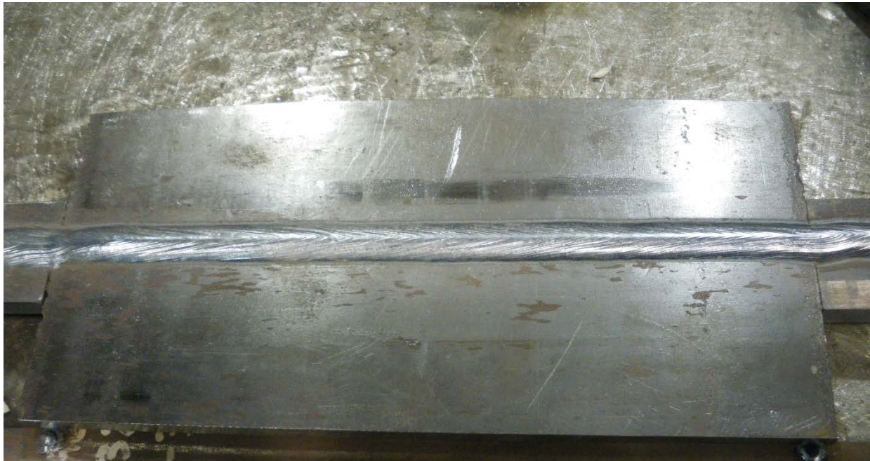
Figure 4.1: Picture of the BOP weld.
