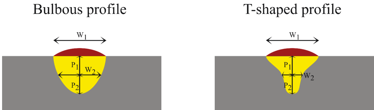
Figure B.6: Schematic explaining how the semi-penetration ratio can help characterize a weld. Inspired by [11].
