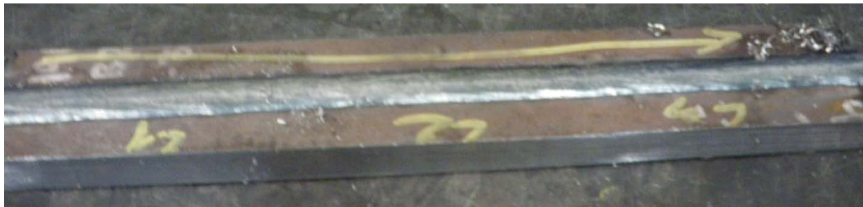
Figure 4.4: Image of the weld performed on the machined plate without thermocouples.
