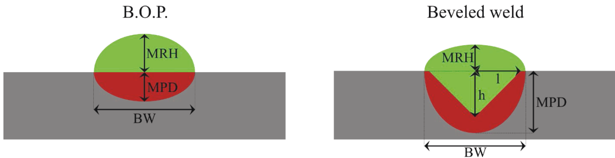
Figure A.6: Schematic illustrating the difference between a BOP weld (left) and a beveled one. The green parts corresponds to the material added during the operation while the red ones corresponds to the material melted.
