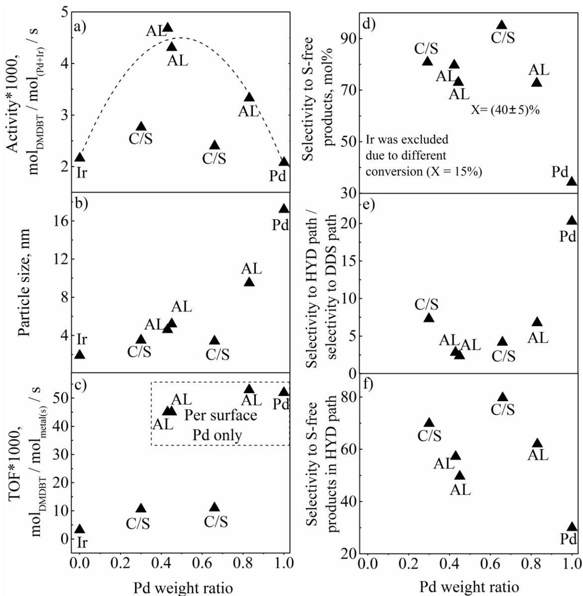
Fig. 5.3. Activity (a), particle size (b), TOF (c), selectivity to sulfur-free products (d), selectivity to HYD path divided by selectivity to DDS path (e) and selectivity to S-free products in HYD path (f) in the HDS of 4,6-DMDBT at 300°C and 5 MPa (WHSV: 30 h<sup>-1</sup>, amount of catalyst: 0.09 g).
