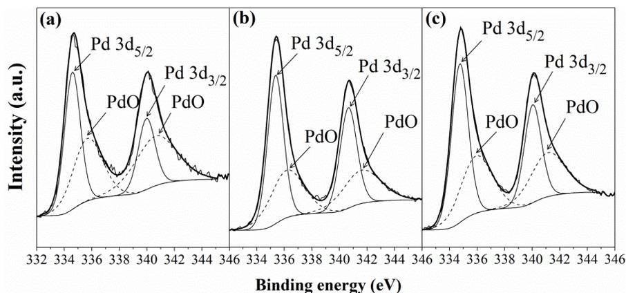
Fig. 2.6. Pd 3d XPS spectra of the selected  $\gamma$ -Al<sub>2</sub>O<sub>3</sub>-supported catalysts: (a) Pd, (b) Pd1Ir1 and (c) Pd(c)Ir(s).
