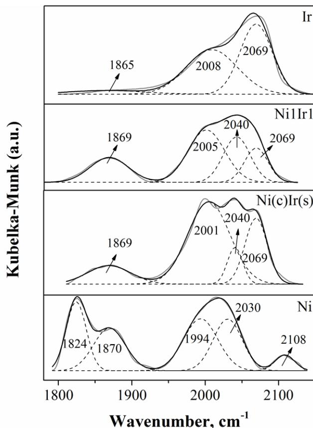
Figure 4.5. DRIFT spectra of the adsorbed CO.
