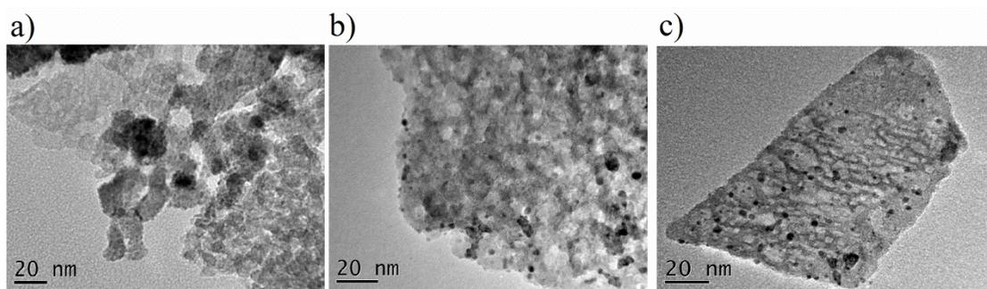
Fig. 3.3. TEM images of selected  $\gamma$ -Al<sub>2</sub>O<sub>3</sub> supported catalysts after calcination at 400°C for 2 h: (a) Pd, (b) Ir and (c) Pd(c)Ir(s) [1/1].
