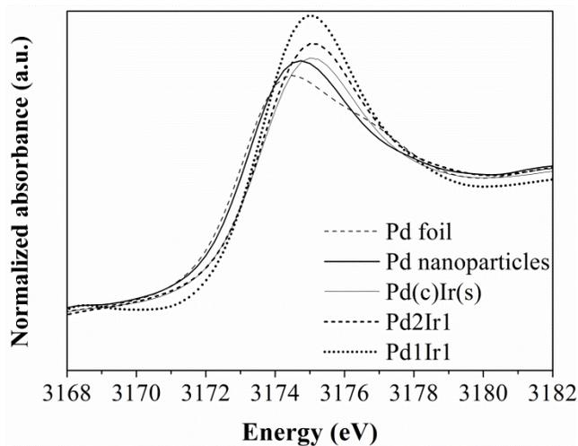
Fig. 2.9. Pd L<sub>3</sub>-edge XANES spectra of the selected nanoparticles supported on  $\gamma$ -Al<sub>2</sub>O<sub>3</sub>. Pd foil was used as the reference.
