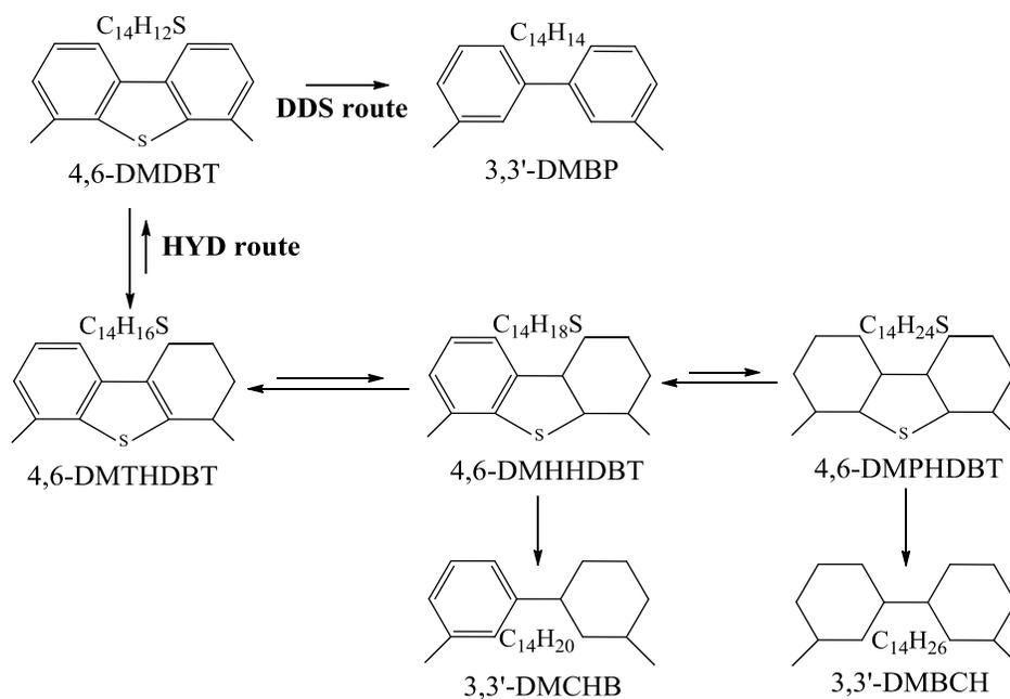
Figure 1.8. The DDS and HYD reaction pathways in the HDS of 4,6-DMDBT at 300°C and 5 MPa.
