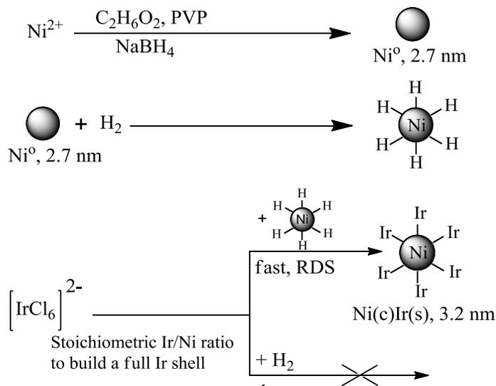
Scheme 4.1. Formation of Ni(c)Ir(s) nanoparticles by hydrogen-sacrificial method.
