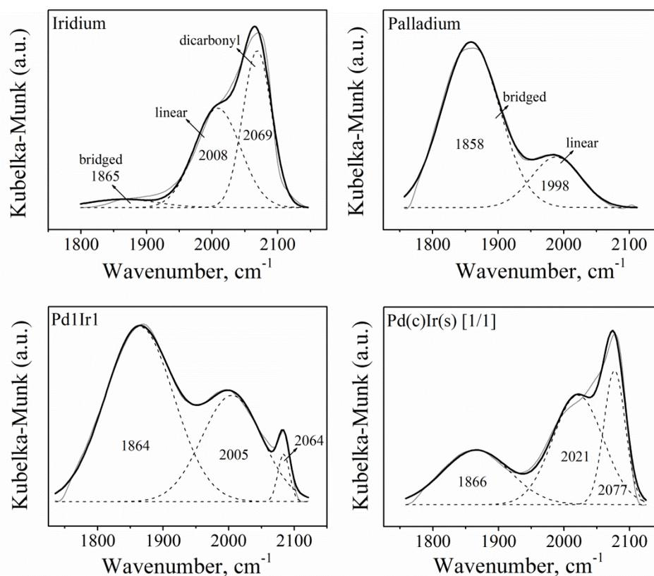
Fig. 3.4. CO-DRIFT spectra for selected samples after calcination and reduction at  $400^{\circ}\text{C}$  (PVP/metal(s) molar ratio of 5:1 used initially for synthesis).
