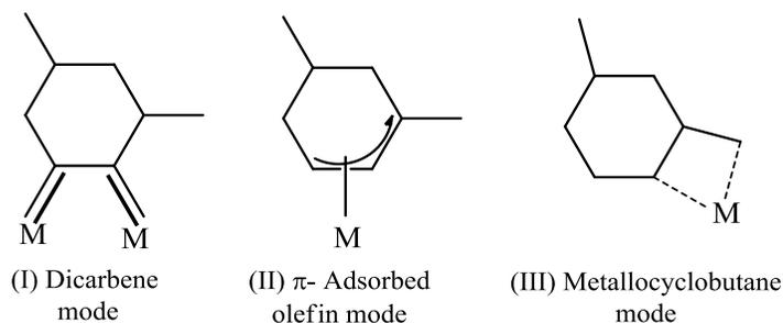
Figure 1.6. A schematic representation of possible reaction mechanisms for ring opening reaction.
