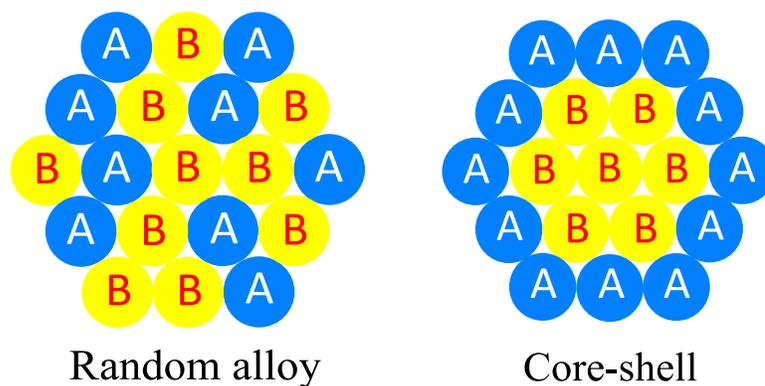
Figure 1.4. Possible structures of bimetallic nanoparticles synthesized by colloidal methods.
