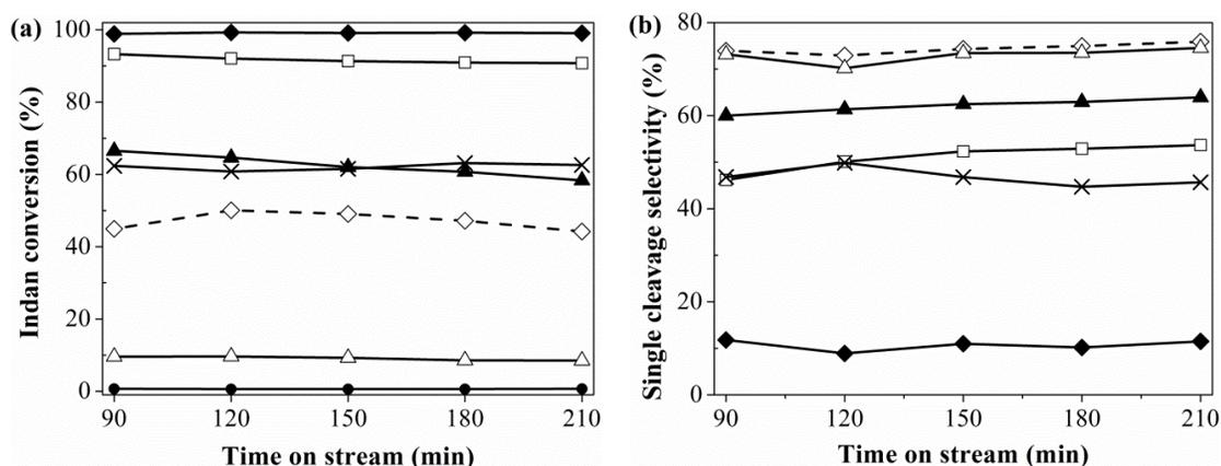
Fig. 2.10. Indane conversion (a) and single cleavage selectivity (b) vs. time-on-stream over different  $\gamma\text{-Al}_2\text{O}_3$ -supported nanoparticles at 336°C and 0.1 MPa: Pd nanoparticles (●), Ir nanoparticles (◆), Ir nanoparticles (half amount) (◇), Pd<sub>2</sub>Ir<sub>1</sub> (Δ), Pd<sub>1</sub>Ir<sub>1</sub> (▲), Pd(c)Ir(s) (□), and industrial Pt-Ir catalyst (×).
