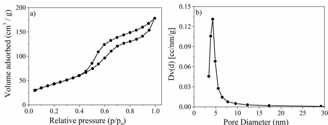
Fig. 5.1. Nitrogen adsorption-desorption isotherm (a) and pore size distribution profile (b) of  $\gamma\text{-Al}_2\text{O}_3$  calcined in air at  $400^\circ\text{C}$ .
