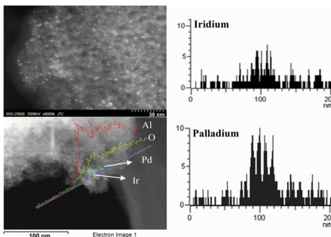
Fig. 2.4. The STEM image with Pd and Ir EDX profiles of the Pd(c)Ir(s) nanoparticle supported on  $\gamma\text{-Al}_2\text{O}_3$ .
