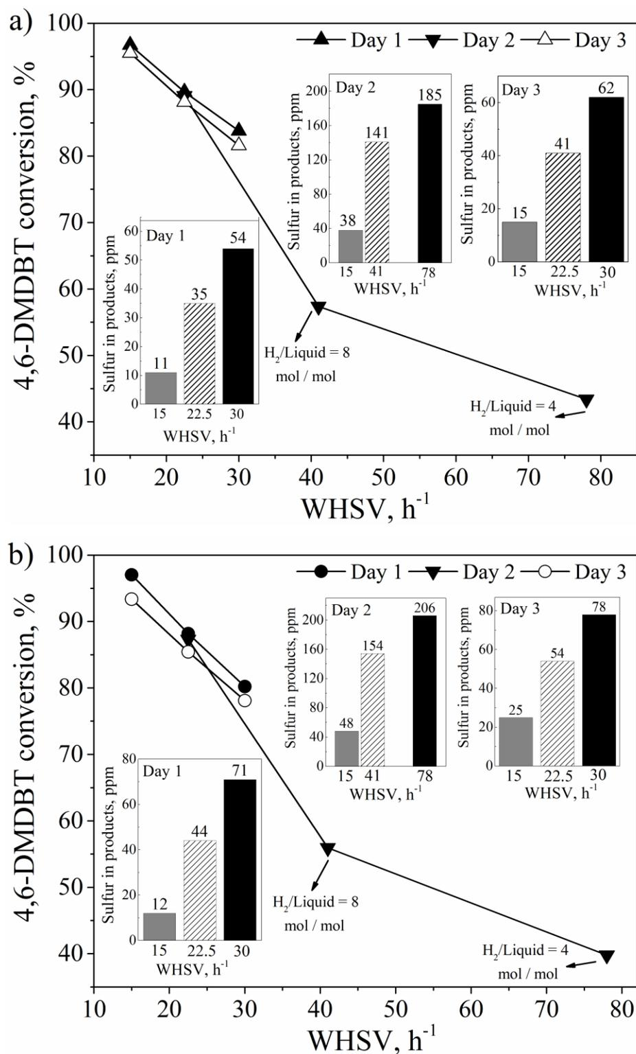
Fig. 5.5. Conversion of 4,6-DMDBT and total sulfur in the final products at various operating conditions over a) Pd66Ir34 (C/S) and b) Pd83Ir17 (AL) supported catalysts (H<sub>2</sub> / liquid: 16 mol / mol, unless indicated on the graphs).
