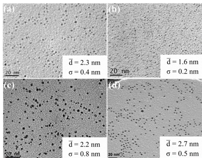
Fig. 2.3. TEM images with average size and one standard deviation for the various Pd and Ir containing nanoparticles: (a) Pd, (b) Ir, (c) Pd<sub>2</sub>Ir<sub>1</sub>, and (d) Pd(c)Ir(s). The image for Pd<sub>1</sub>Ir<sub>1</sub> is not shown; the size is  $2.3 \pm 1.0$  nm. The scale bars correspond to 20 nm.
