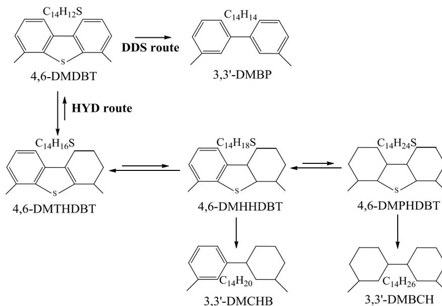
Scheme 5.1. The DDS and HYD reaction pathways in the HDS of 4,6-DMDBT at 300°C and 5 MPa. Reprinted from [24] with permission from Elsevier.
