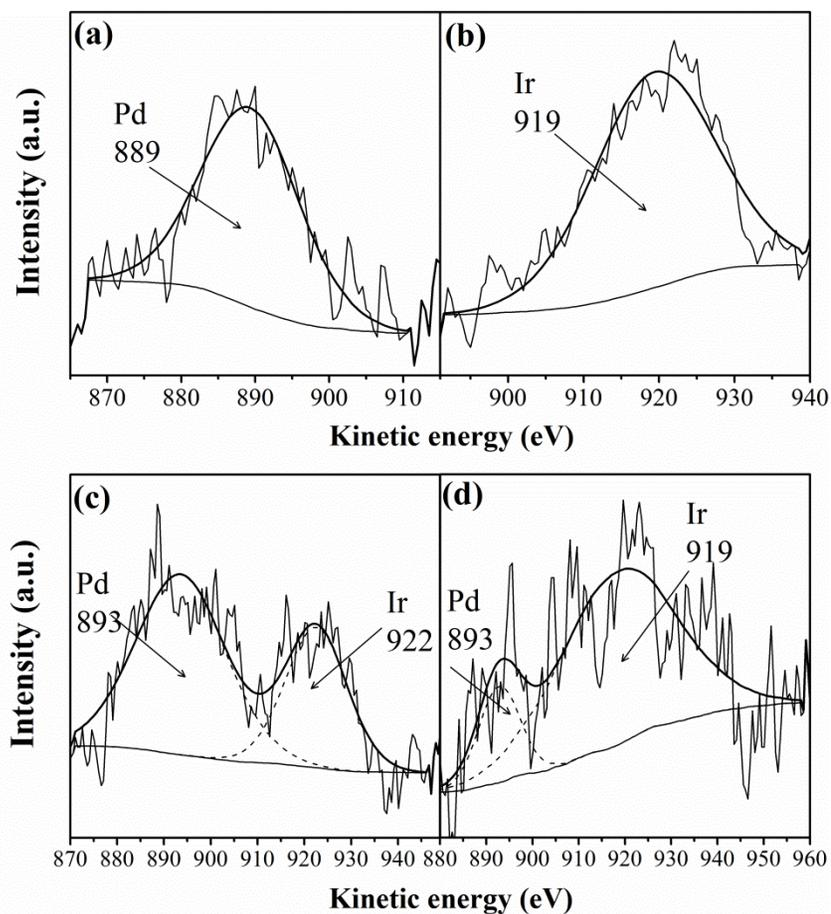
Fig. 2.8. Ion scattering spectra of the selected  $\gamma$ -Al<sub>2</sub>O<sub>3</sub>-supported catalysts: (a) Pd, (b) Ir, (c) Pd1Ir1 and (d) Pd(c)Ir(s).
