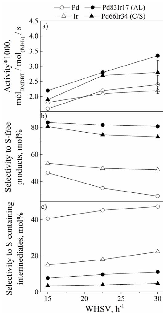
Fig. 5.4. Catalytic activity (a), selectivity to sulfur-free products (b) and selectivity to sulfurous intermediates (c) in the HDS of 4,6-DMDBT over selected supported catalysts at different WHSV values at 300°C and 5 MPa (H<sub>2</sub> / liquid: 16 mol / mol).
