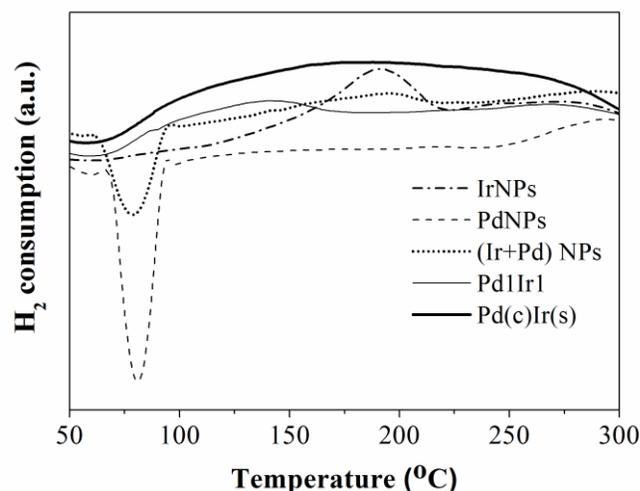
Fig. 2.5. H<sub>2</sub>-TPR profiles of the selected catalysts in 10 ml/min mixture of 10% H<sub>2</sub> in Ar (heating rate: 5°C/min).
