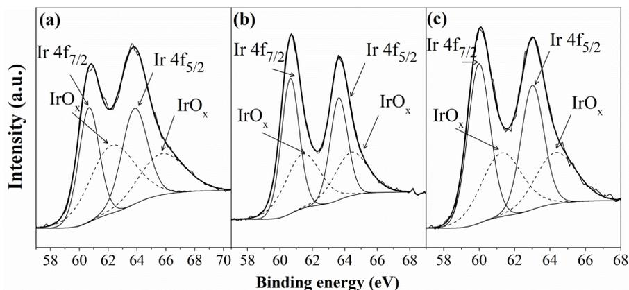
Fig. 2.7. Ir 4f XPS spectra of the selected  $\gamma$ -Al<sub>2</sub>O<sub>3</sub>-supported catalysts: (a) Ir, (b) Pd1Ir1 and (c) Pd(c)Ir(s).
