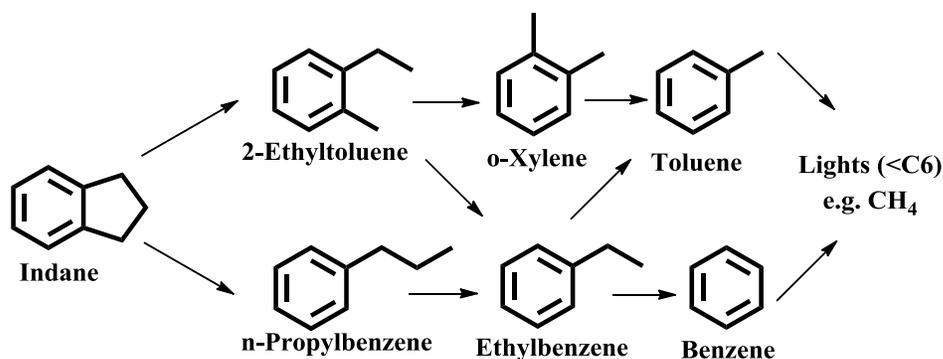
Scheme 2.1. Reaction pathway for the ring opening of indane at atmospheric pressure. Reprinted from [37] with permission from Elsevier<sup>1</sup>.
