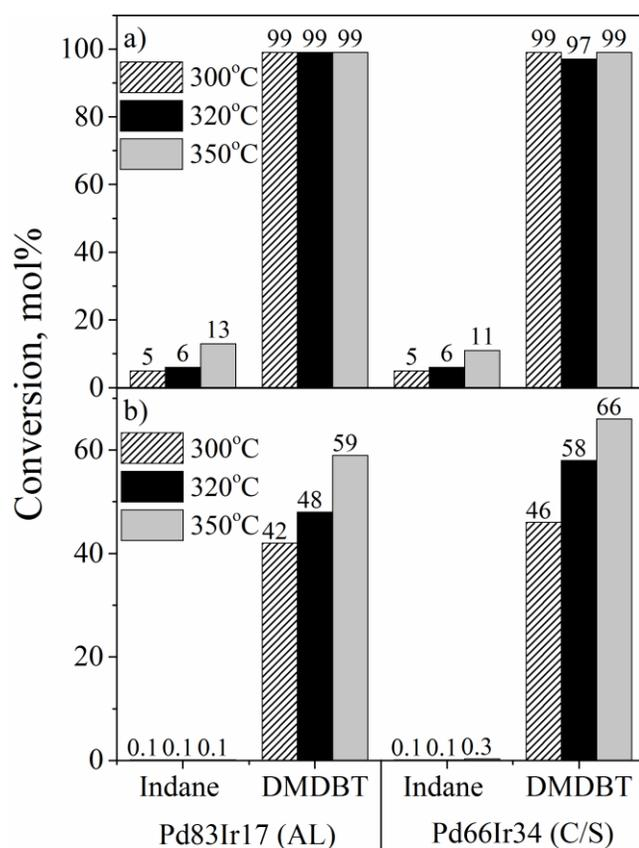
Fig. 5.8. Catalytic conversion of a mixture including: 2 wt.% indane and 300 ppm sulfur as 4,6-DMDBT at various temperatures and 5 MPa over selected catalysts: a) WHSV:  $8.5 \text{ h}^{-1}$ ,  $\text{H}_2$  / liquid: 16 mol / mol, and b) WHSV:  $45 \text{ h}^{-1}$ ,  $\text{H}_2$  / liquid: 4 mol / mol. (Note: metal loadings are different: 0.233 wt.% Pd and 0.047 wt.% Ir in Pd83Ir17, as well as 0.259 wt.% Pd and 0.131 wt.% Ir in Pd66Ir34).
