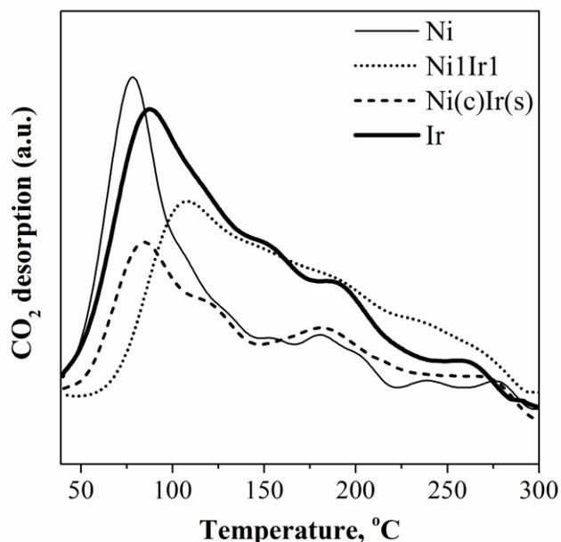
Figure 4.4. CO<sub>2</sub>-TPD profiles of selected  $\gamma$ -Al<sub>2</sub>O<sub>3</sub> supported catalysts, after subtraction of the TPD data for the support.
