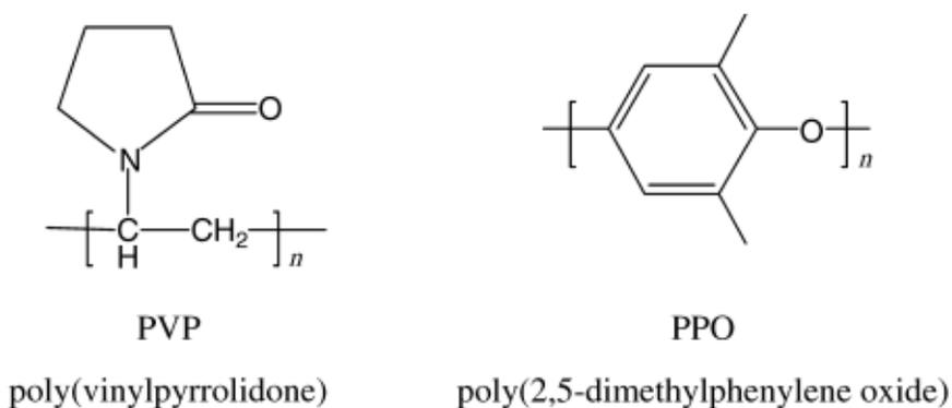
Figure 1.2. Schematic structure of PVP and PPO polymeric stabilizers. Reprinted from [41] with permission of John Wiley and Sons (© 2005 WILEY-VCH Verlag GmbH & Co. KGaA, Weinheim).
