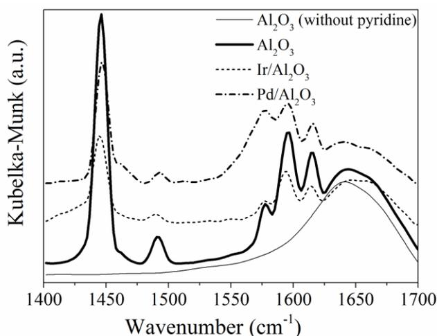
Fig. 5.2. DRIFT spectra of adsorbed pyridine on  $\gamma\text{-Al}_2\text{O}_3$  and selected  $\gamma\text{-Al}_2\text{O}_3$  supported catalysts.
