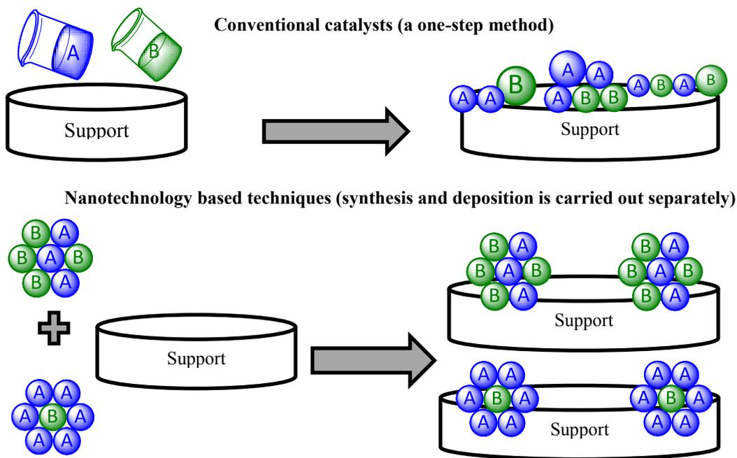
Figure 1.1. A schematic representation of impregnation and nanotechnology based techniques in synthesis of bimetallic supported catalysts.
