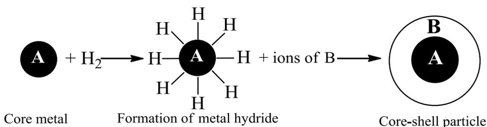
Figure 1.5. Schematic presentation of hydrogen sacrificial reduction method for synthesis of core-shell nanoparticles.
