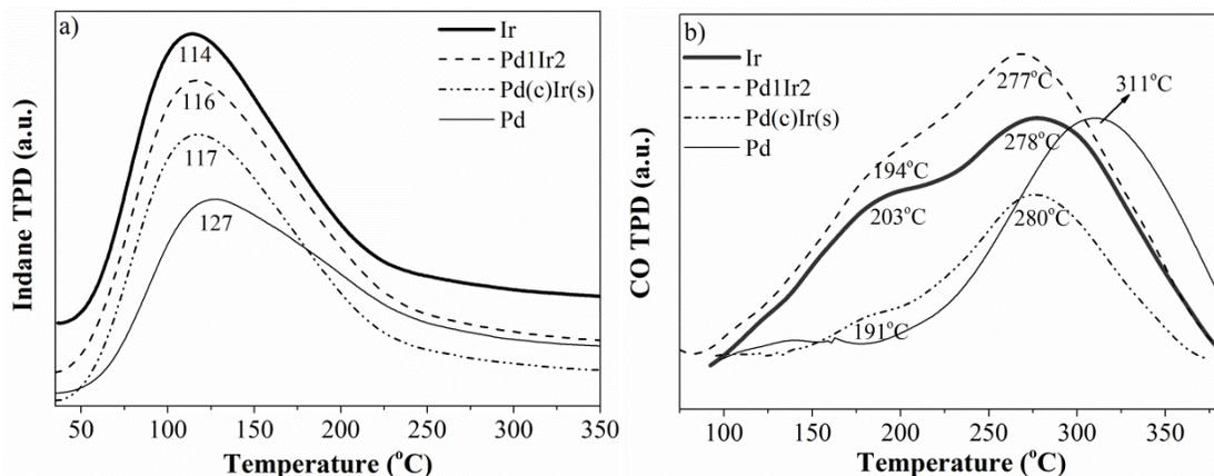
Fig. 3.6. TPD profiles at various heating rates for supported Ir catalysts after calcination and reduction at 400°C: (a) indane-TPD and (b) CO-TPD.
