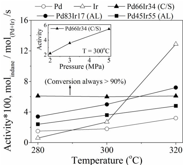
Fig. 5.7. Catalytic activity in high pressure hydrogenation over selected catalysts at various temperatures and 5 MPa (WHSV: 45 h<sup>-1</sup>, H<sub>2</sub> / liquid: 4 mol /mol). Inset shows the activity of Pd66Ir34 (C/S) at 300°C and various pressures.
