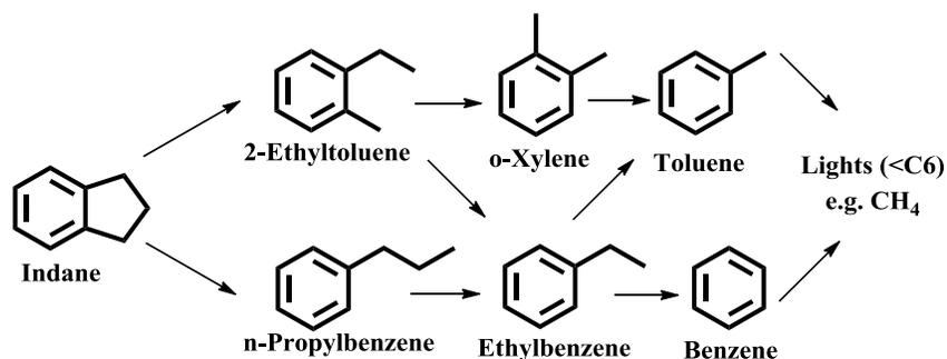
Figure 1.7. Reaction pathway for the ring opening of indane at atmospheric pressure. Reprinted from [4] with permission from Elsevier.
