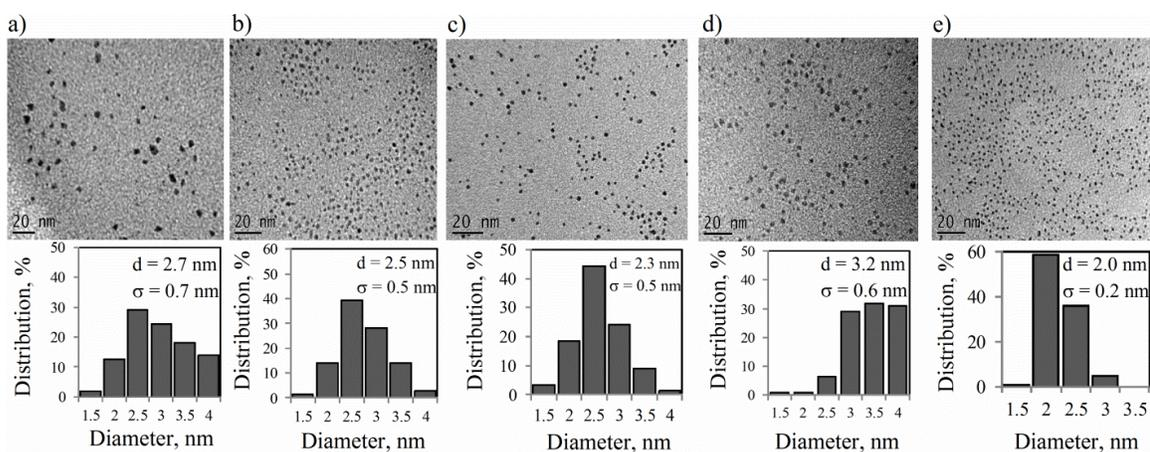
Figure 4.2. Size distribution histograms and the corresponding TEM images: (a) Ni, (b) Ni<sub>2</sub>Ir<sub>1</sub>, (c) Ni<sub>1</sub>Ir<sub>1</sub>, (d) Ni(c)Ir(s) and (e) Ir.
