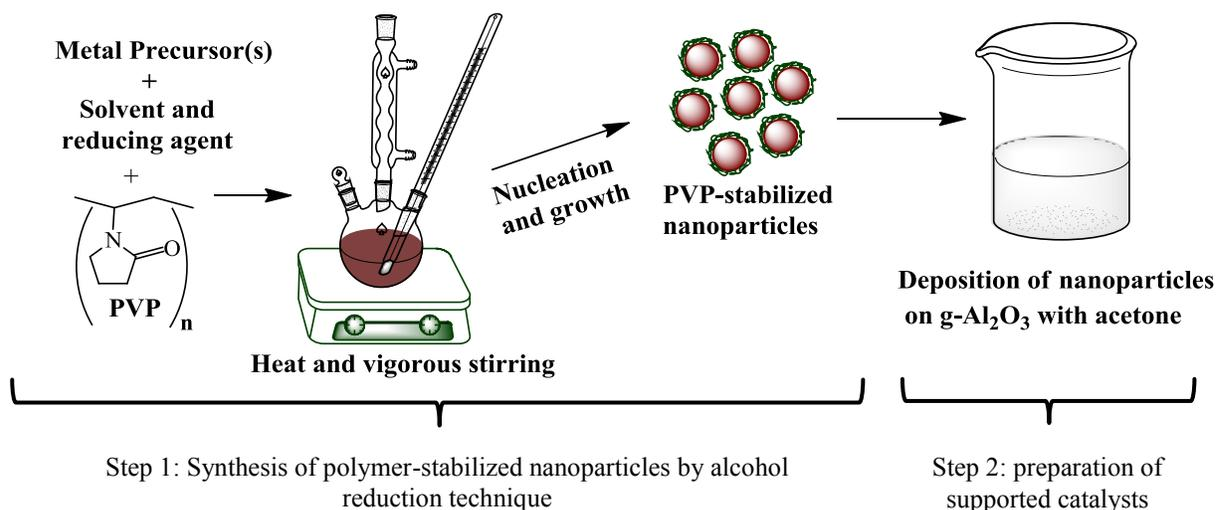
Figure 1.3. Schematic presentation of nanoparticles formation, and deposition on the support material with acetone.
