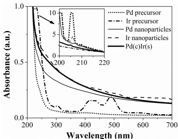
Fig. 2.1. UV-vis spectra of the selected PVP-stabilized nanoparticles and the starting solutions of metal precursors.
