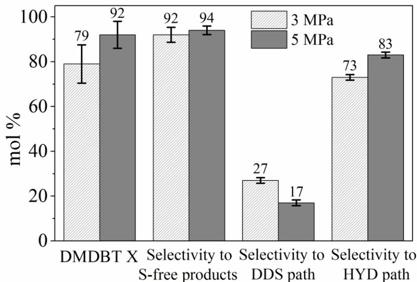
Fig. 5.6. The range of conversions, selectivities to sulfur-free products, DDS and HYD selectivity values in the HDS of 4,6-DMDBT over Pd66Ir34 (C/S) catalyst at 300°C and different pressures for WHSV's of 15, 22.5 and 30 h<sup>-1</sup>, H<sub>2</sub> / liquid: 16 mol / mol.
