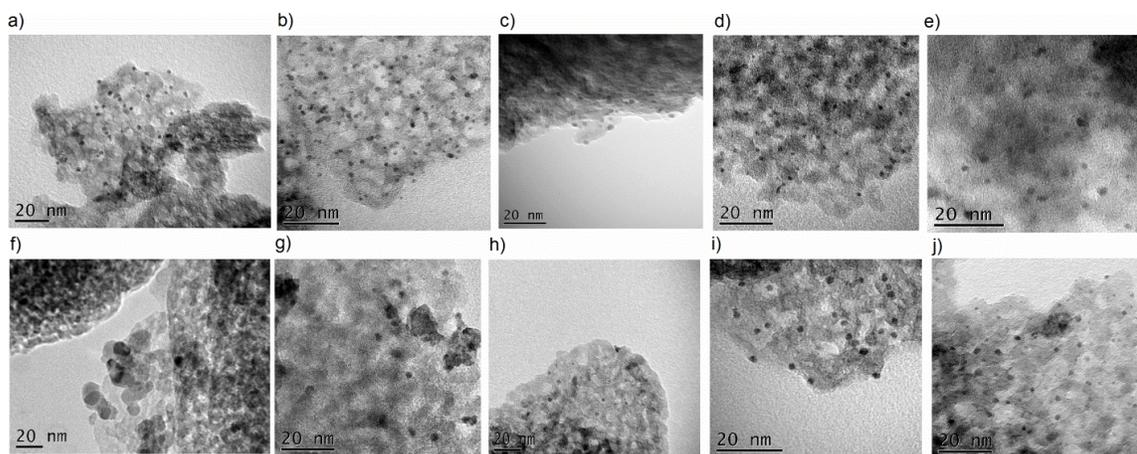
Figure 4.6. TEM images of the fresh (top column) and calcined (2 h, 400°C; bottom column) supported catalysts: (a, f) Ni, (b, g) Ni<sub>2</sub>Ir<sub>1</sub>, (c, h) Ni<sub>1</sub>Ir<sub>1</sub>, (d, i) Ni(c)Ir(s) and (e, j) Ir.
