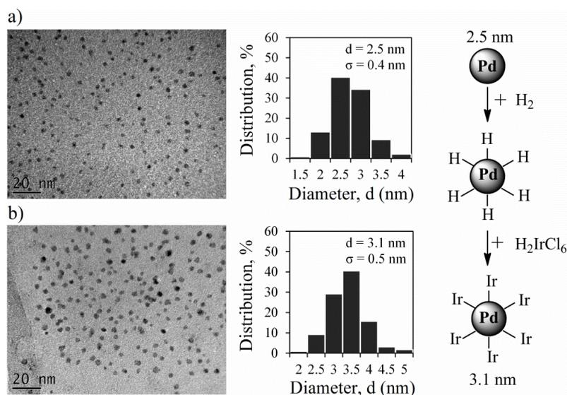
Fig. 3.1. TEM images and size distribution histograms of as-synthesized nanoparticles and their formation schematic: (a) Pd and (b) Pd(c)Ir(s) [1/1] (PVP/metal(s) molarratio = 5:1).
