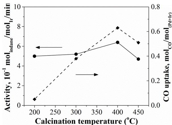
Fig. 3.5. Ring opening catalytic activity and CO uptake of supported Pd(c)Ir(s) [1/1](PVP/metal(s) molar ratio = 5:1) after various thermal treatments.
