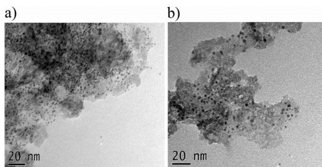
Fig. 3.2. TEM images of selected  $\gamma$ -Al<sub>2</sub>O<sub>3</sub> supported catalysts after calcination at 200°C for 1 h: (a) Ir and (b) Pd(c)Ir(s) [1/1] (PVP/metal(s) molar ratio of 5:1).
