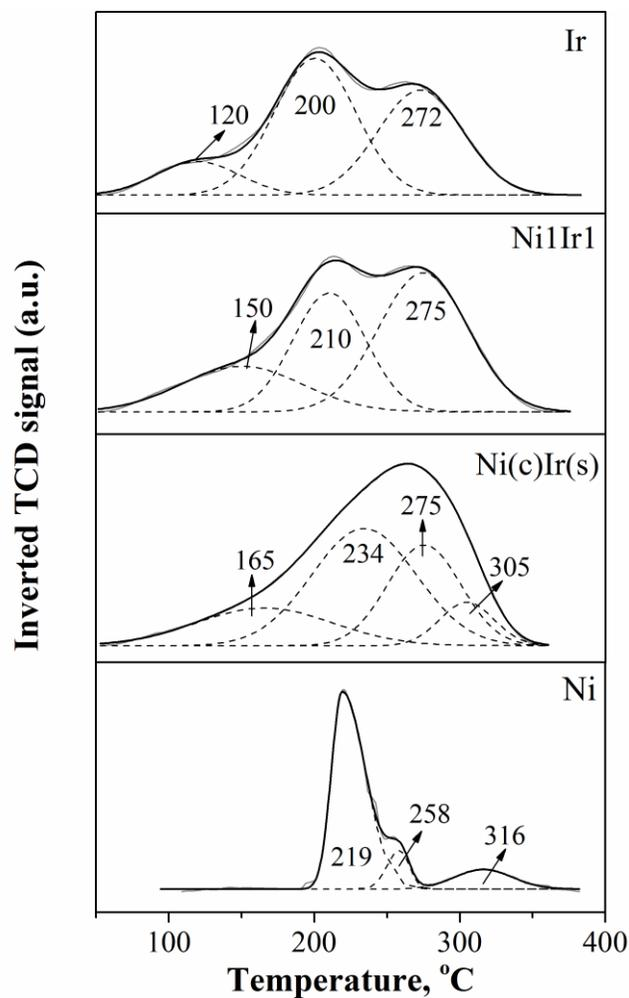
Figure 4.3. H<sub>2</sub>-TPR profiles of the selected  $\gamma$ -Al<sub>2</sub>O<sub>3</sub> supported catalysts. Positive inverted TCD signal indicates hydrogen consumption in H<sub>2</sub>/Ar mixture.
