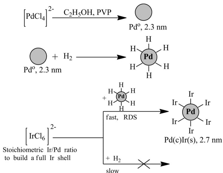
Scheme 2.2. Formation of Pd(c)Ir(s) nanoparticles by hydrogen-sacrificial reduction method.
