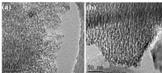
Fig. 2.11. TEM photographs of (a) Ir/ $\gamma$ -Al<sub>2</sub>O<sub>3</sub> after the reaction, 210 min on stream; (b) Pd(c)Ir(s)/ $\gamma$ -Al<sub>2</sub>O<sub>3</sub> after the reaction, 210 min on stream.
