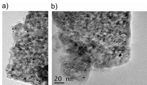
Figure 4.7. TEM images of Ni1Ir1 catalyst: (a) before the catalytic reaction (calcined and reduced in-situ) and (b) after the 200 min on stream.
