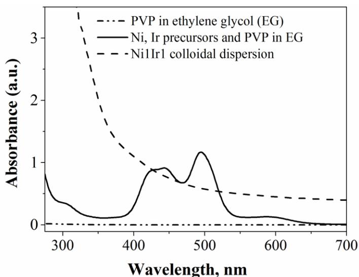
Figure 4.1. UV-vis spectra during the preparation of Ni1Ir1 colloidal dispersion.
