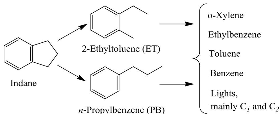
Scheme 4.2. The reaction scheme for ring opening of indane at atmospheric pressure and 350°C.
