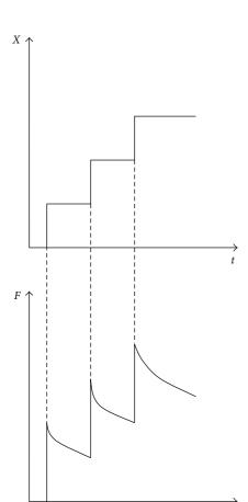
FIGURE 2: Typical force response to a stepwise and discrete generation of displacement for a visoelastic material. Following each idealized step, the tissue relaxes, and observed force decreases based on the relaxation function.
