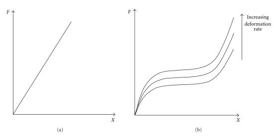
FIGURE 1: Typical force versus displacement characteristics for a linear (a) and a viscoelastic (b) material.
