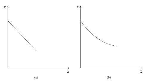
FIGURE 3: Typical force versus displacement curves for spring-type (a) and magnetic (b) activation methods.
