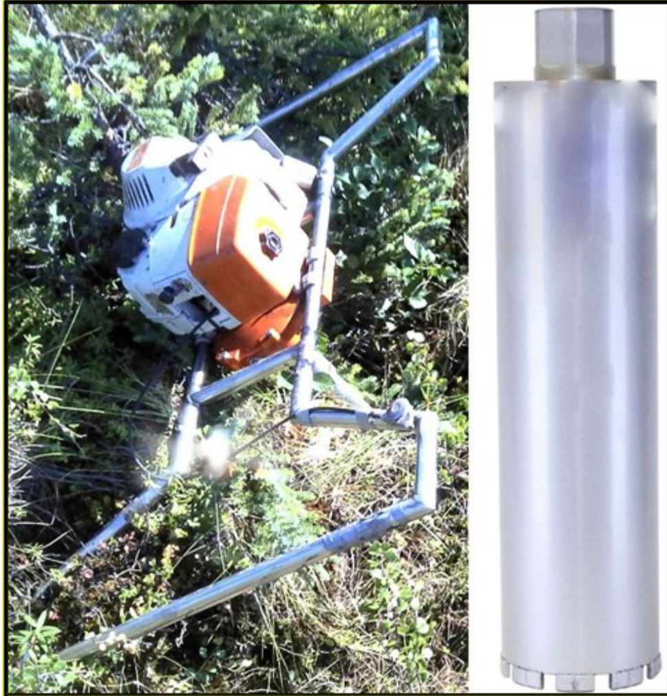
Figure 2.1: Two person operated earth-drill (left) (Calmels et al. 2005) and a 4 inch diameter diamond tooth core barrel used for drilling permafrost cores (right).
