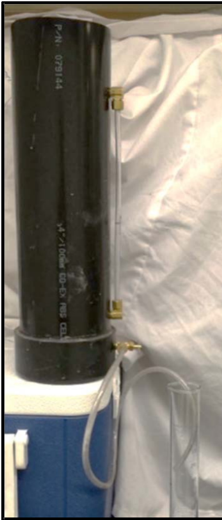
Figure 2.6: PVC tube set for measuring IVC with clear rubber hose attached to the bottom control valve for precise drainage into graduated cylinder.
