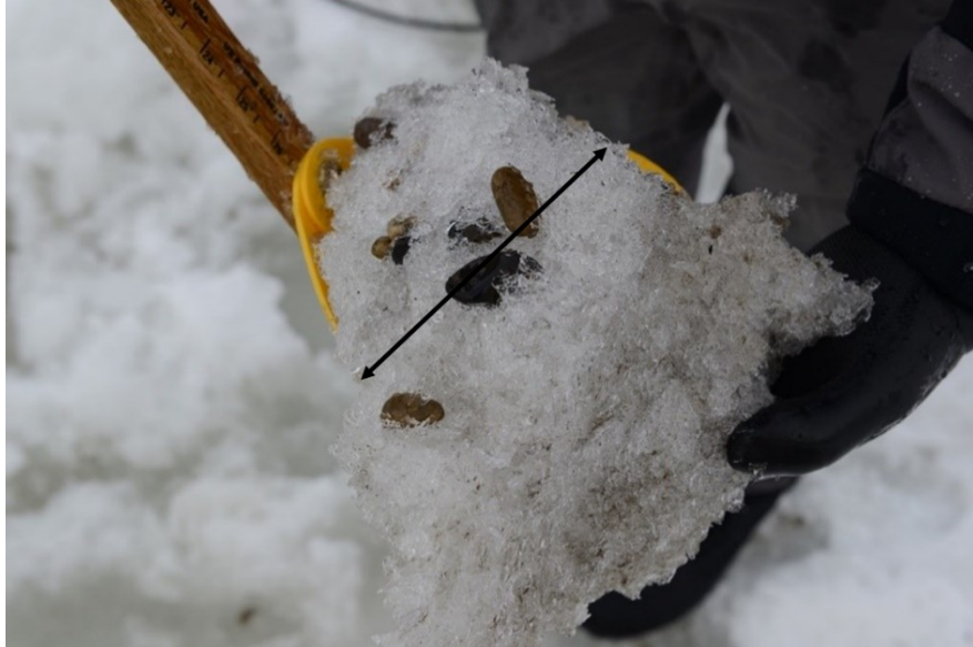
Figure 2-4. Digital image of a drained anchor ice sample collected using an ice scoop, November 28, 2016. The width of the scoop as indicated by the arrow is ~18 cm.
