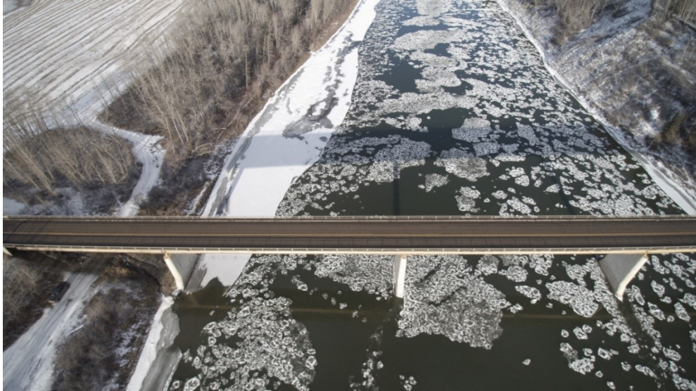
Figure 1-3. Digital image taken on the North Saskatchewan River on December 3, 2016 showing frazil ice pans and larger frazil ice rafts (field of view is ~200 m wide).
