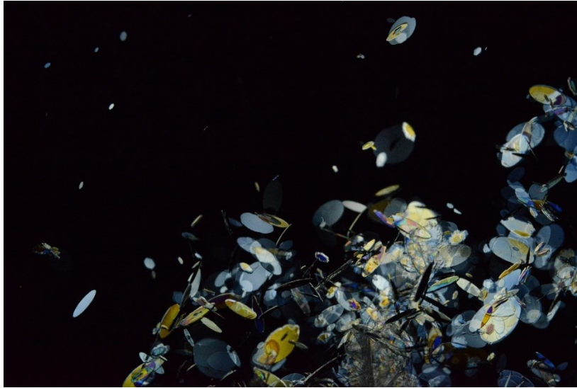
Figure 1-1. Digital image showing typical disc shaped frazil particles and frazil flocs (image courtesy of V. McFarlane) (field of view is ~4.1 cm wide).
