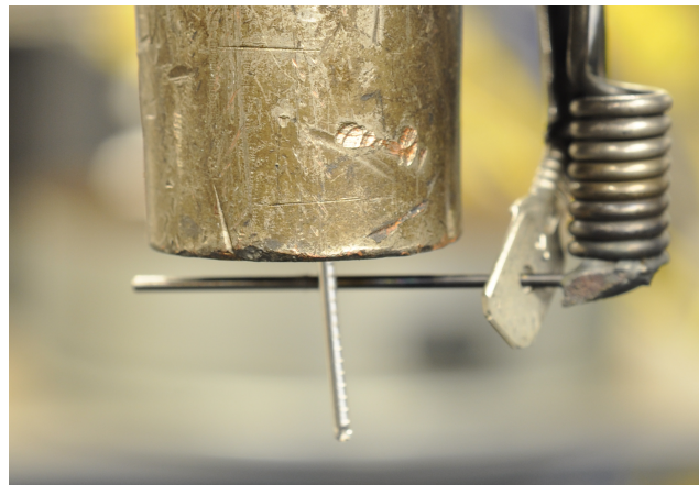
Fig. A.6: Tungsten probe used to measure contact tip voltage loss in aluminum electrode.
