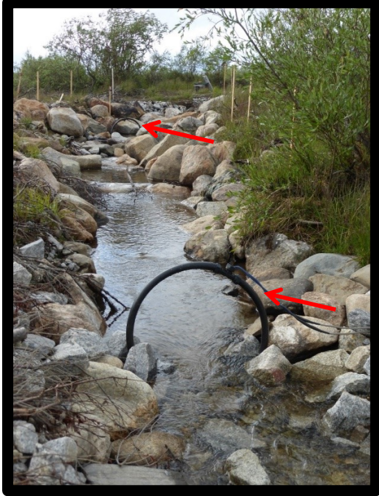
Figure 9. Photograph looking upstream at two pass-through antennas in WIS (red arrows). The closest antenna in the photo is at 25 m upstream of Lac de Gras, while the antenna further upstream and toward the top of the photo is at 36 m upstream.
