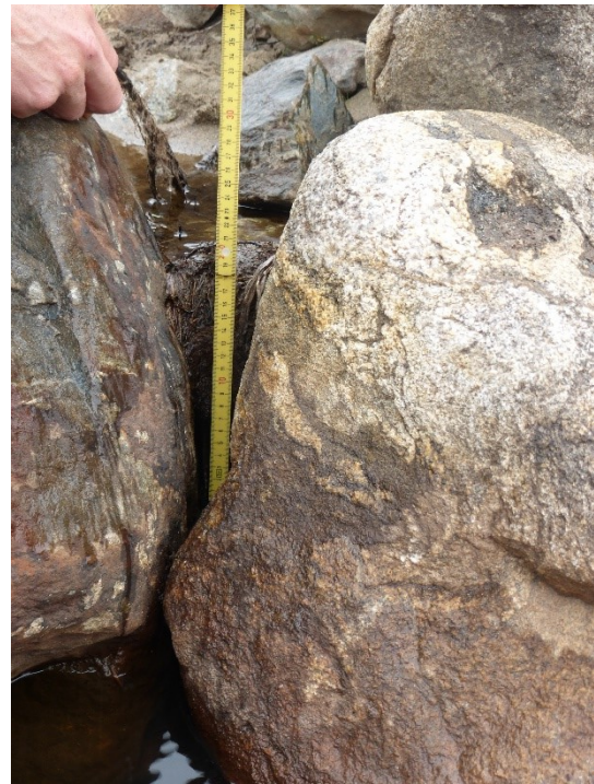
Figure 22. A photograph of the V notch created by the two large boulders, at low summer flow.
