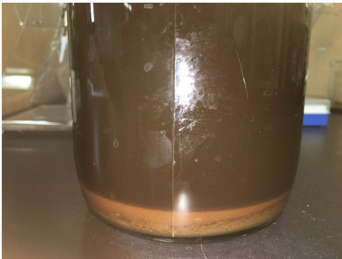
Figure 4-19 Separated layers of brown grease
