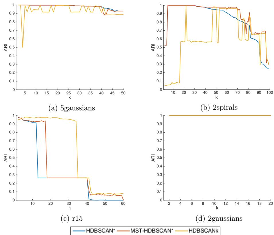
Figure 4.8: ARI values over the range of  $k$  nearest neighbors to consider for HDBSCAN\*, MST-HDBSCAN\* and HDBSCANk.
