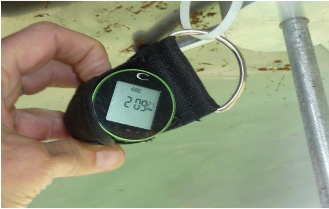
Figure 14. Photograph of Cairclip attached under shelter in backyard setting.
