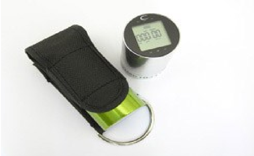
Figure 4. Example of the Cairclip sensor \text{O}_3/\text{NO}_2 used in the study (adapted from Cairpol, 2014).
