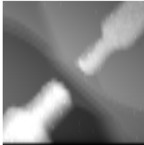
(b) STM image of the gap between the contact pads on low-doped n-type Si(111) (600 nm, -3 V, 100 pA).
