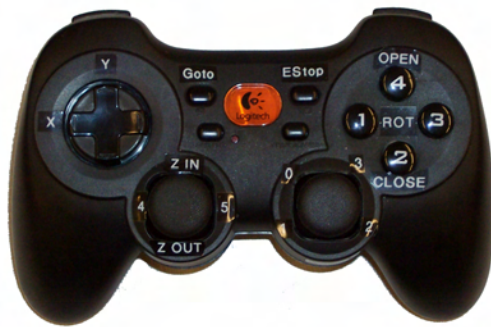
Figure 5.11: Photograph of the wireless gaming controller used to control the pliers.
