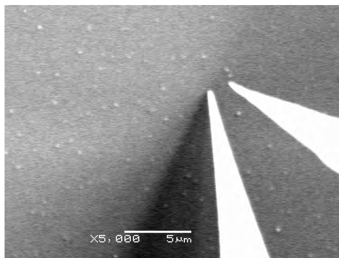
Figure 7.5: SEM image of two STM tips (the right probe and the center STM) brought close to each other over a Si(111) surface with \text{TiSi}_2 islands. 5000 \times magnification, 7 kV beam voltage.
