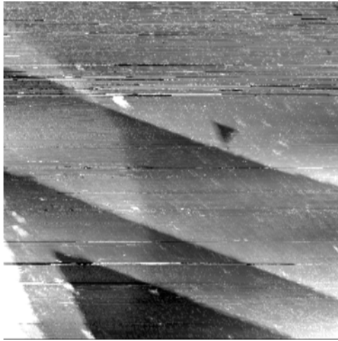
(a) Topography image (200 nm wide). The metal contact is close to the lower left corner. The bright patch is Si(111)-7 \times 7.
