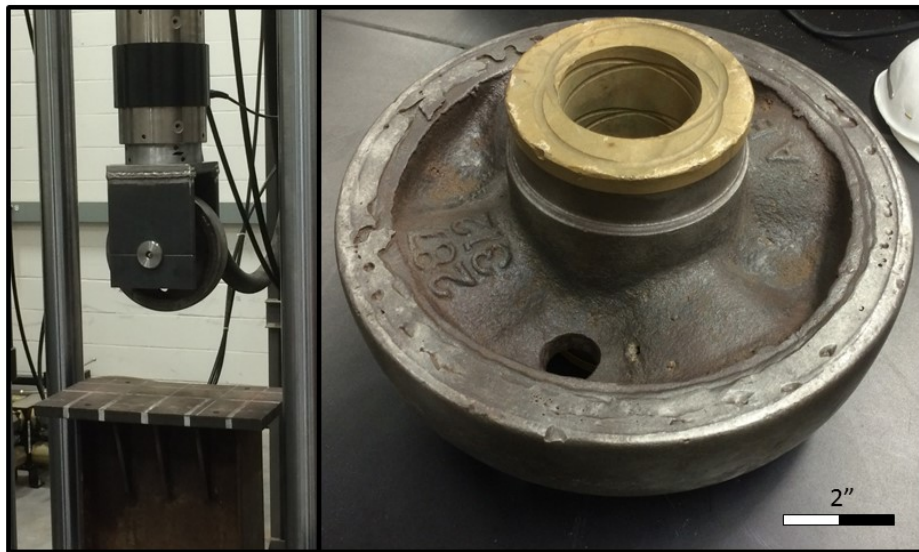
Figure 32: Main load roller; mounted onto the loading frame (left), and isolated (right)
