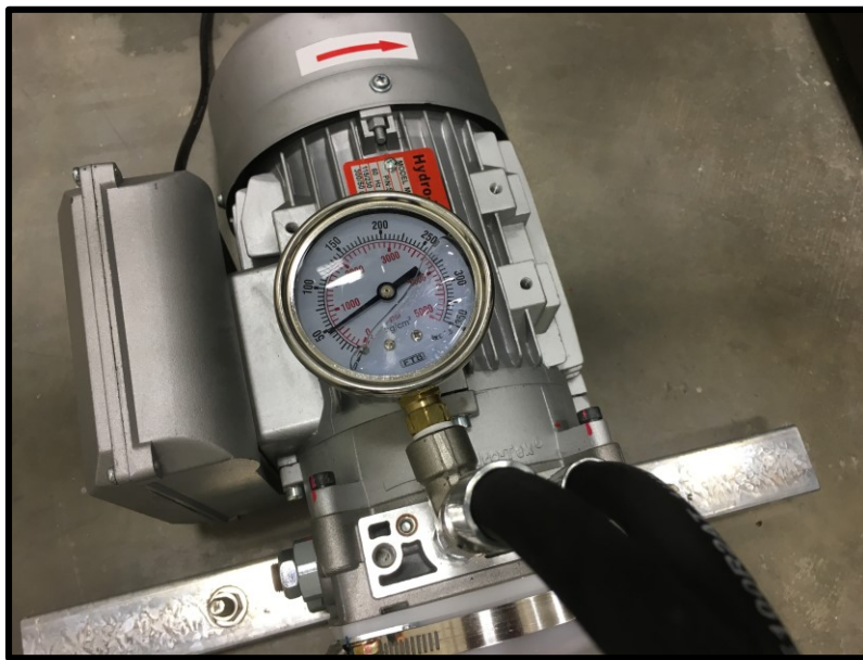
Figure 36: 1 HP Hydro-Tek power unit (pump)
