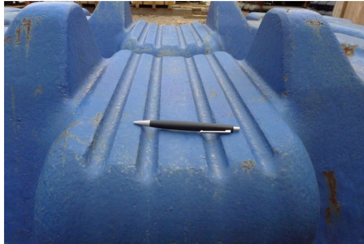
Figure 16: Roller path for high manganese shoes
