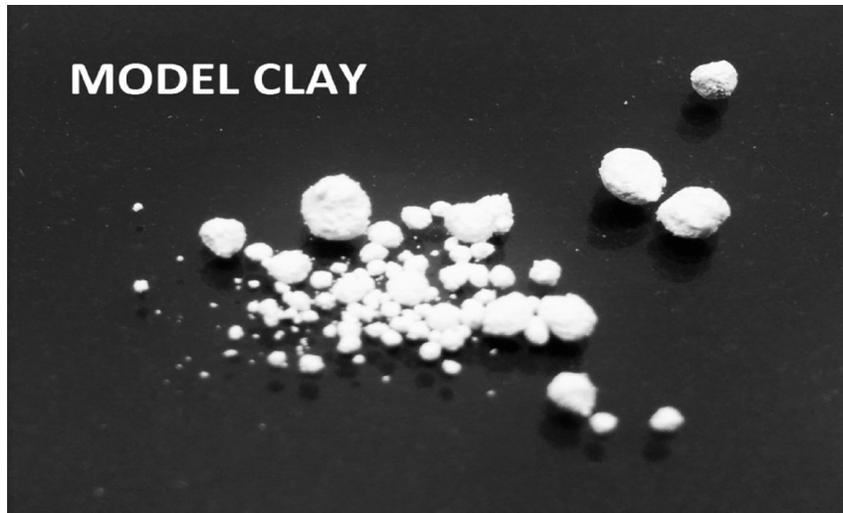
**Figure 3-3: Kaolin (model clay) used to observe the fluorescence intensity difference between bitumen and clay.**
