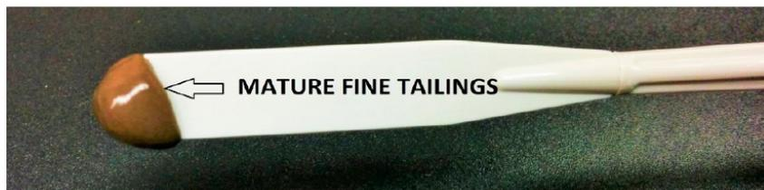
**Figure 3-4: MFT sample from Syncrude tailings pond.**
