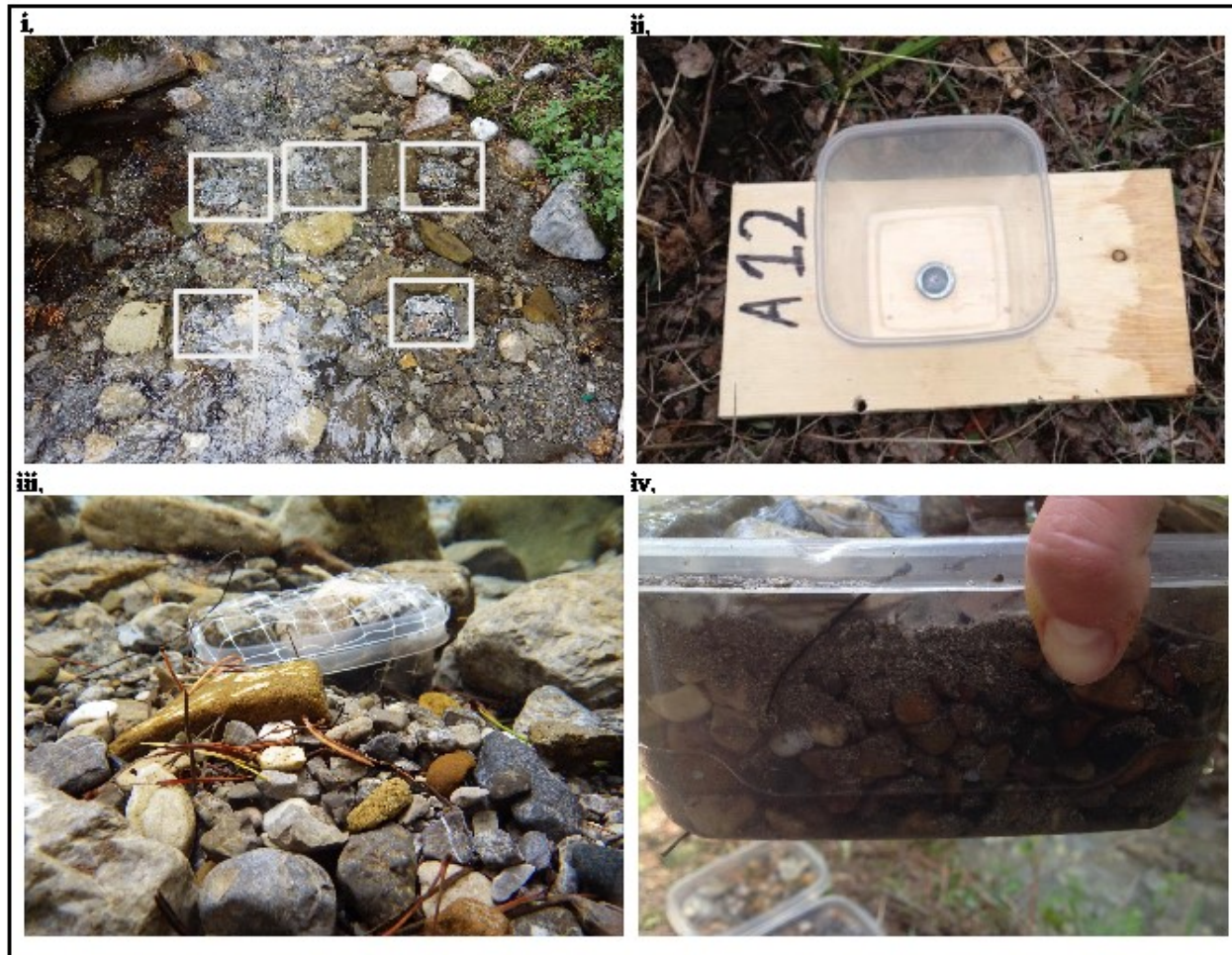
Figure 3-3. Photographs of ingress sediment traps components including: i) typical layout of transects (each consisting of five-sediment ingress traps), ii) out-of-stream plywood-based anchors used to prevent trap loss during high-flow events, iii) nested traps covered with plastic garden mesh and placed flush to streambed, and iv) example of ingress sediment collected within the interstitial void space following 2-3 week deployment.
