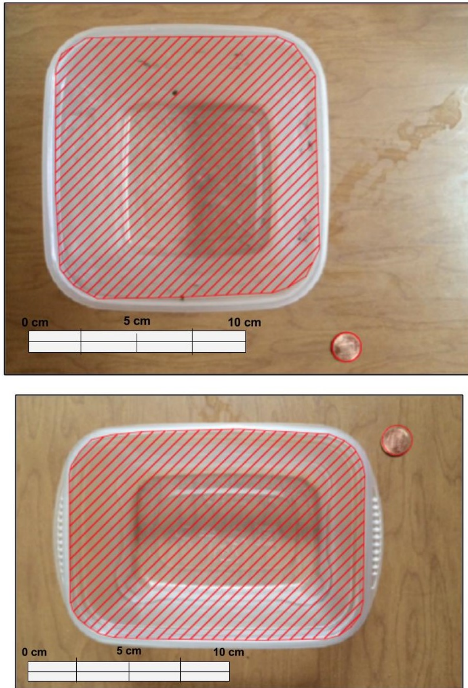
Figure 3-4. Two-sizes of sediment ingress traps were used. Larger sediment traps were utilized in Star West and Star East ( 156.3 \text{ cm}^2 ), while smaller ingress traps ( 145.0 \text{ cm}^2 ) were utilized in McLaren. Area ( \text{cm}^2 , red) of trap orifice was determined using AutoCAD software (AutoDesk, 2017), using a penny for scale.
