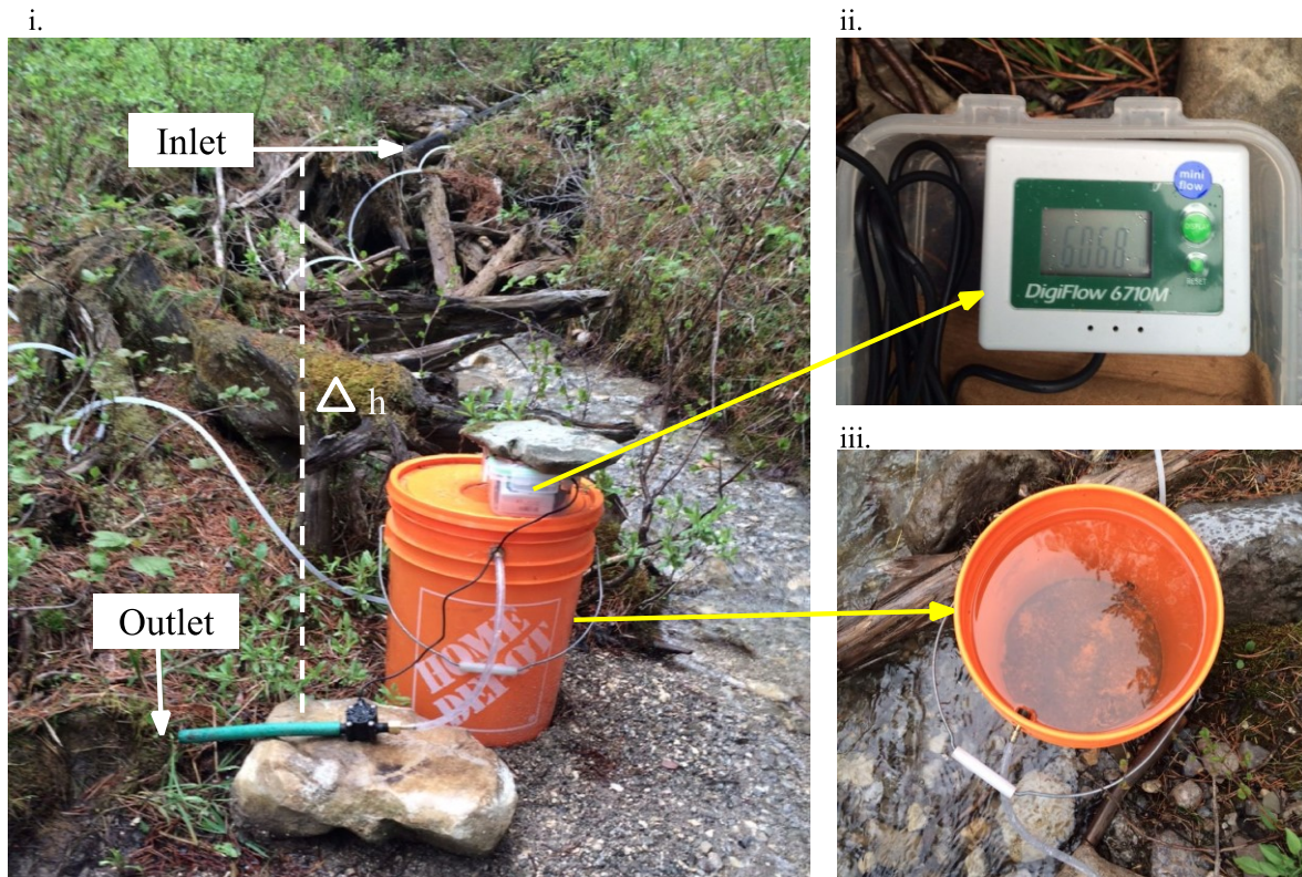
Figure 2-4. The ‘siphonator’ sampling device used to measure continuous wash load concentration (mg/L) up and downstream of road-stream crossing in areas of i) sufficient hydraulic head (meanders, log-steps etc.). Siphonators were deployed for 2-3 weeks, during which ii) total volume (L) was recorded using a DigiFlow volume totalizer (Model 6710M-32, Savant Electronics), while iii) settling basin accumulated sediment.
