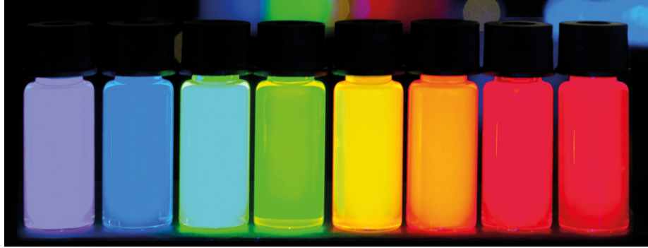
Figure 1.1: Different size colloidal QDs excited by ultraviolet light showing a wide range of colours [1].
