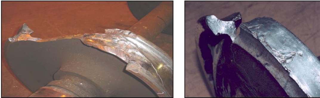
Figure 5-9. Examples of wheel related failures. (Source: TSB Railway Investigation Reports R04T0008 and R04Q0047)
