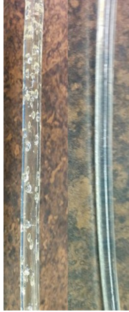
Figure 2-4 Filament without material preprocessing (left)/ Filament with material preprocessing (right)
