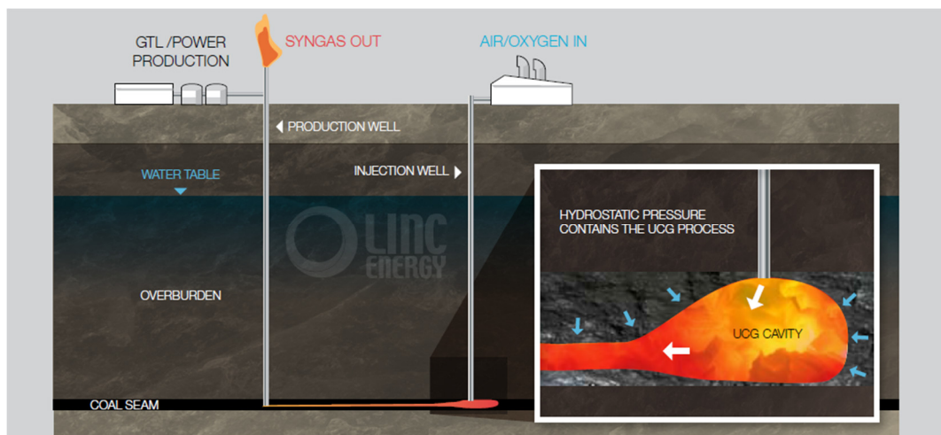
Figure 1 UCG Process and its cavity-Picture from linc energy (3)
