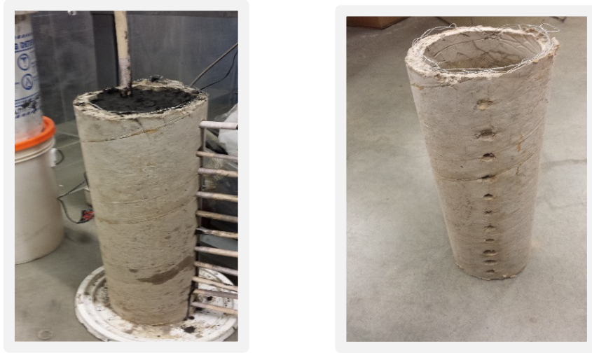
Figure 8 Sample preparation for UCG experiment
