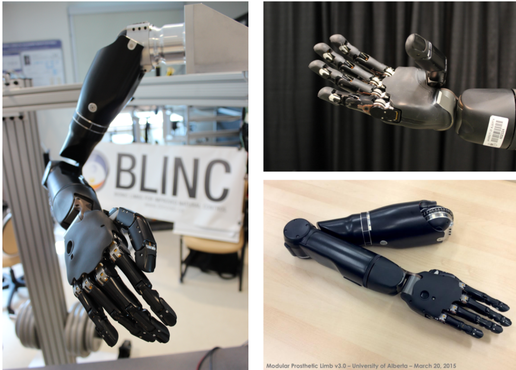
Figure 2.1: The Modular Prosthetic Limb (MPL). It is arguably the most advanced prosthetic arm till date. It has 26 DOF, 17 DOC, and 100+ sensory percepts. The MPL can effect almost all the movements of a biological arm. The MPL therefore promises to provide patients with improved, dexterous control of a prosthetic arm and hand, including a sense of touch.
