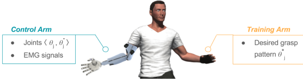
Figure 4.2: We obtain control signals and state information from the control arm. The training arm provides reward signals for the RL agent.
