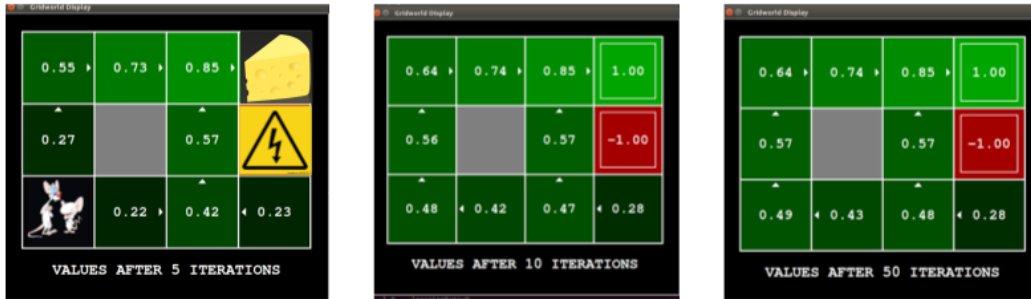
Figure 2.4: This figure shows the learned values over multiple iterations using Temporal Difference (TD) learning without eligibility traces in this grid world. The grid world GUI was adapted from the Berkeley Pacman Project.
