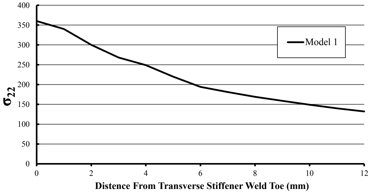
Figure A.C. 1: Vertical stress distribution for Model 1(Run 1) a) in web gap detail, b) along the vertical path at web gap
