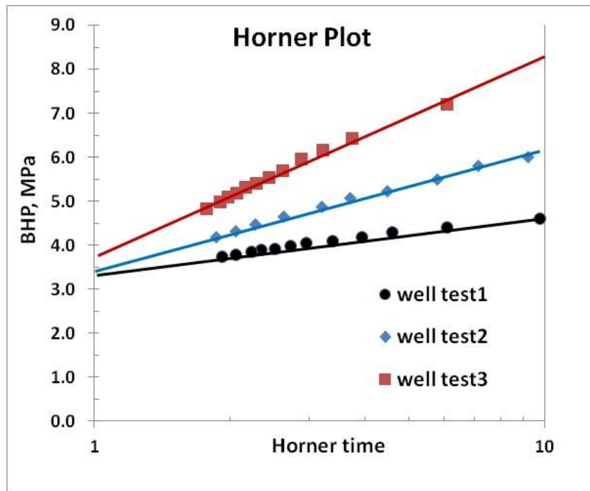
Fig. 5-7: Horner plot of the three well tests
